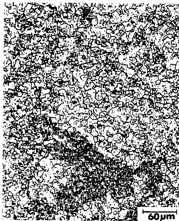
FIGURE 3. Microstructure of UO 2 Pellet Made from Powder Lot Th-D-25, 96.9% TD.
