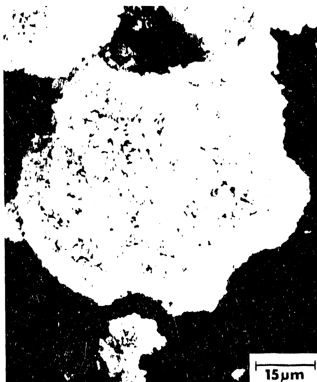
FIGURE 11. Scanning Electron Micrographs (SEM) of Powder Lot Th-D-5 After Calcination and Reduction (Screening Test 600°C, 4 h, 50% H 2 -Ar).
