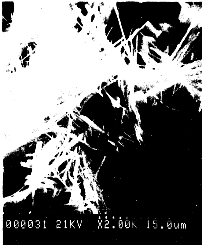
Figure 4-15. SEM micrograph of precipitate on cube surface.
