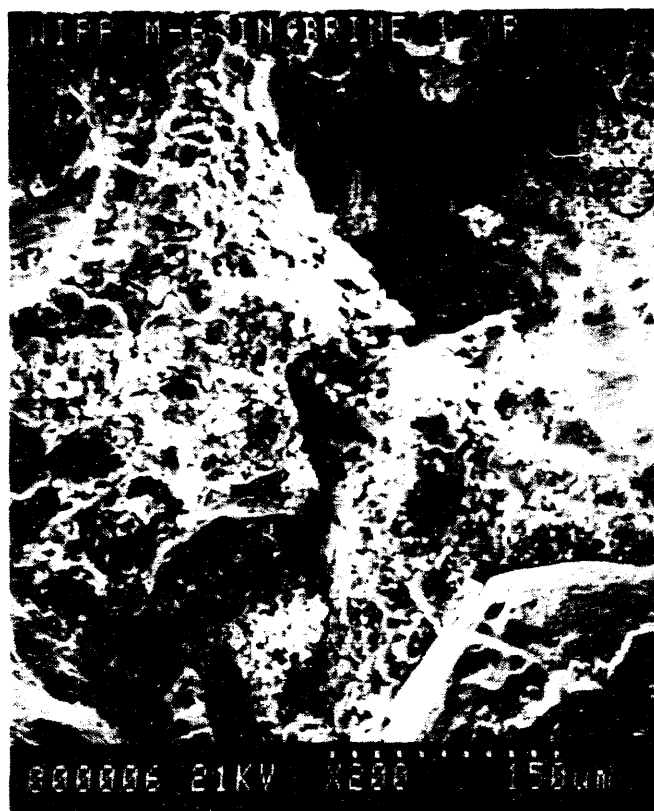
Figure 4-16. SEM micrograph of deteriorated mortar from near edge of M-6 after 1 yr in brine.
