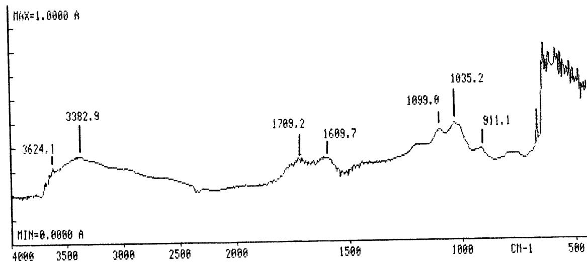
**Figure 6:** DRIFT spectrum of MV bituminous C (PSOC-1527) coal oxidized with air at 230° C for 24 hours
