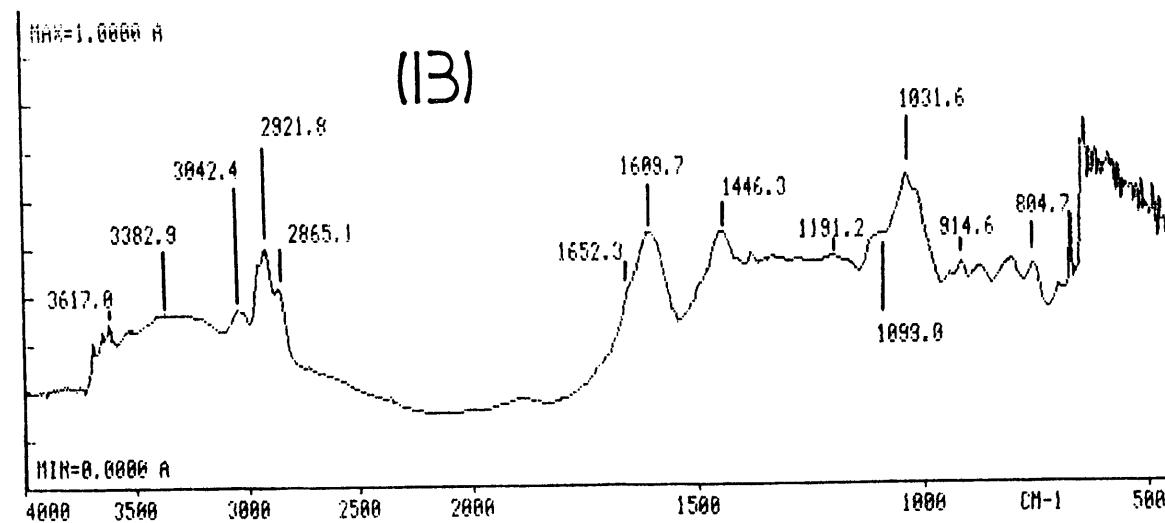
Figure 4: DRIFT spectra of MV bituminous C (PSOC-1527) coal; (A): as-received; (B): oxidized with 1.0 M HNO<sub>3</sub> for 5 hours at room temperature
