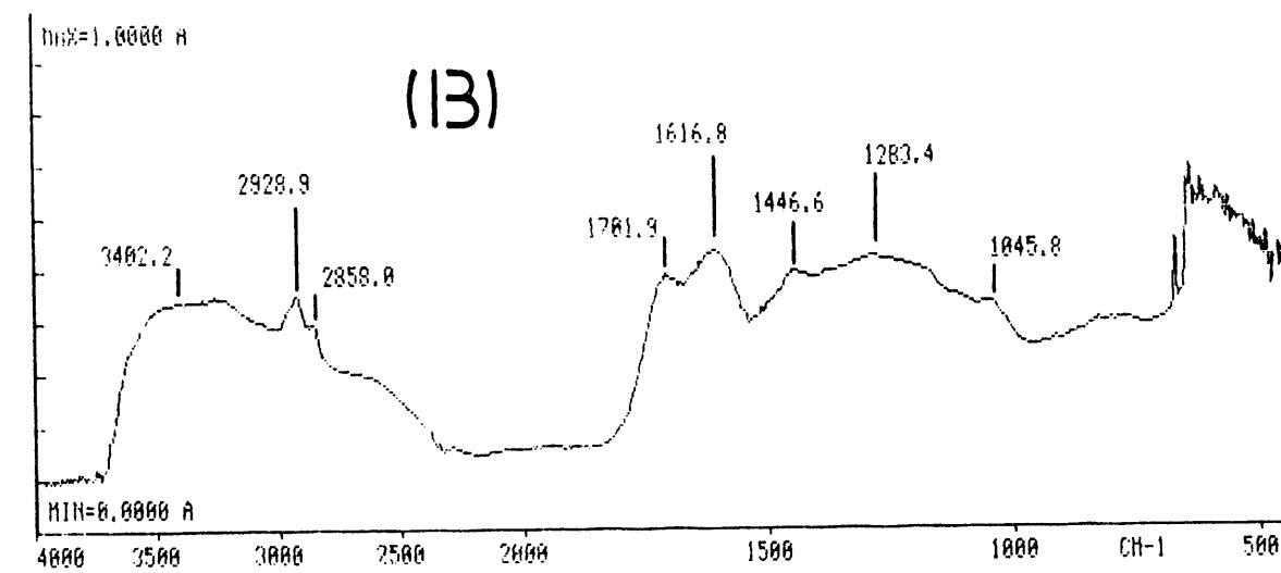
**Figure 1:** DRIFT spectra of sub-bituminous C (PSOC-1+42) coal; (A): as-received; (B): oxidized with 1.0 M  $\text{HNO}_3$  for 5 hours at room temperature
