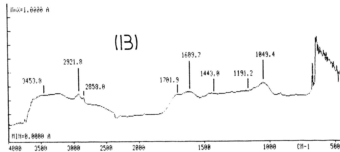
**Figure 3:** DRIFT spectra of HVA bituminous C (PSOC-1481) coal; (A): as-received; (B): oxidized with 1.0 M  $\text{HNO}_3$  for 5 hours at room temperature
