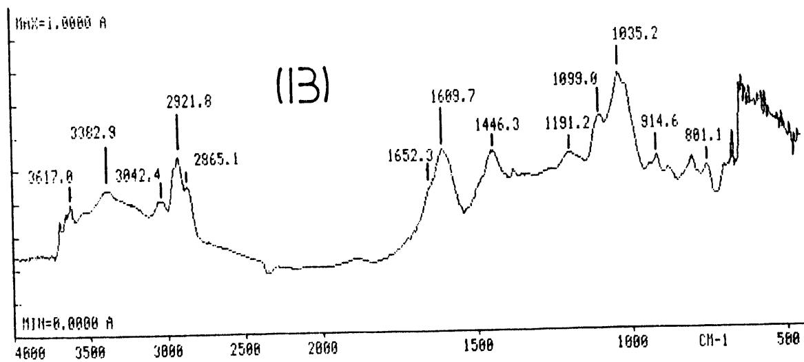
**Figure 5:** DRIFT spectra of MV bituminous C (PSOC-1527) coal; (A): oxidized with  $\text{H}_2\text{O}_2$ ; (B): oxidized with 0.05 M  $\text{Fe}_2(\text{SO}_4)_3$  for 5 hours at room temperature
