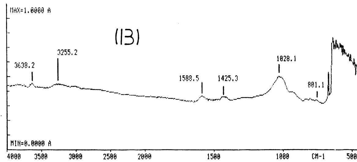
**Figure 7:** DRIFT spectra of anthracite (PSOC-1461) coal; (A): as-received; (B): oxidized with 1.0 M  $\text{HNO}_3$  for 5 hours at room temperature
