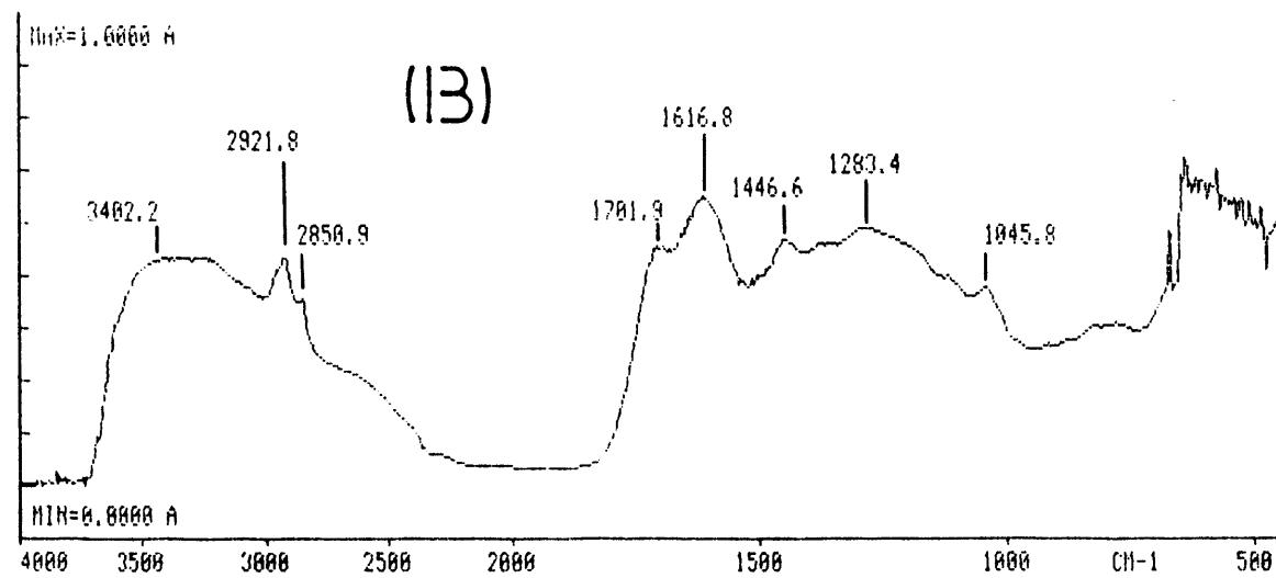
**Figure 2:** DRIFT spectra of sub-bituminous C (PSOC-1442) coal; (A): oxidized with  $\text{H}_2\text{O}_2$ ; (B): oxidized with 0.05 M  $\text{Fe}_2(\text{SO}_4)_3$  for 5 hours at room temperature
