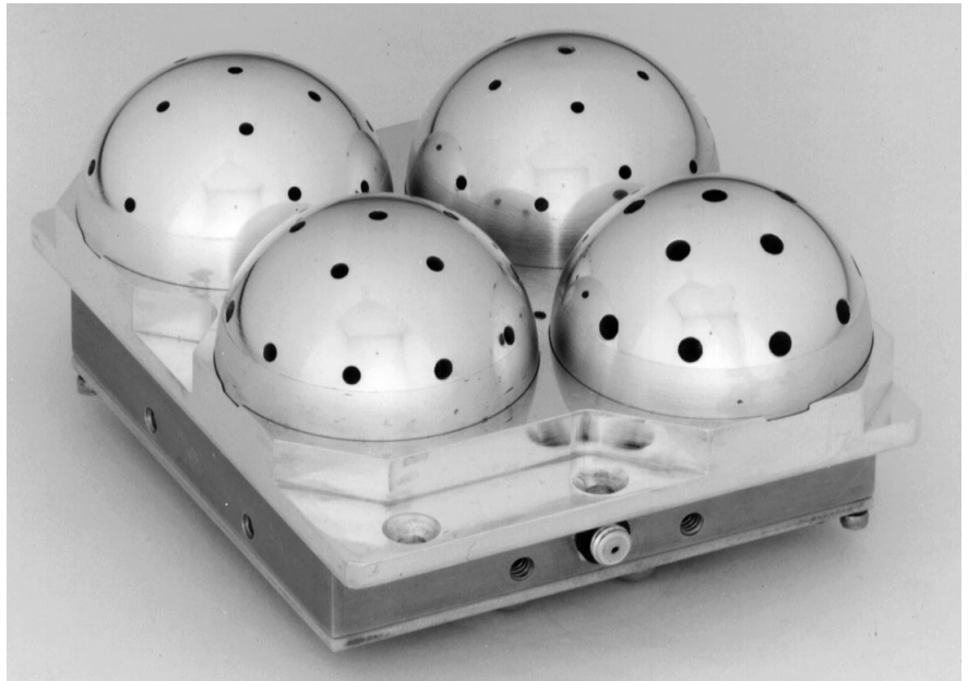
■ Figure 2. Four domes of the background instrument. Holes surrounded by thick material allow the flux to be sampled over a hemisphere at a counting rate that can be conveniently handled by the electronics. A hemispherical filter inside each dome defines an energy threshold for the particles entering the holes. Thus, four energy channels can be defined for the dose measured by the instrument.
