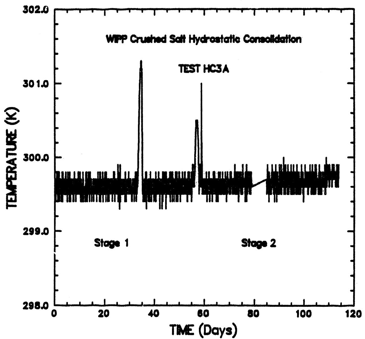
Figure I-3. Temperature-versus-time for Test HC3A.
