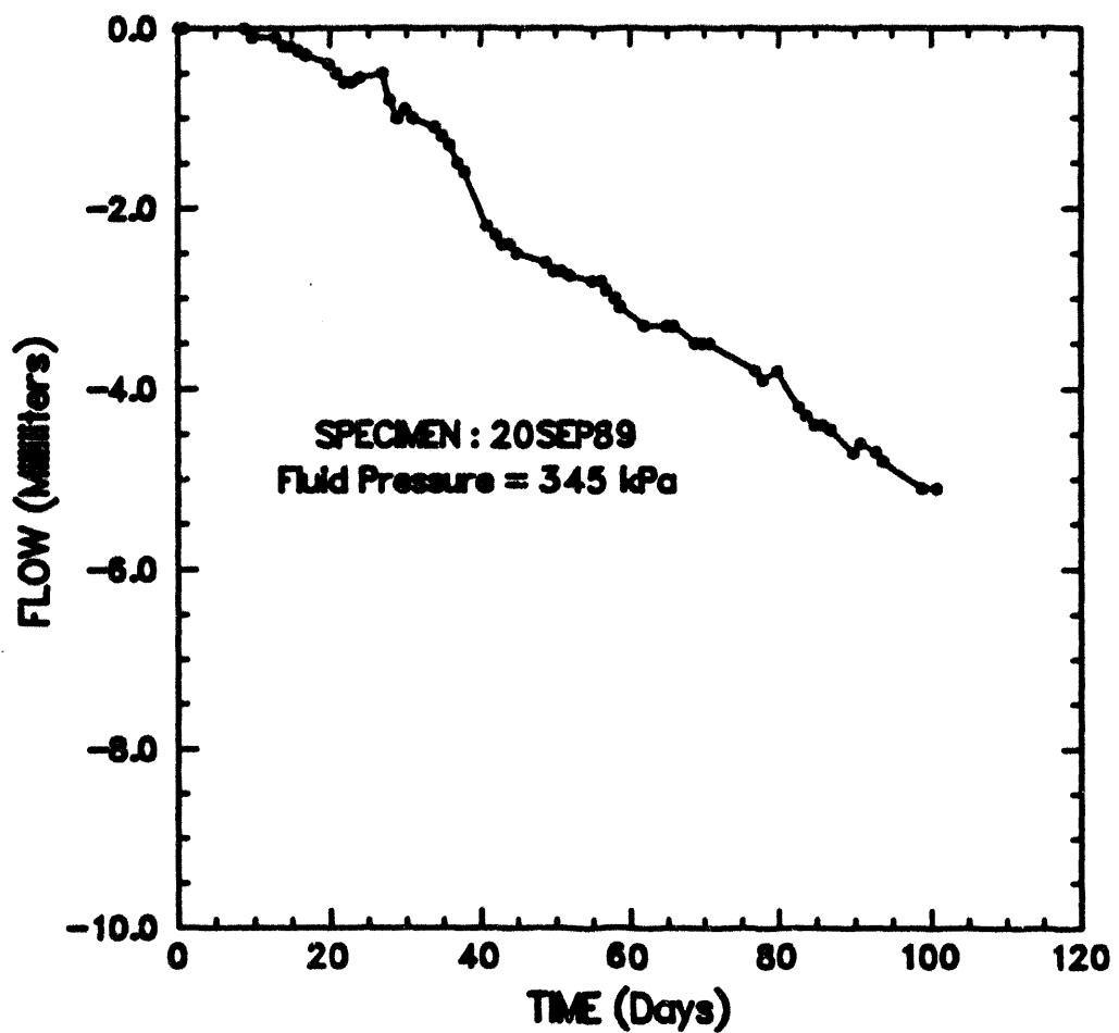
Figure 5-4. Brine volume-versus-time for Sandia-furnished Specimen 20SEP89.
