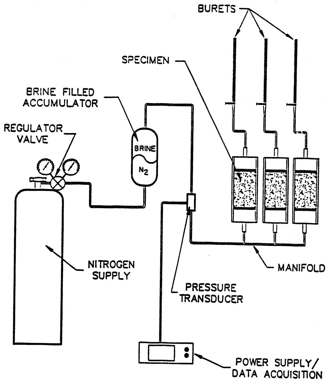
Figure 3-2. Schematic of brine permeability test apparatus used for Sandia-furnished specimens.
