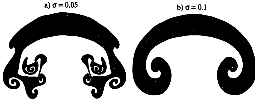
Figure 14 Bubble shapes at t^* = 3 for core radii of a) 0.05 and b) 0.1, with adaption criteria of 2.5. The solution using the smaller core size has many more small-scale features than the solution using the larger core size. Similar findings are also reported by Rottman and Stansby [20].
