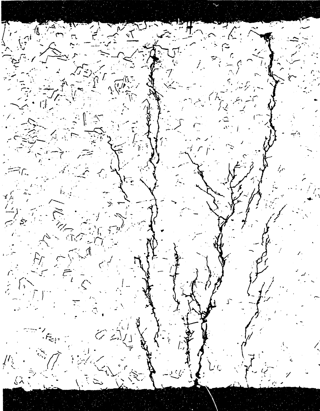
EXHIBIT NO. 14 105-H REAR FACE - PHOTOMICROGRAPH OF STRESS CORROSION CRACK IN CONNECTOR
