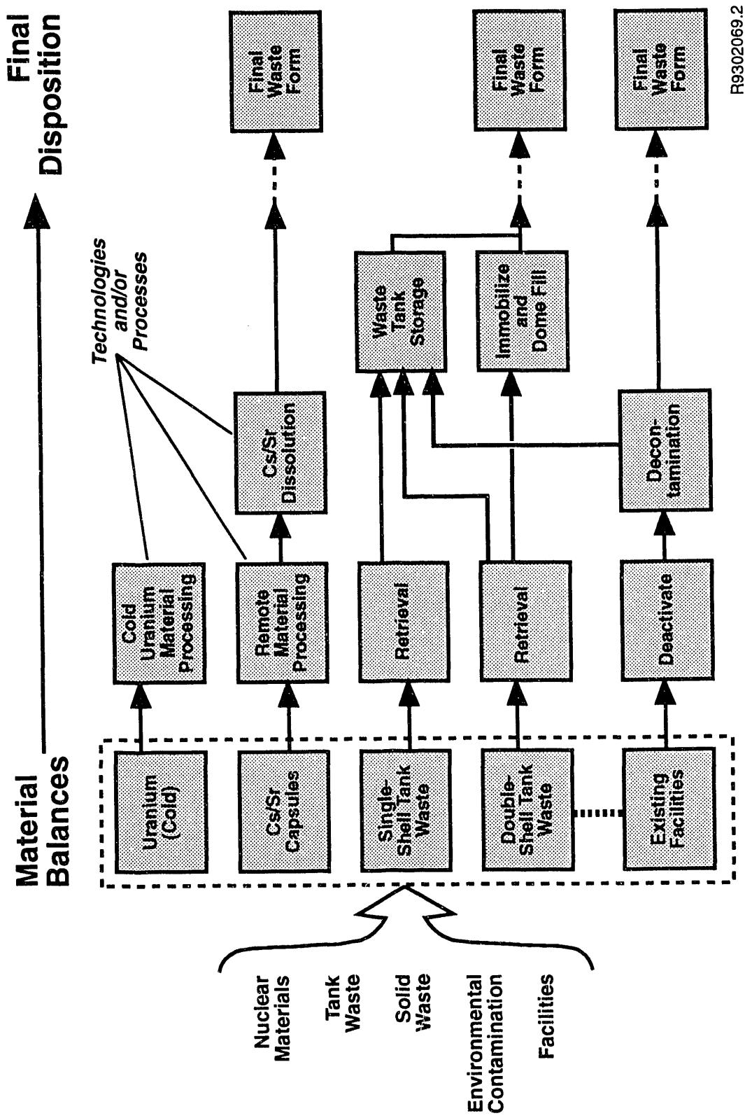
Fig. 1 Systems Analysis Model of Cleanup Process
