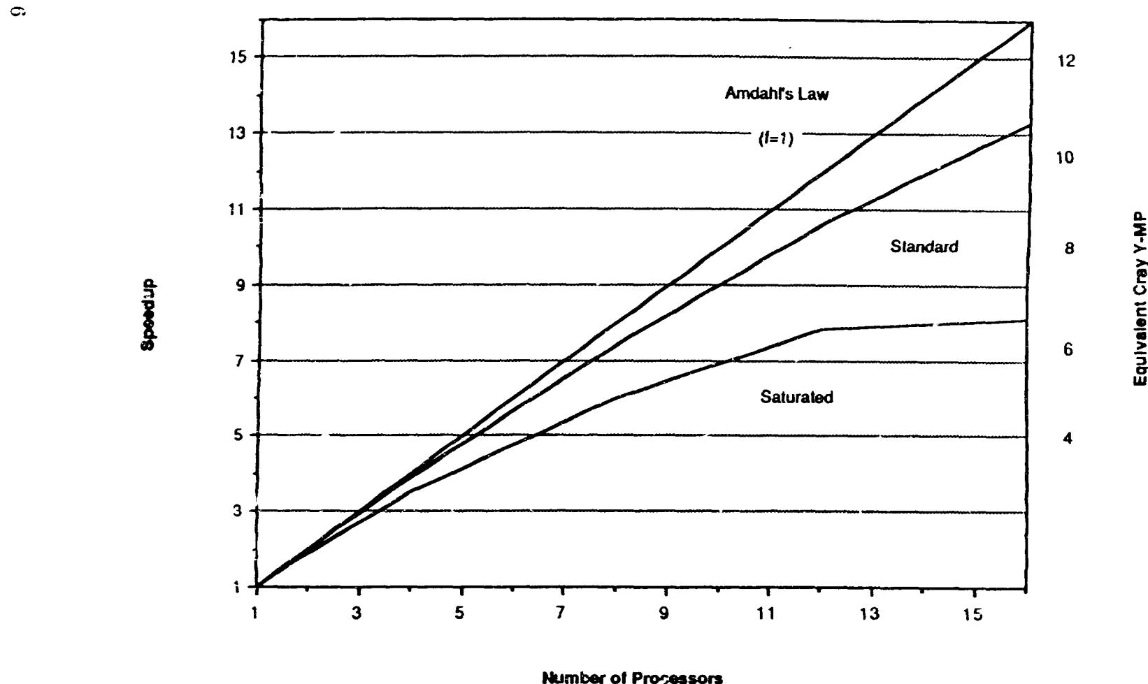
Fig. 1. MCNP Speedup on the LANL 16 Processor IBM RS/6000 Cluster.
