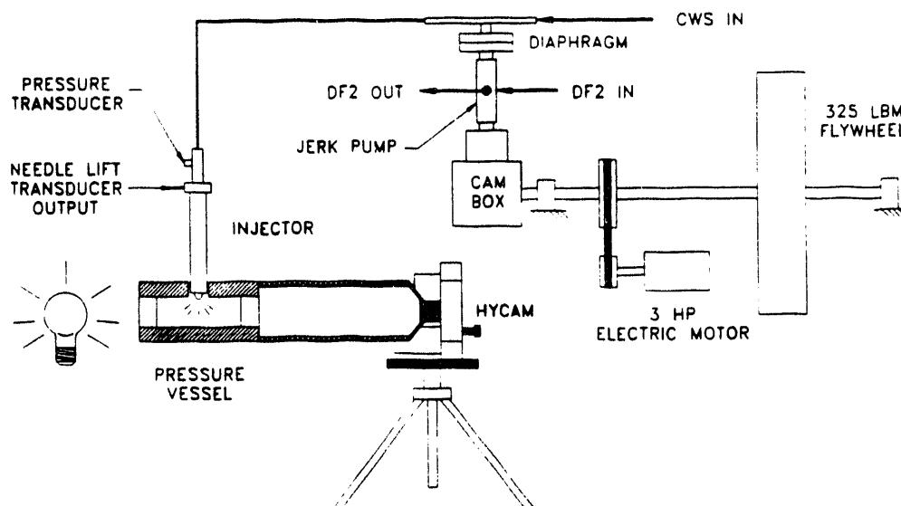
Figure 1. Schematic of the experimental facility.
