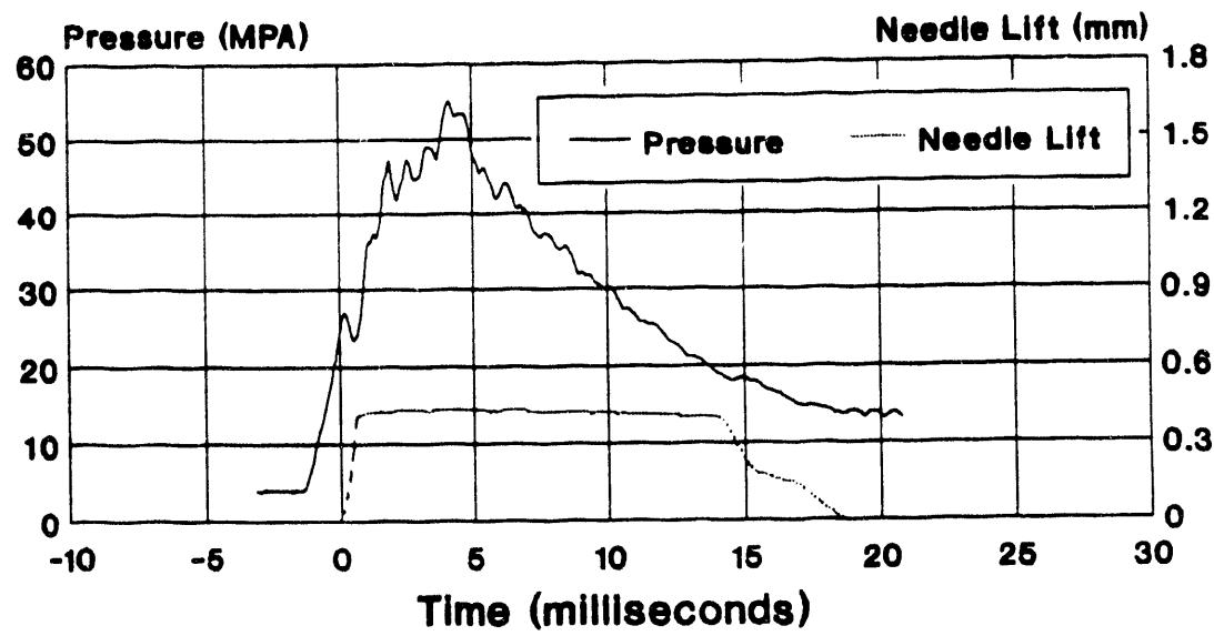
Figure 3. Instantaneous fuel line pressure and needle lift as a function of time.
