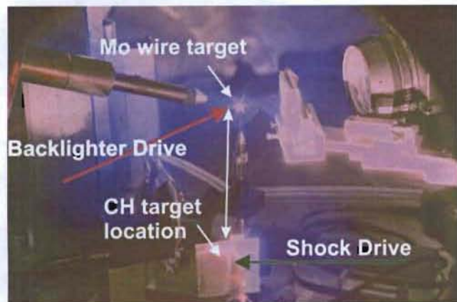
Figure 1 As shot target geometry showing backlighter position and polystyrene (CH) target location. The incident laser for the backlighter allowed the wire to be place tip-on to the target. The nanosecond shock drive is from the right. Backlighter and target are 25-cm apart while the detector is located 120-cm from the target.
