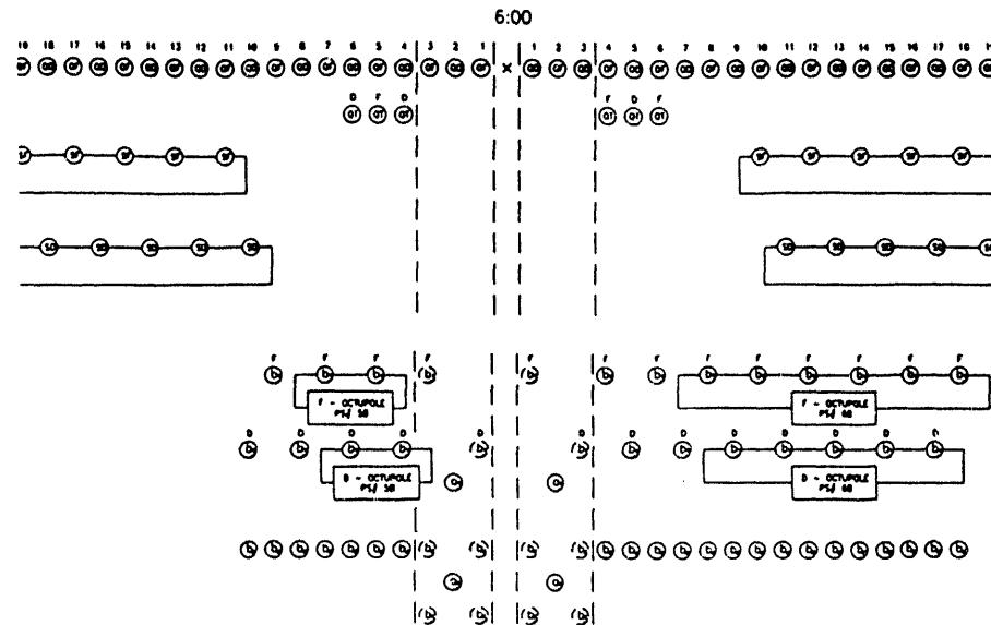
Figure 1. Octupole and decapole correction elements inside the interaction region.
