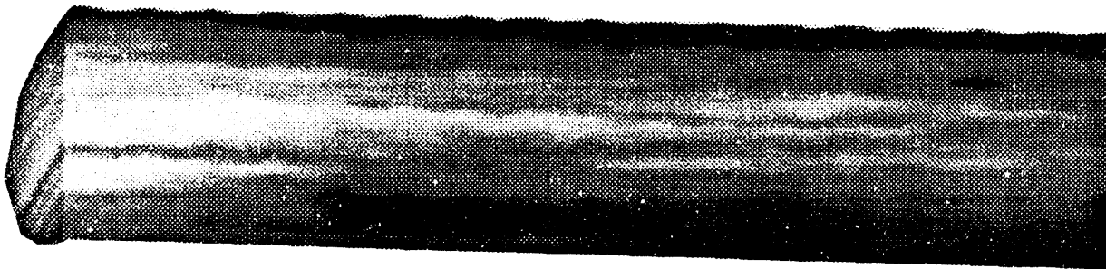
FIGURE 37. - CT composite image of coreflood CT-CF 2 showing oil distribution after the polymer flood. Fluids channelled through the center of the core leaving significant amounts of oil in the core in agreement with oil recovery measurements.
