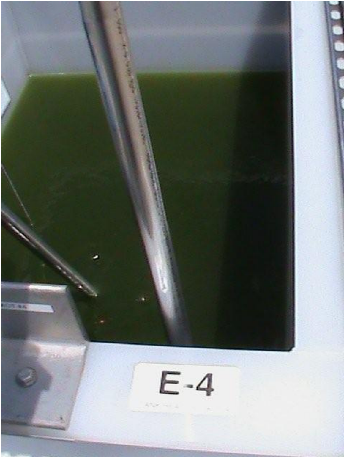
Figure 20 – Hopewell Algal Tank with high turbid mixed algal/bacterial growth
