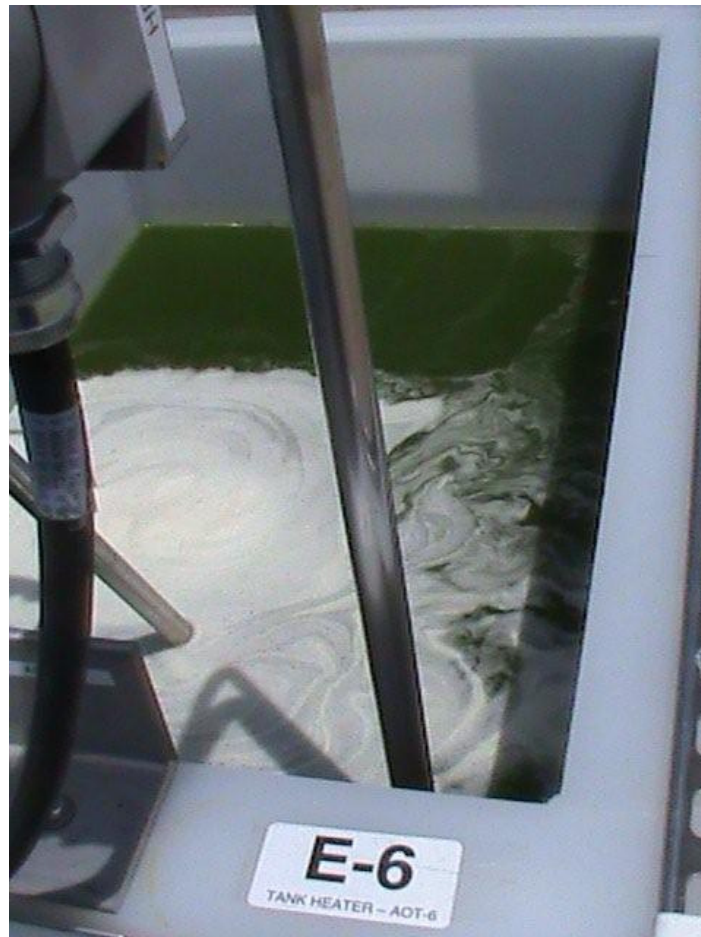
Figure 15 – CO 2 Sparging of Algal Pilot
