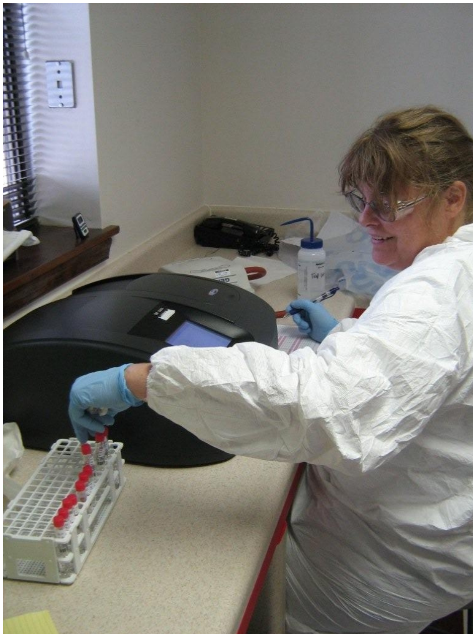
Figure 12 – Measurement of Nutrients in Hopewell Wastewater with HACH Spectrometer
