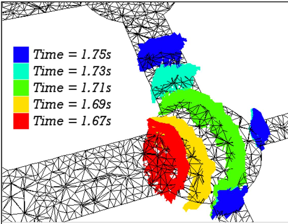
Air-water interface entering a lattice-cell pore during a simulation.
