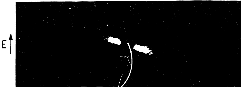
Figure 4. The scattering pattern of a sheared fluid is rotated with respect to that of a quiescent fluid (Figure 1). In this case, the shear rate \dot{\gamma} = 1.04\text{s}^{-1} . There is also a much stronger intensity near the origin, where the scattering wave-vector is small, than for the quiescent fluid.
