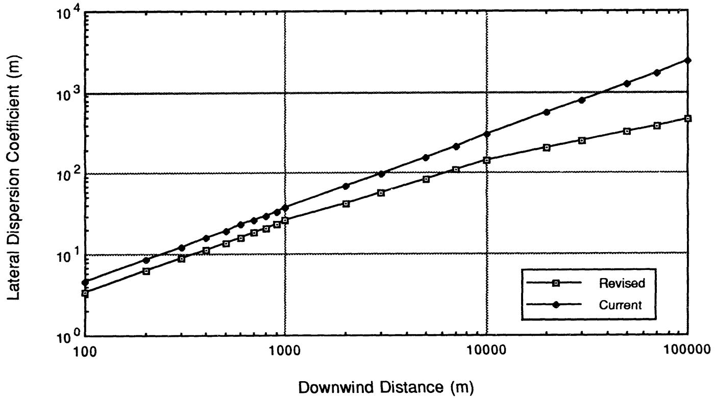
Figure 8. Lateral Dispersion Coefficient Comparison for Stability F
