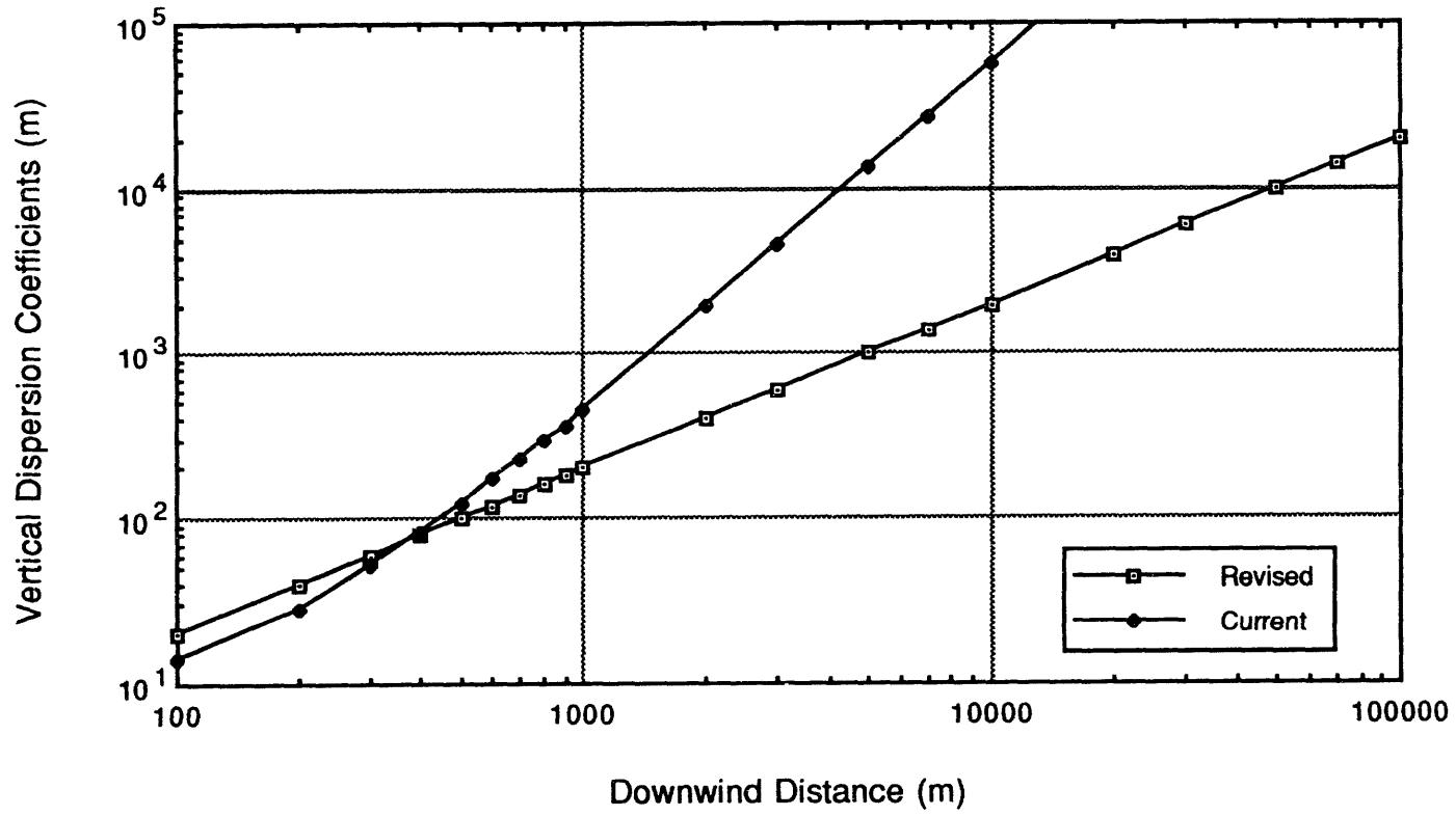
Figure 10. Vertical Dispersion Coefficient Comparison for Stability A
