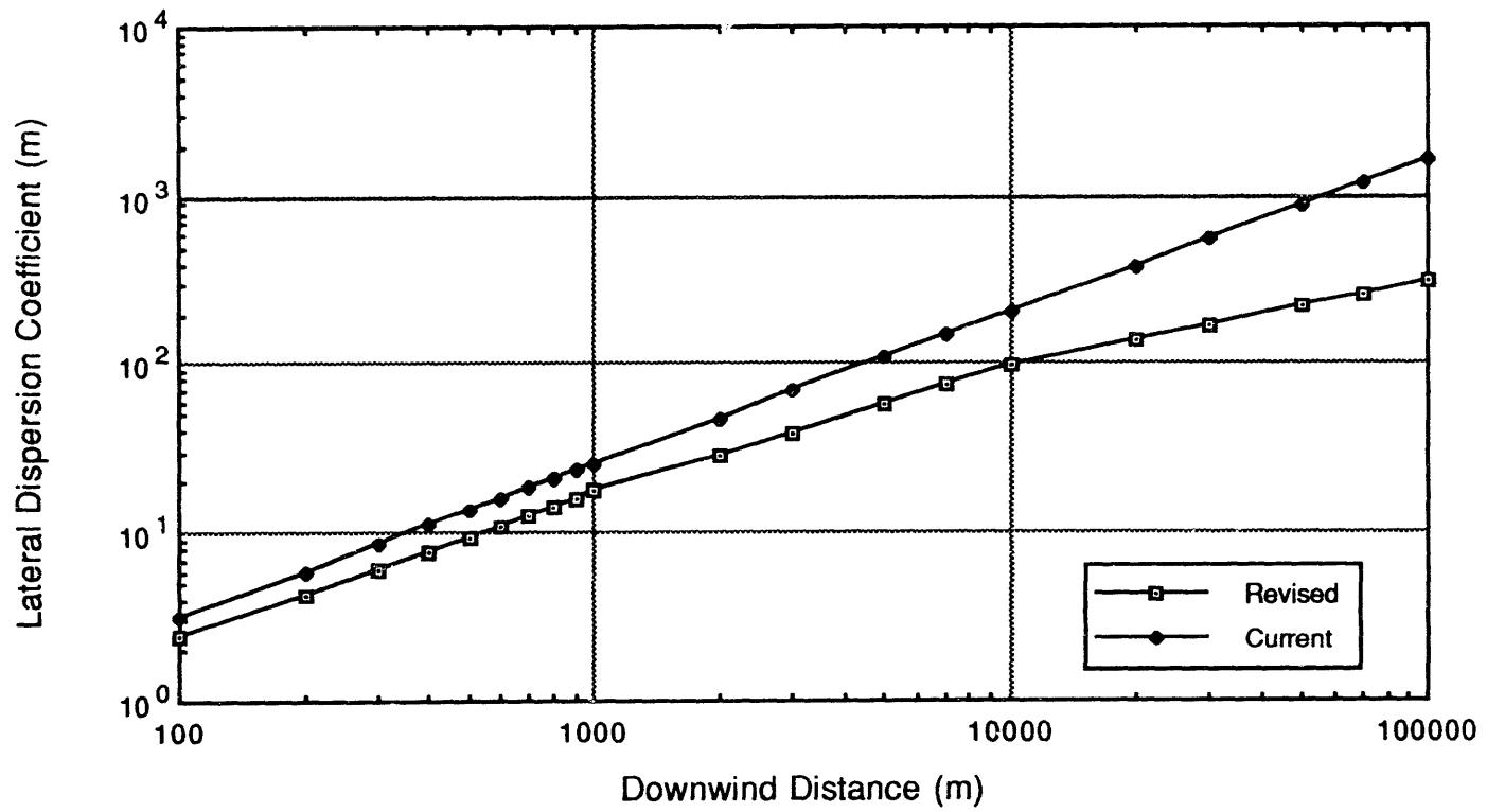
Figure 9. Lateral Dispersion Coefficient Comparison for Stability G
