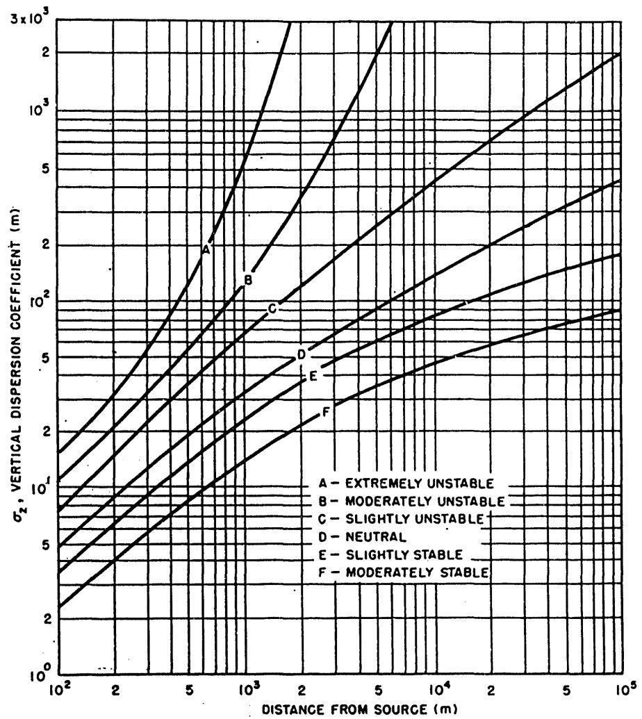
Figure 2. Vertical Diffusion Coefficients from NRC 1.145
