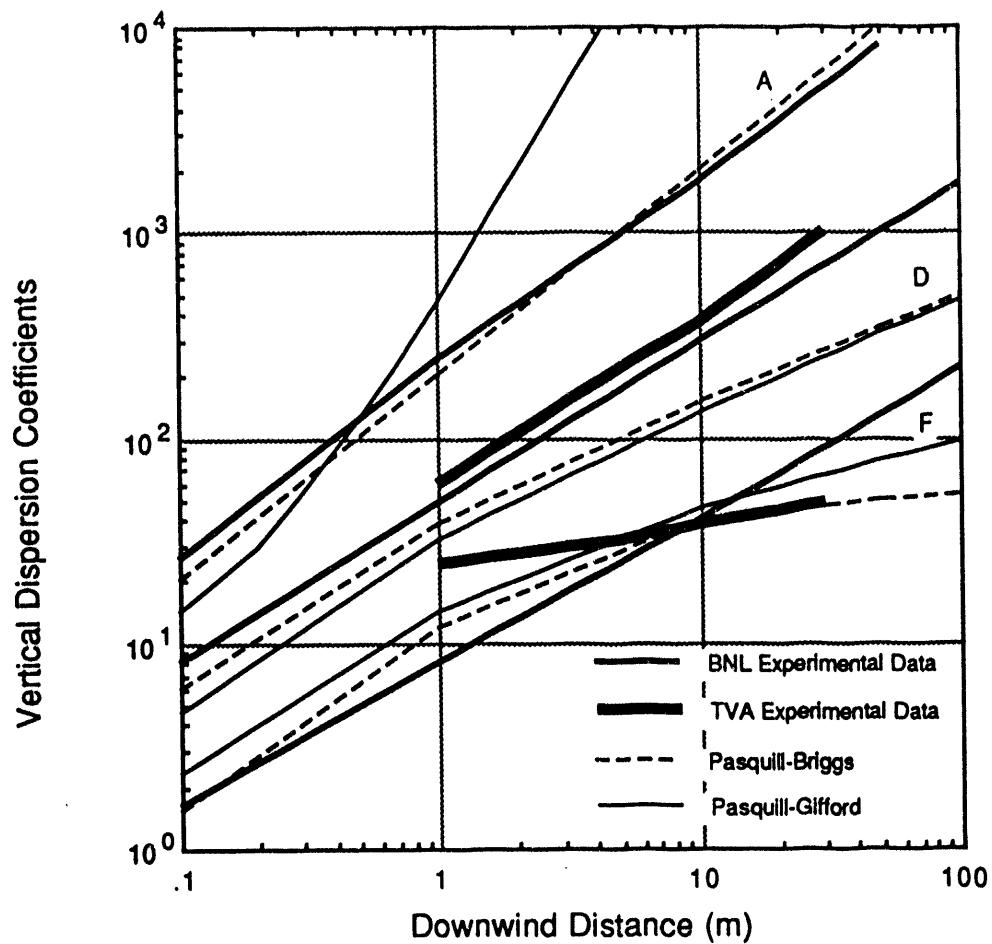
Figure 19. Vertical Dispersion Coefficient Comparison with Experimental Data
