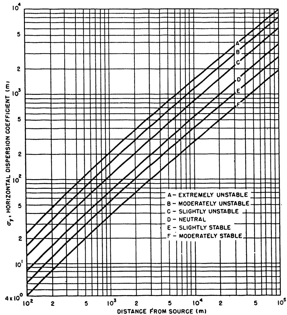
Figure 1. Lateral Diffusion Coefficients from NRC 1.145
