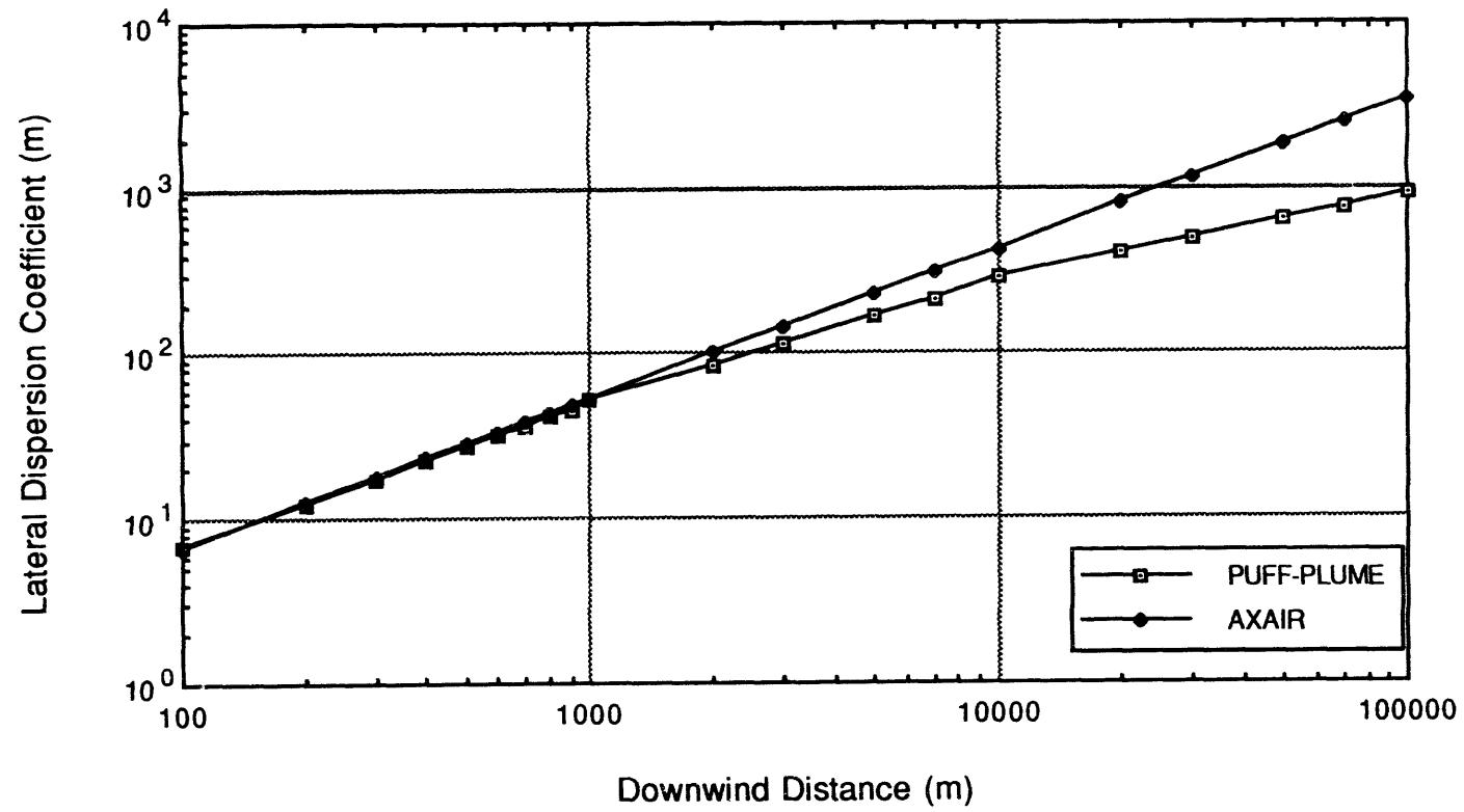
Figure 7. Lateral Dispersion Coefficient Comparison for Stability E
