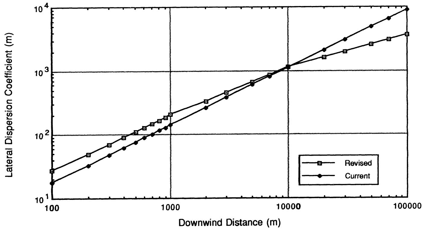
Figure 4. Lateral Dispersion Coefficient Comparison for Stability Class B
