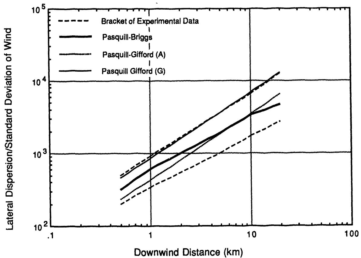
Figure 20. Horizontal Dispersion Coefficient Comparison w/ Experimental Data
