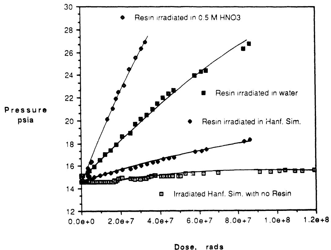
Figure 4. Pressures produced from irradiation of 13.5 grams of resin in 27 ml of 0.5 M HNO<sub>3</sub>, water, and Hanford simulant in 45 ml stainless steel sealed vessels. The lower curve is from pressures produced from irradiation of 31 ml of Hanford simulant with no resin present.
