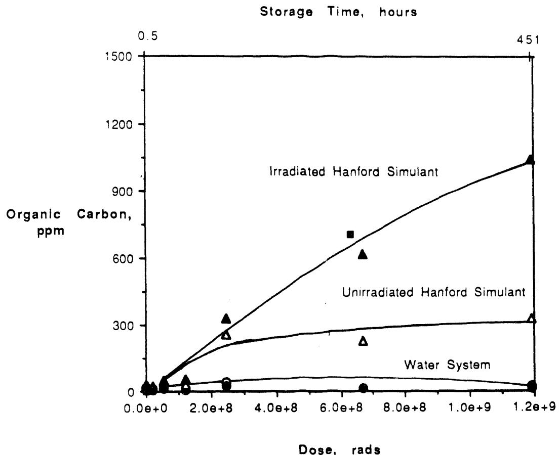
Figure 1. Organic carbon leached by 60 ml ASTM water rinses of samples of Na/K form resin that had been irradiated or stored in Hanford Simulant or Water. Closed symbols are for the irradiated system and open symbols for unirradiated. All results are for resin samples irradiated or stored in glass, except the result shown by ■, which is the average of duplicate resin samples irradiated in Hanford simulant contained in stainless steel vessels.
