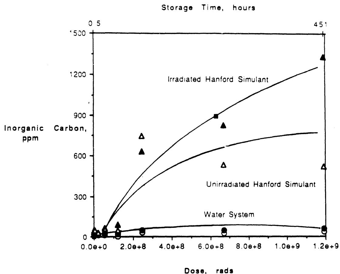
Figure 2. Inorganic carbon leached by 60 ml ASTM water rinses of samples of Na/K form resin that had been irradiated or stored in Hanford Simulant or Water. Closed symbols are for the irradiated system and open symbols for unirradiated. All results are for resin samples irradiated or stored in glass, except the result shown by ■, which is the average of duplicate resin samples irradiated in Hanford simulant contained in stainless steel vessels.
