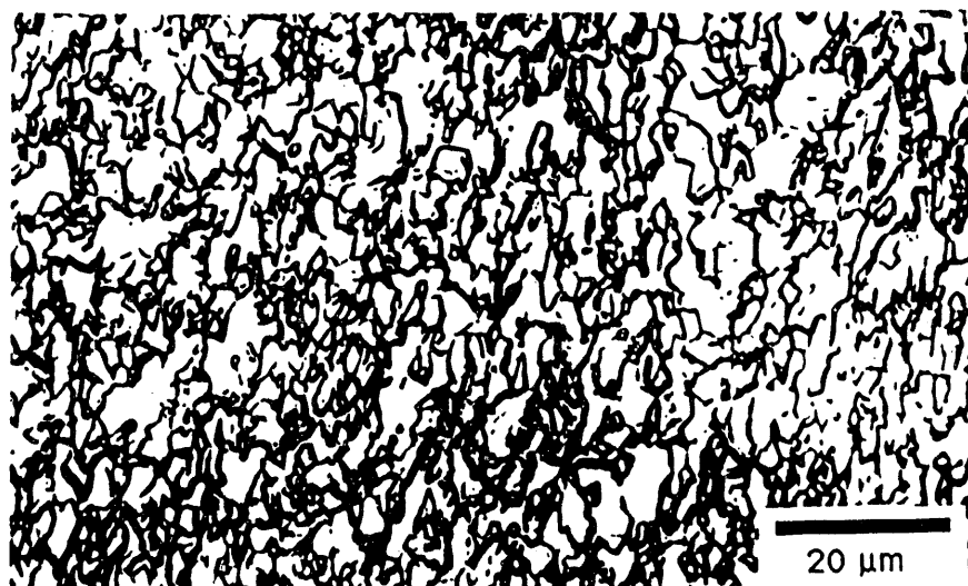
Fig.6 Microstructure of CVD tungsten showing fine grain size.
