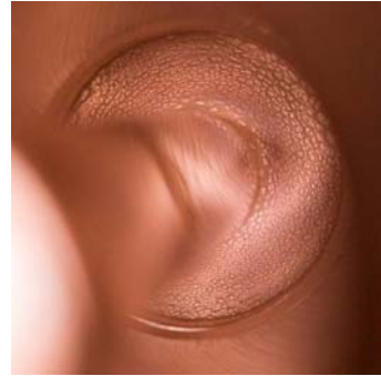
Figure 6: View of ceramic rf window after testing cavity in a magnetic field. A layer of copper was somehow deposited on the ceramic window during the test process.
