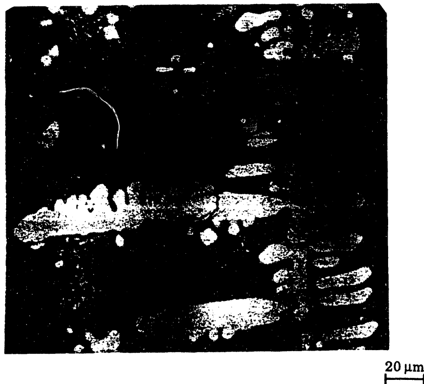
Figure 6. Scanning Electron Micrograph Showing Dendritic Fe 3 Zr Phase in the HT-9 Matrix (backscattered electron image)
