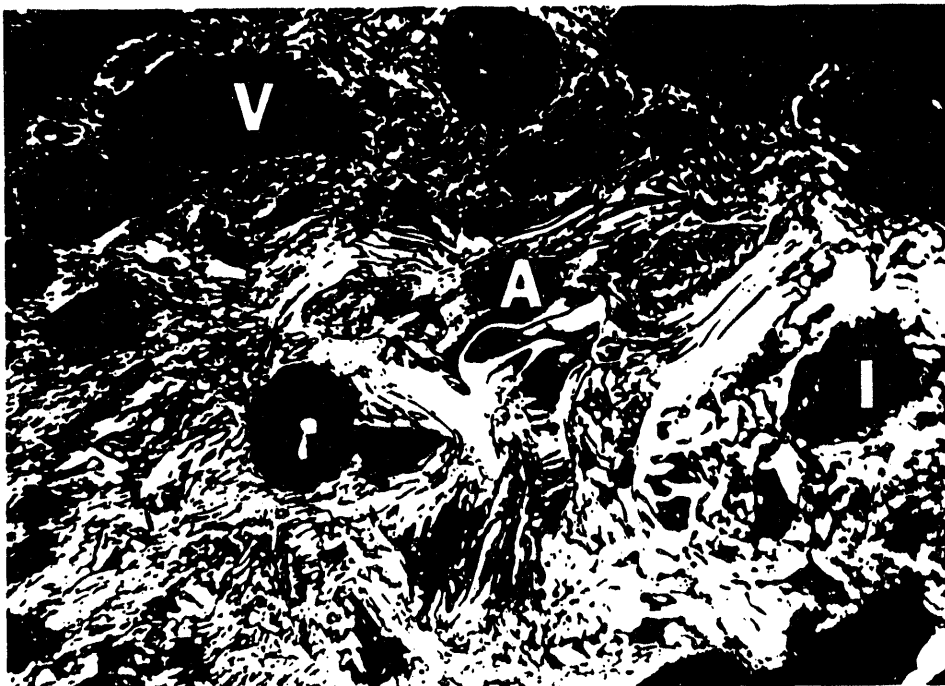
Figure 4. Photomicrographs of Char from Coal Technology Corporation's Twin Screw Carbonizer Showing Char in Polarized Light Where A=Anisotropic Binder Carbon, I=Isotropic Inert Filler Carbon and V=Voids. Reflected Polarized Light with Tint Plant in Oil, X 450.
