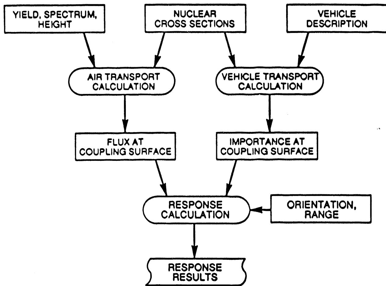
Figure 1. General Structure of a Typical Application of the MASH Code System.
