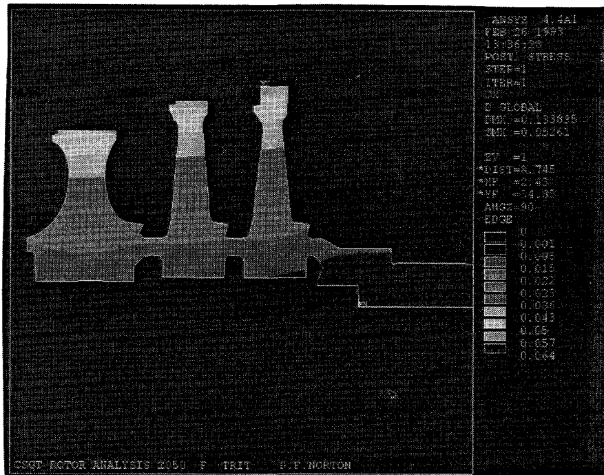
Figure 4-41. Radial CSGT Turbine Disk Displacements at 1121°C (2050°F) TRIT
