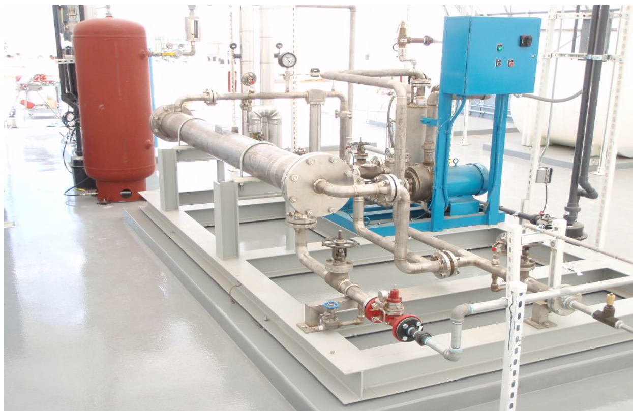
Figure 4-16. MTR CO 2 Capture Membrane Skid
