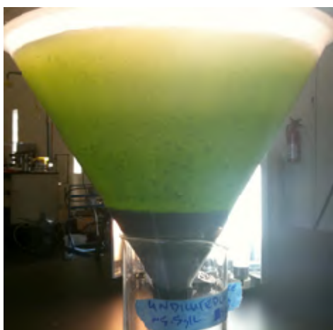
Figure 4-7. Settled Scenedesmus Culture after 5 hours in a Conical Bottom Vessel
