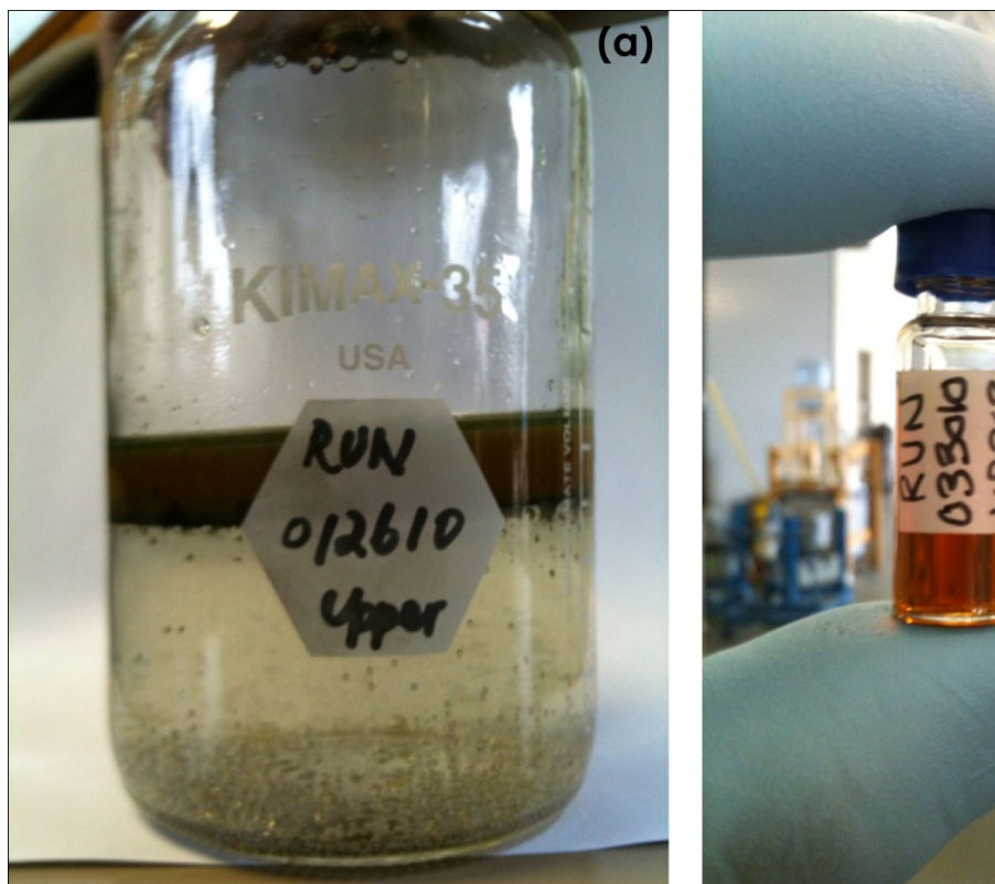
Figure 3-7. (a) Liquid from the Upper Condenser Pot; (b) Comparison of Oil/BTX Samples from Upper and Lower Condenser Pots
