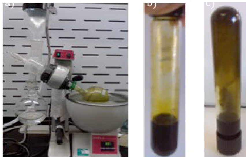
Figure 4-34. a) Rotary Evaporation; b) Lipid Extracts; and c) Flowable Lipid Extracts
