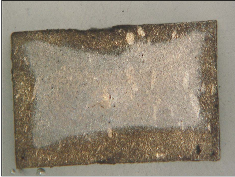
Figure 4-18: Polished cross section of Pellet 4 at 25x magnification demonstrating inner and outer regions.
