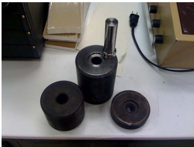
Fig 1. The hot extrusion tooling assembly. From left to right: The top piece which holds the sample canister, the base, the extrusion ram, and the reduction die.
