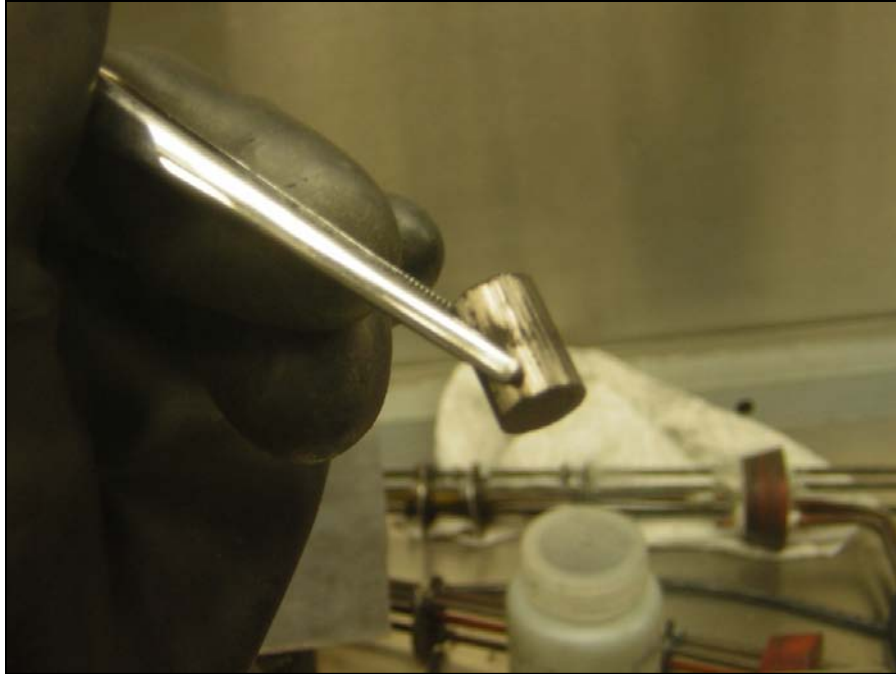
Figure 4-9: Pellet 6 as pressed, before sintering.
