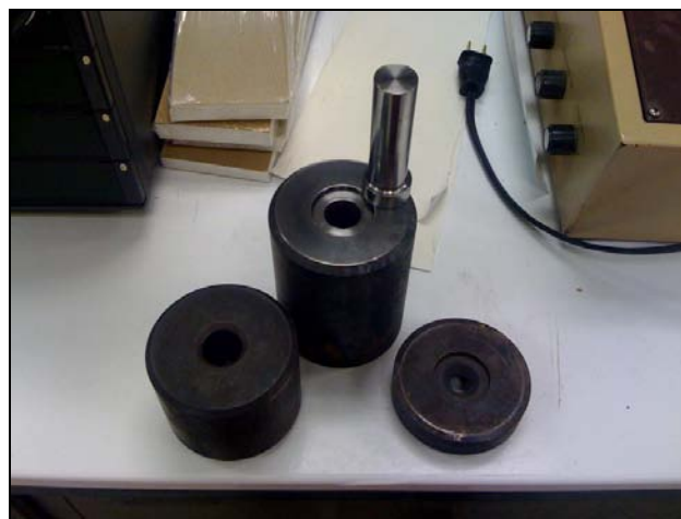
Fig 1. Extrusion tooling assembly. From left to right: The top piece which holds the sample canister, the base, the extrusion ram, and the reduction die.
