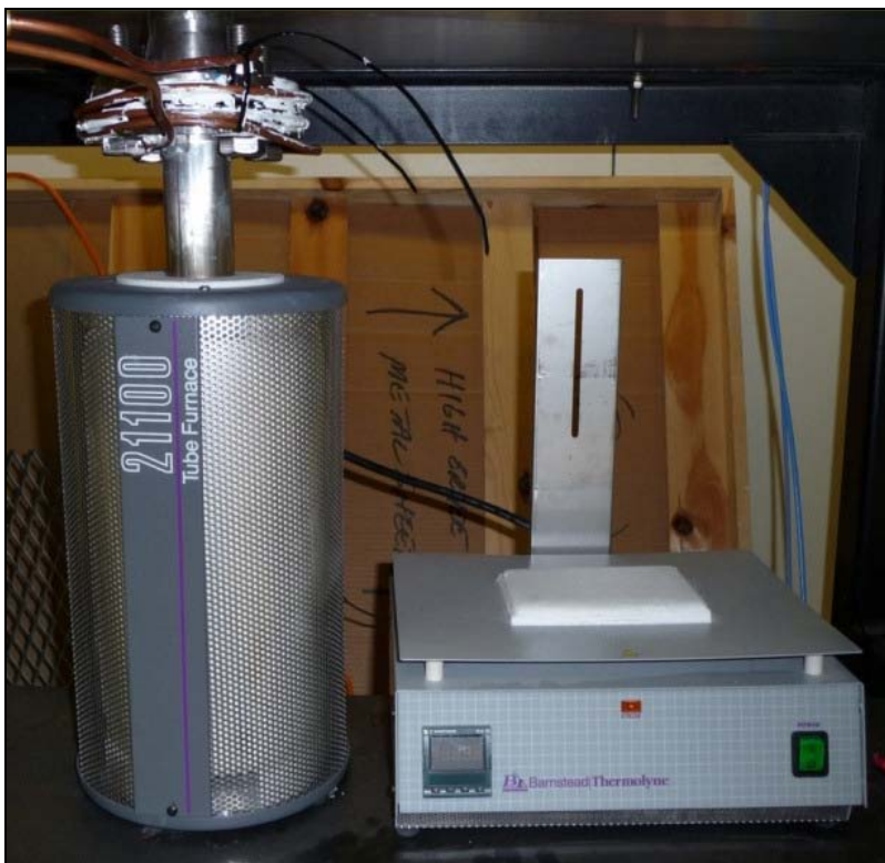
Figure 3-6: Furnace used for hydride/dehydride process.
