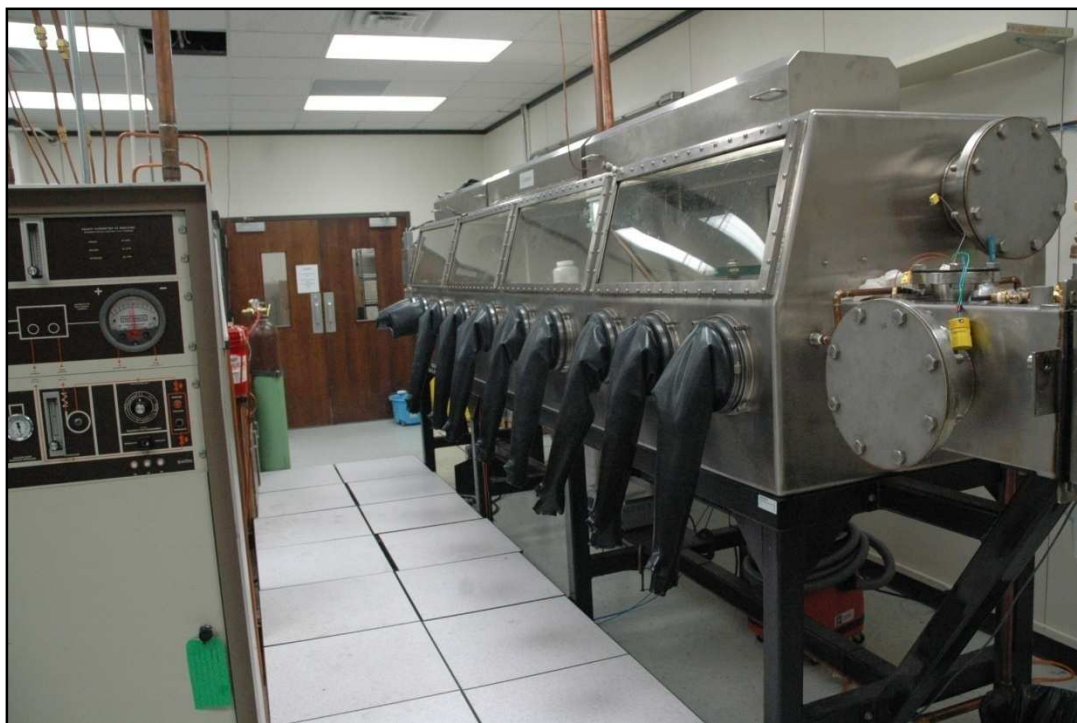
Fig. 3-1 Inert atmosphere glovebox, primary location of the experiments
