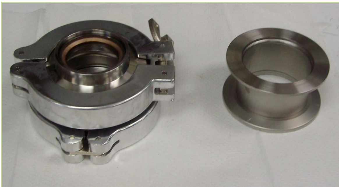
Figure 6. The ACV with an alternate nipple size for viewing larger samples.
