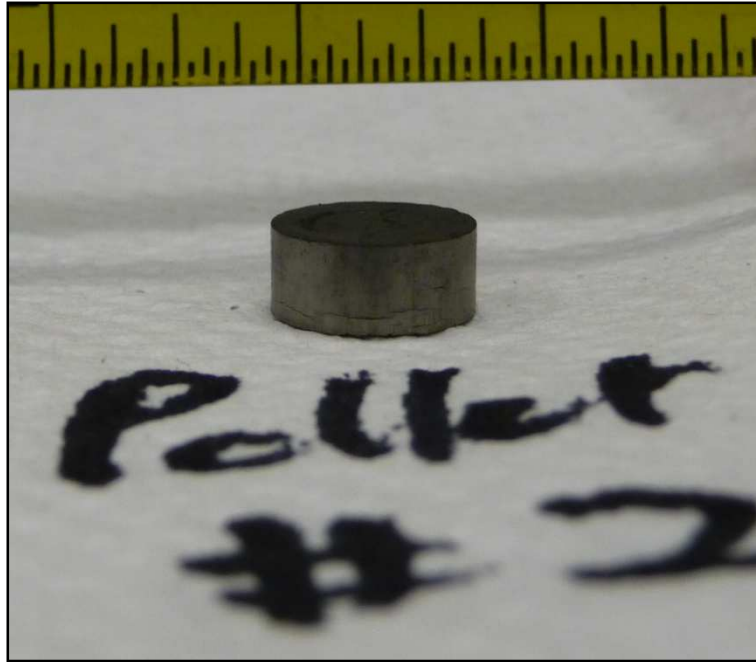
Fig. 4-22 Pellet 2 post sinter
