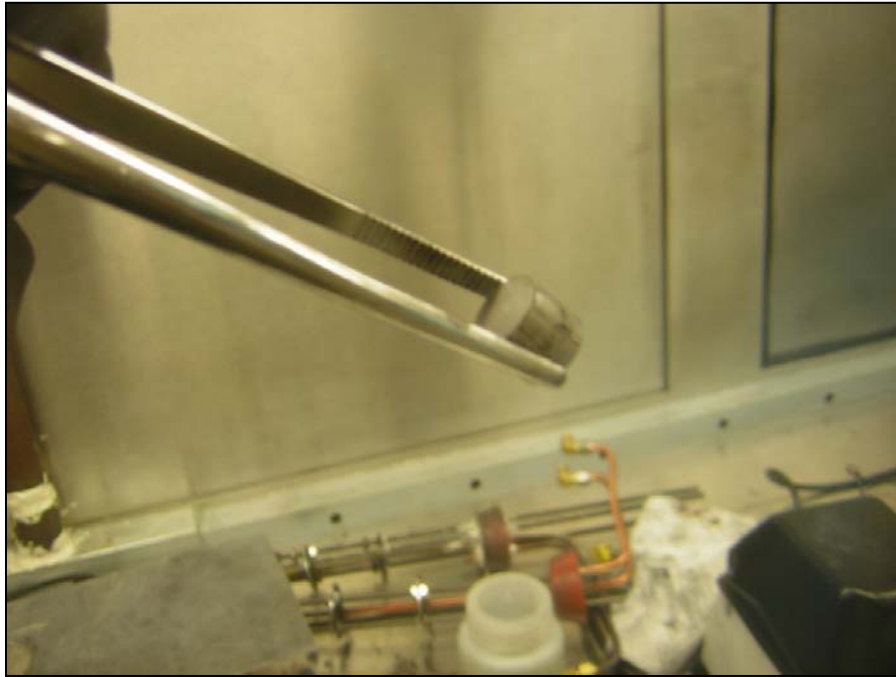
Figure 4-25: Pellet 9 as pressed, before sintering.
