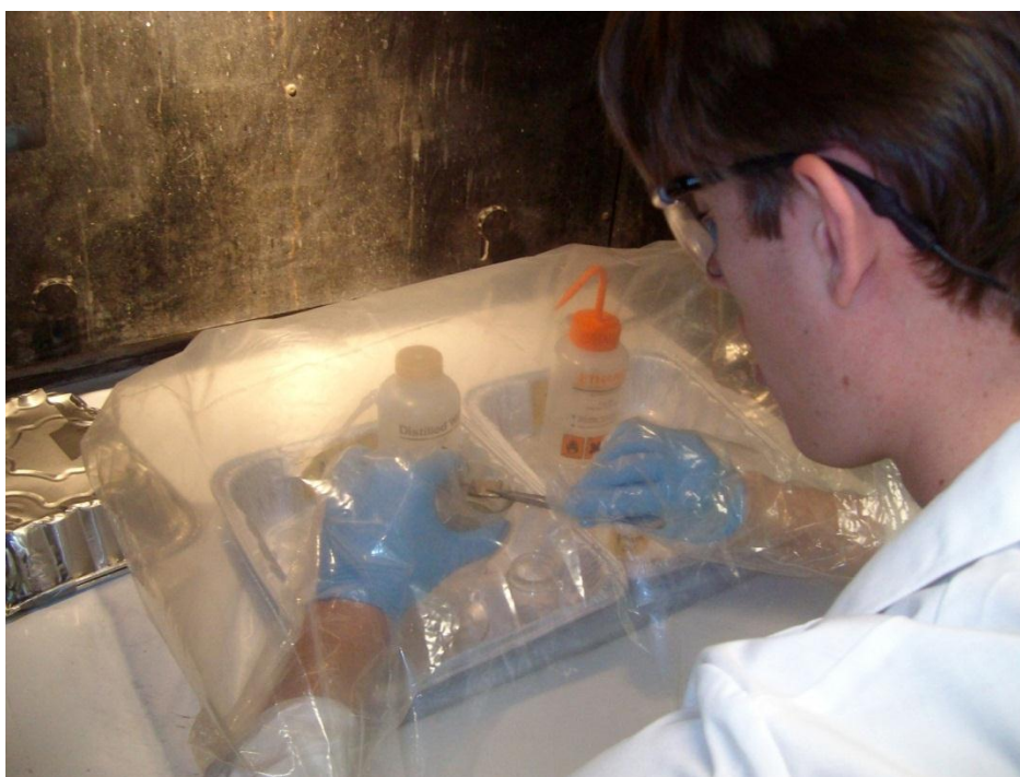
Figure 11. Acid wash station located inside a glovebag under argon atmosphere to reduce sample oxidation.
