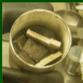
Uranium slugs loaded into Yttria crucible before hydriding
