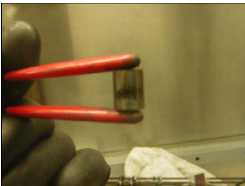
Figure 4-3: Pellet 3 as pressed, before sintering.
