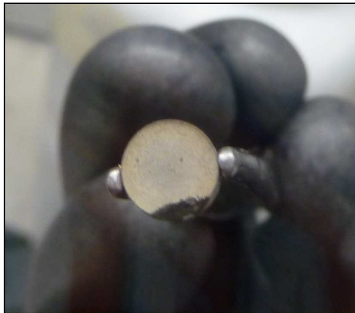
Fig. 4-38 Pellet 10 post experiment, pellet was gold and structurally damaged33
