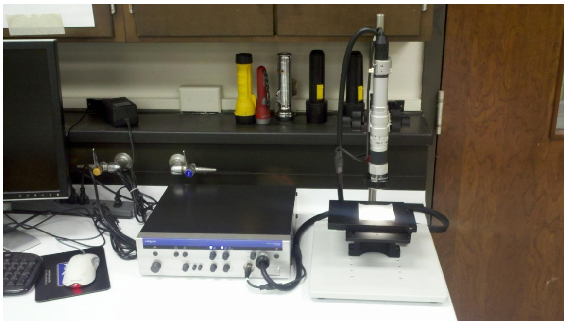
Figure 7. HIROX digital microscope used for powder imaging.
