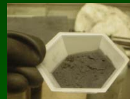
Uranium powder after removal from the reaction vessel
