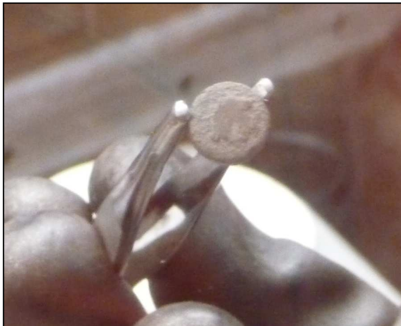
Fig. 4-35 Pellet 9 (DU-10Zr Wt %) post experiment
