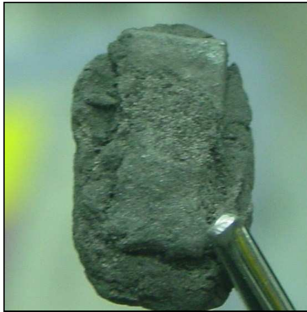
Figure 4-11 Non-hydrated DU visible and surrounded by sintered powder
