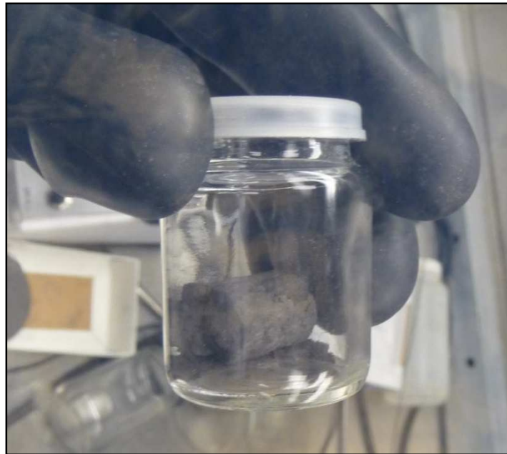
Figure 4-7 Loose and sintered powder produced post experiment
