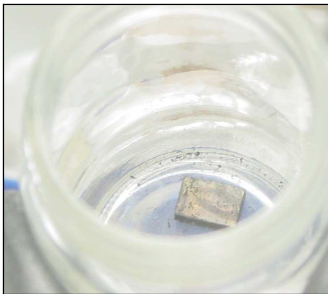
Figure 4-2 DU piece structurally intact but discolored after experiment 5
