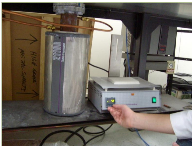
Figure 13. Furnace and furnace controls used in hydride-dehydride process.
