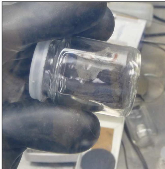
Figure 4-8 Break down of sintered powder after shaking the container
