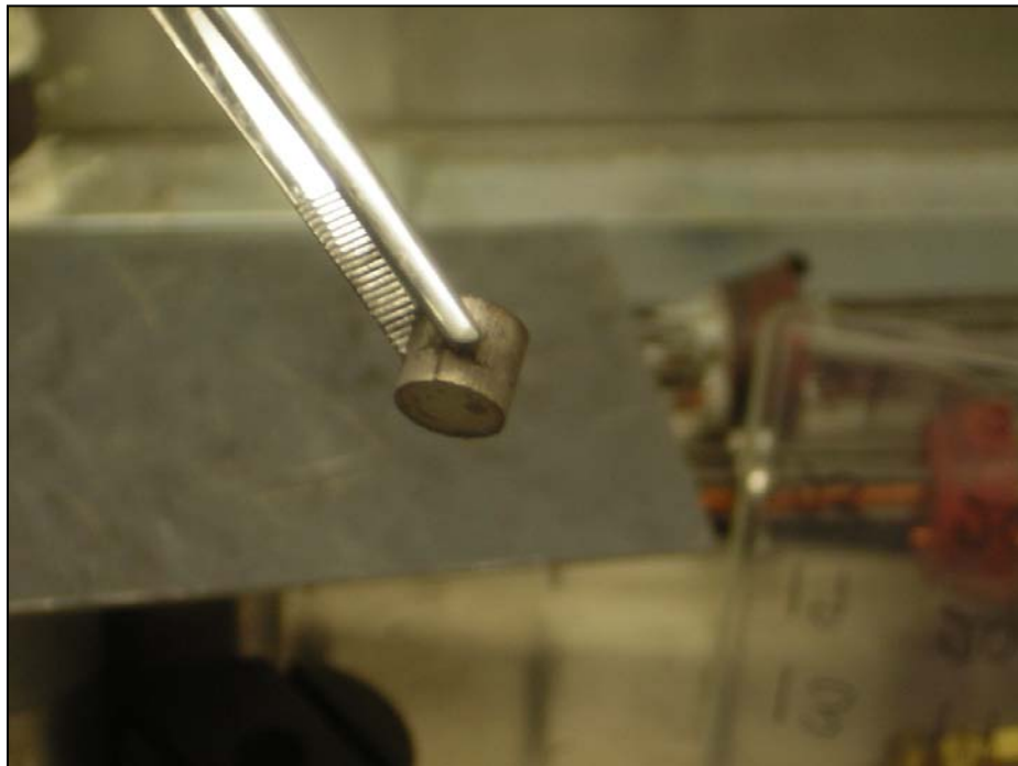
Figure 4-29: Pellet 10 after sintering.
