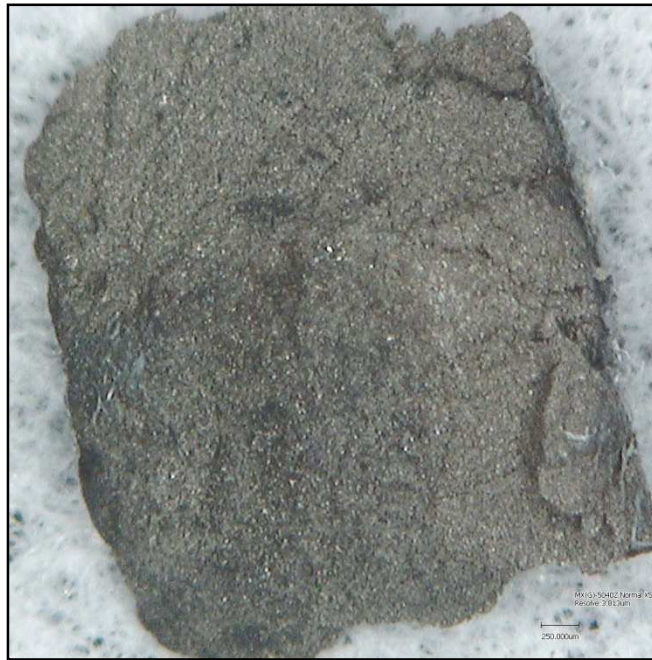
Fig. 4-16 DU powder sintered during dehydriding at 50X
