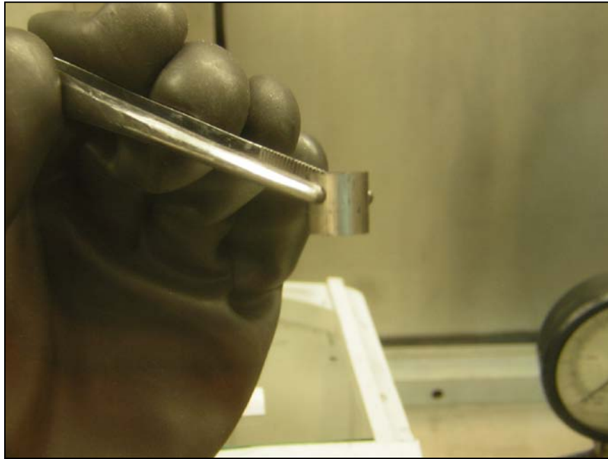
Figure 4-31: Pellet 11 as pressed, before sintering.
