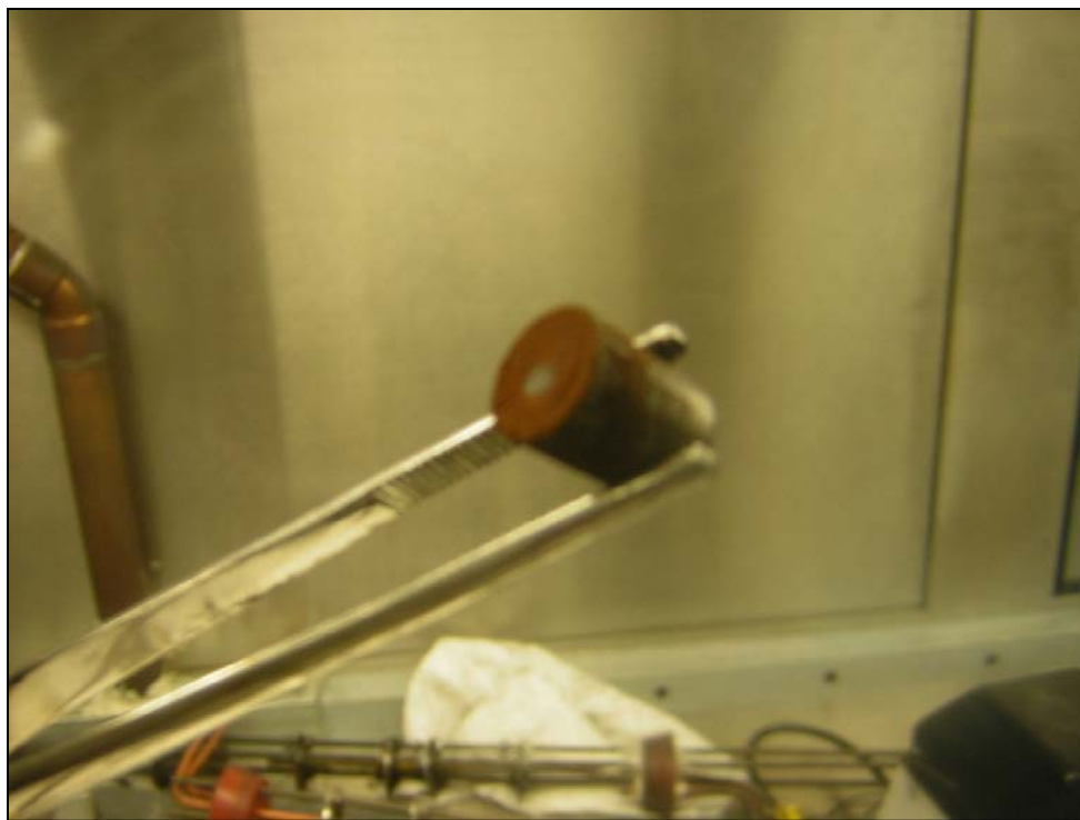
Figure 4-4: Pellet 3 after sintering, with red U-Fe powder formation.
