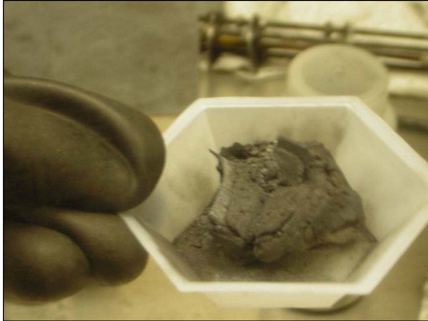
Figure 3-7: Loosely sintering DU coupons coated in powder following dehydriding.
