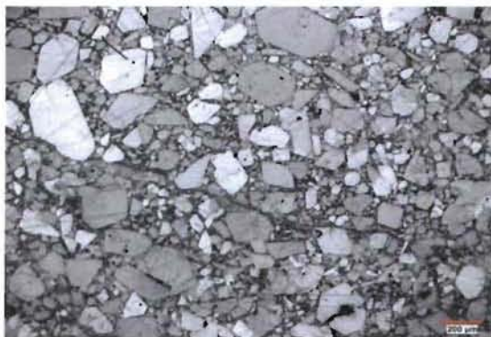
Figure 1. Micrograph of PBX 9501, illustrating the heterogeneous microstructure
