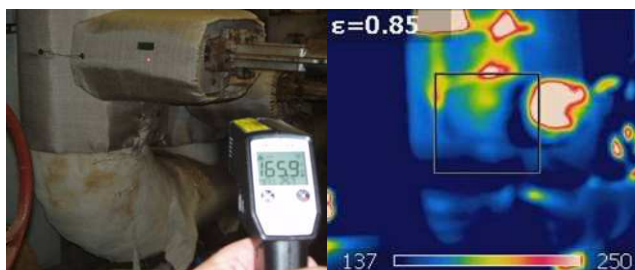
Figure 45. Pyrometer reading and infrared imaging of Pyrogel XT valve cover
