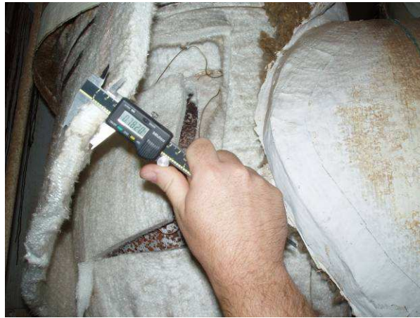
Figure 46. Measured thickness of in-use section of 1" glass mat shows the material compressed to 0.78"
