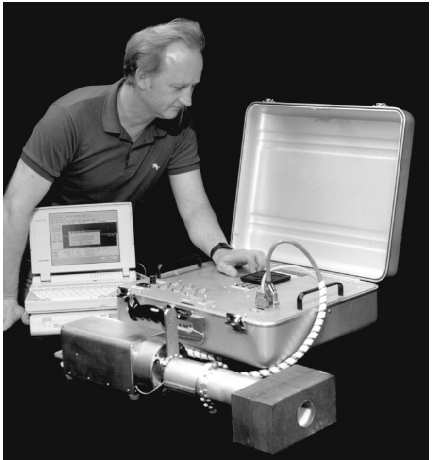
■ Figure 1. LLNL's electro-mechanically cooled germanium detector.
