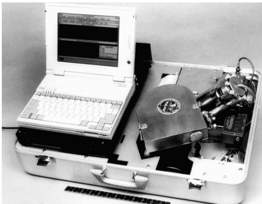
■ Figure 1. A small, portable GC-MS instrument contained in a standard 9.5 x 18 x 27-in. suitcase. The package contains a GC, MS, vacuum system, 486 computer, and support electronics. As shown, it weighs 69 lbs. We are modularizing the instrument and its associated equipment and packing so that users can select the modules appropriate to their analytical requirements, size, weight, portability, and use in the field.
