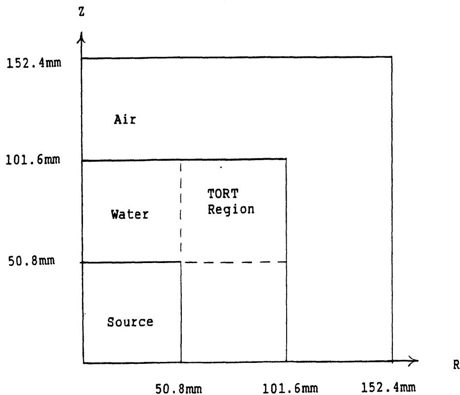
Fig. 1. Coupling of RZ DORT Reactor Calculation to XYZ TORT Geometry.
