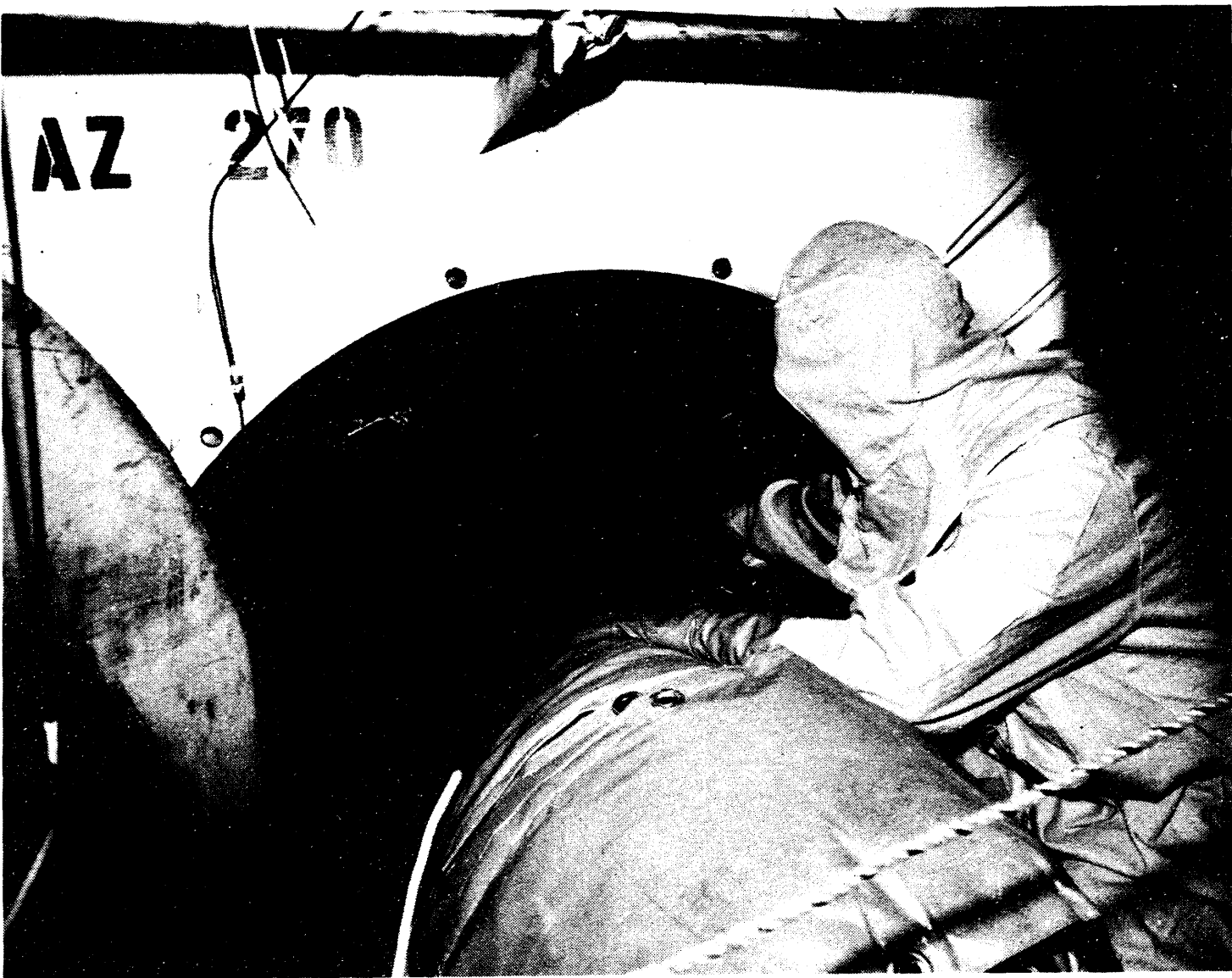
Figure 2.5. Waveguide AE Sensor Being Pressure Coupled to the Pipe Surface - Limerick Unit 1
