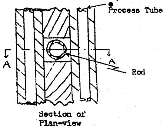
The next layer below or above this section results in filler blocks completely surrounding the rod.
