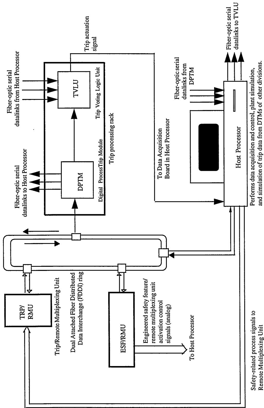
Fig. 1. Diagram of the prototypic reactor trip channel.
