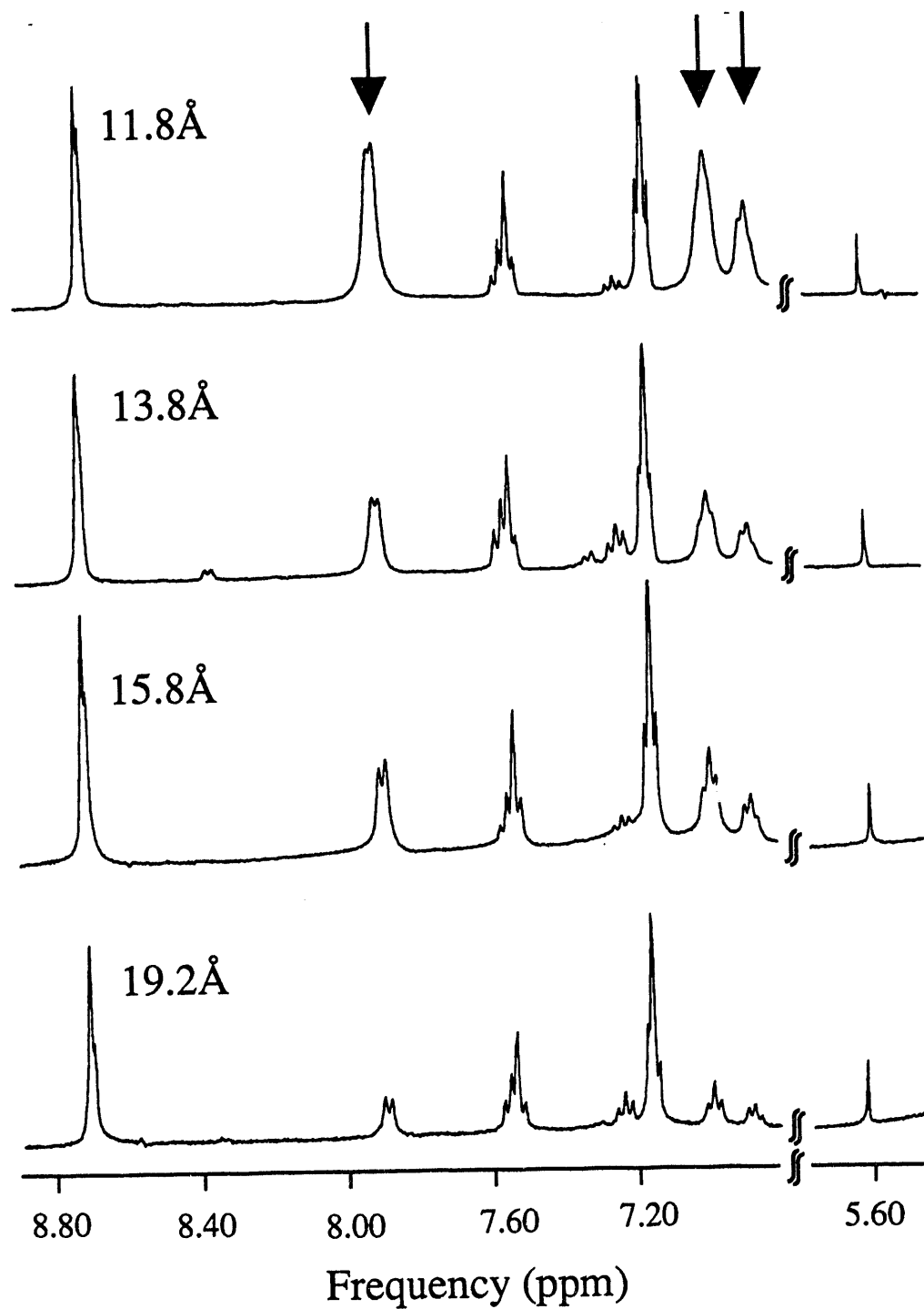
Figure 2.2.4: Intensity calibrated, size-dependent ^1\text{H} spectra of thiophenol capped CdS nanocrystals. The samples were made from the same stock solution of d_5 -pyridine to which had been added 0.9 mmoles of \text{CH}_2\text{Cl}_2 per kilogram of solution. The intensity of the \text{CH}_2\text{Cl}_2 at 5.68 ppm is constant in these spectra.
