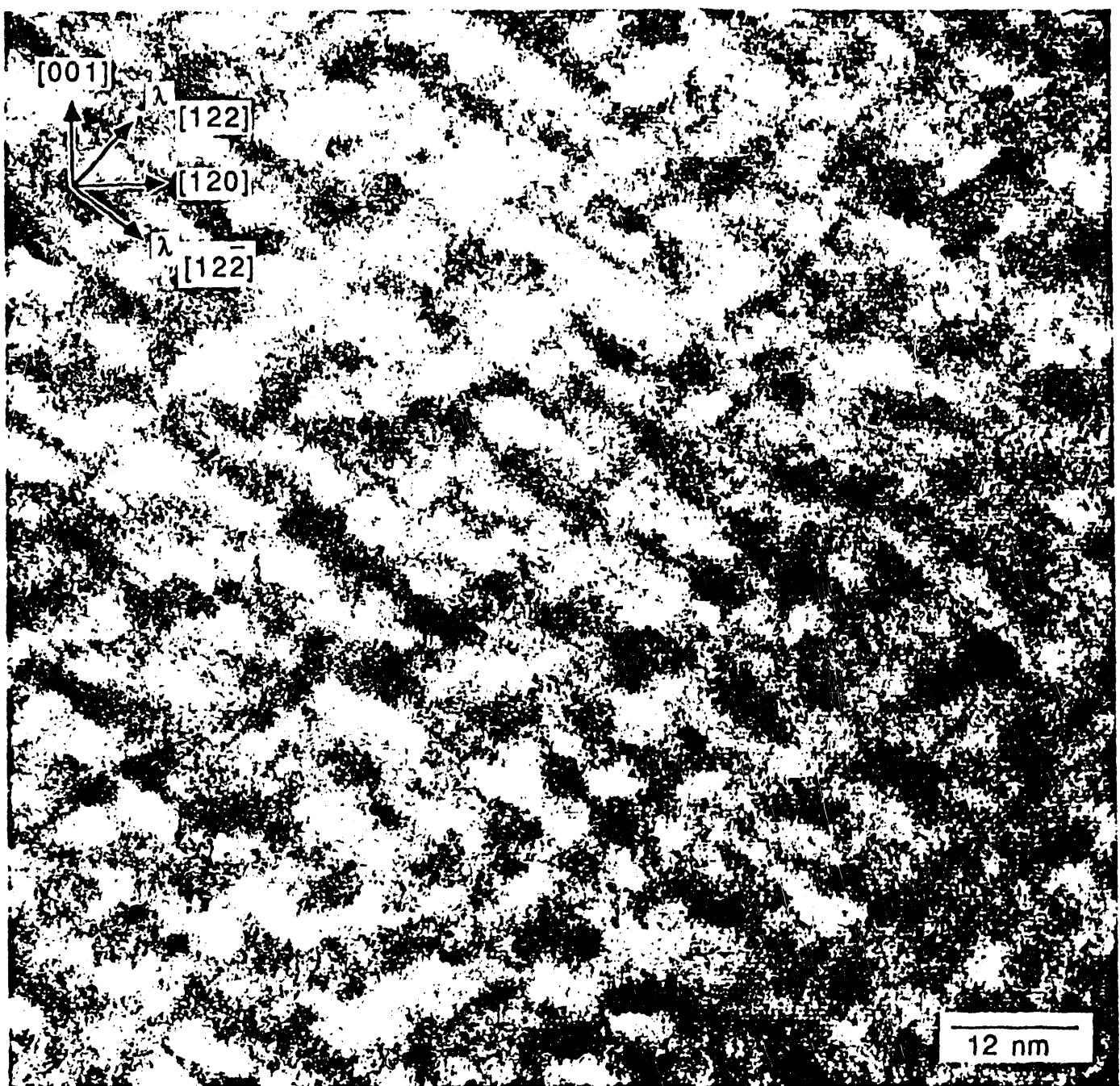
Figure #1(a): TEM high resolution image of SiC-AlN annealed at 1600°C for 320 hours.
