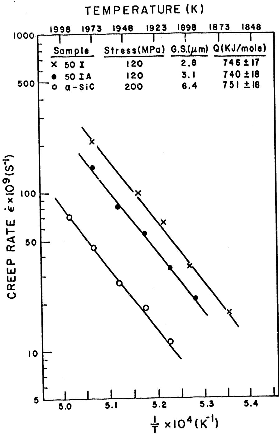
Figure #3: Plots of  $\log(\text{creep rate})$  vs.  $1/T$  for SiC-AlN solid solution, spinodally decomposed SiC-AlN, and  $\alpha$ -SiC.
