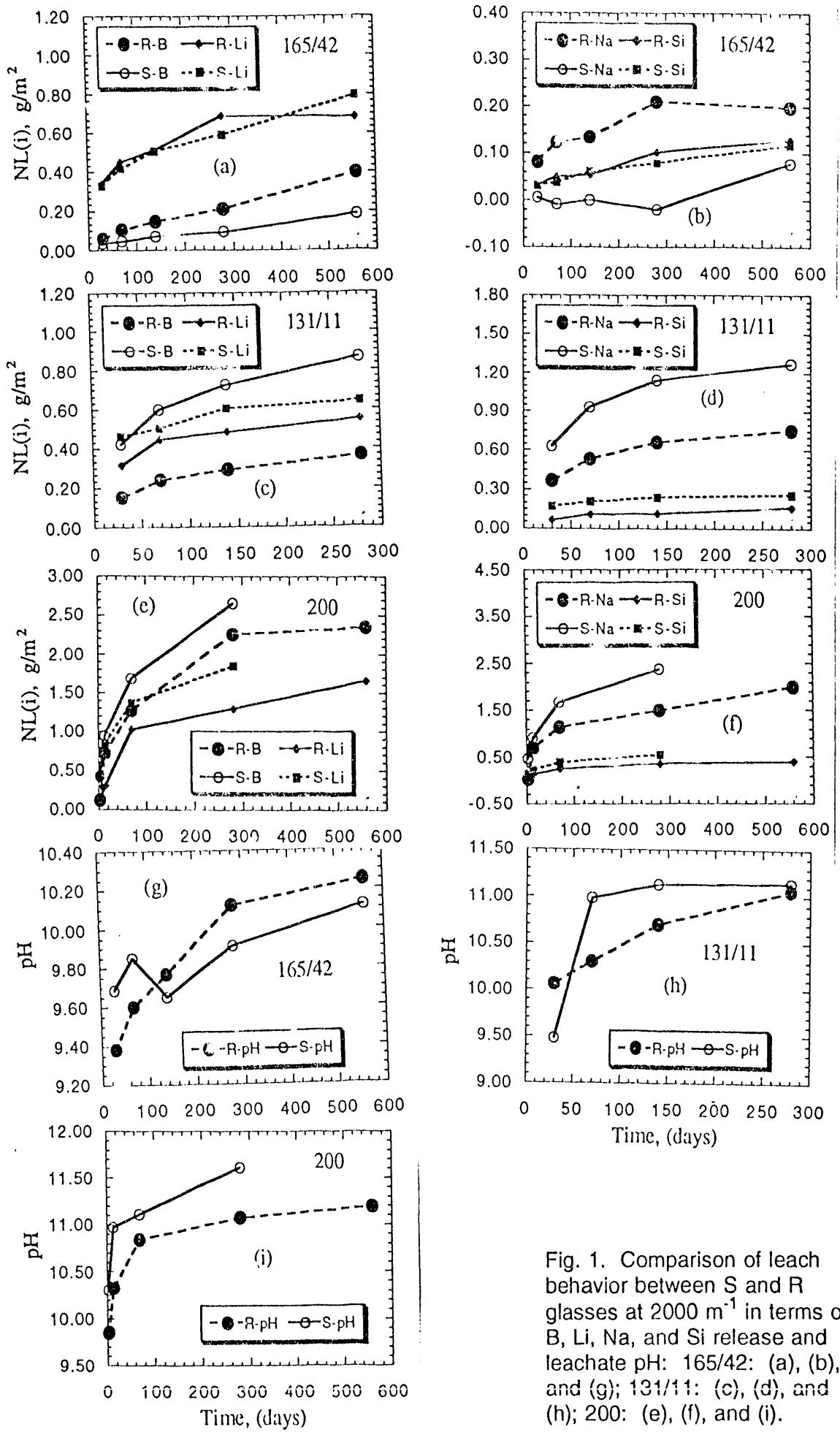
Fig. 1. Comparison of leach behavior between S and R glasses at  $2000 \text{ m}^{-1}$  in terms of B, Li, Na, and Si release and leachate pH: 165/42: (a), (b), and (g); 131/11: (c), (d), and (h); 200: (e), (f), and (i).
