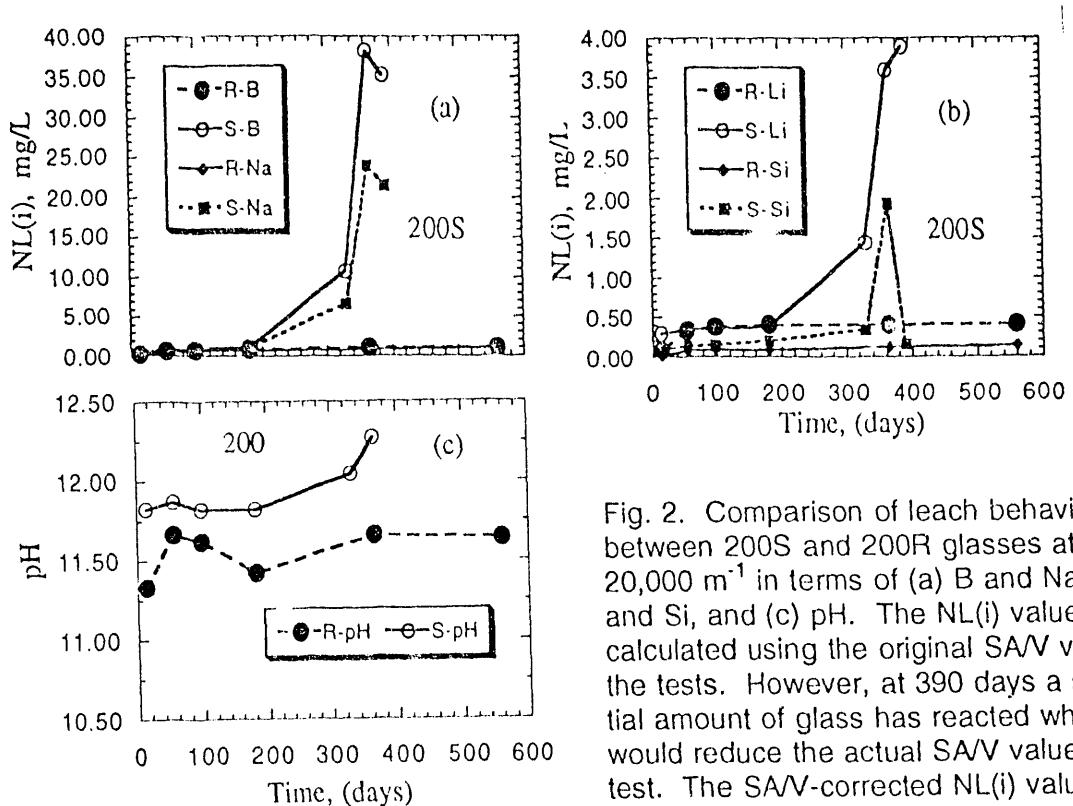
Fig. 2. Comparison of leach behavior between 200S and 200R glasses at  $20,000 \text{ m}^{-1}$  in terms of (a) B and Na, (b) Li and Si, and (c) pH. The NL(i) values are calculated using the original SA/V value of the tests. However, at 390 days a substantial amount of glass has reacted which would reduce the actual SA/V value of the test. The SA/V-corrected NL(i) values are higher than the NL(i) values shown above.
