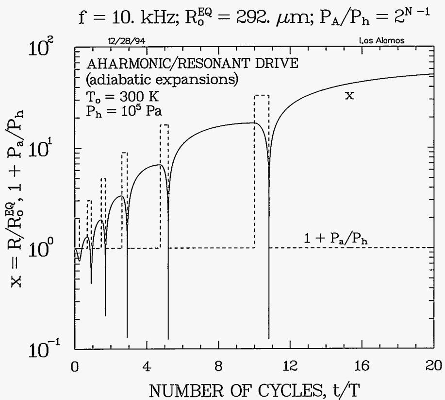
Figure 5. Response of normalized bubble radius to progressively doubled pressure pulses for conditions that are otherwise identical to those used for the harmonically driven case given on Fig. 3.
