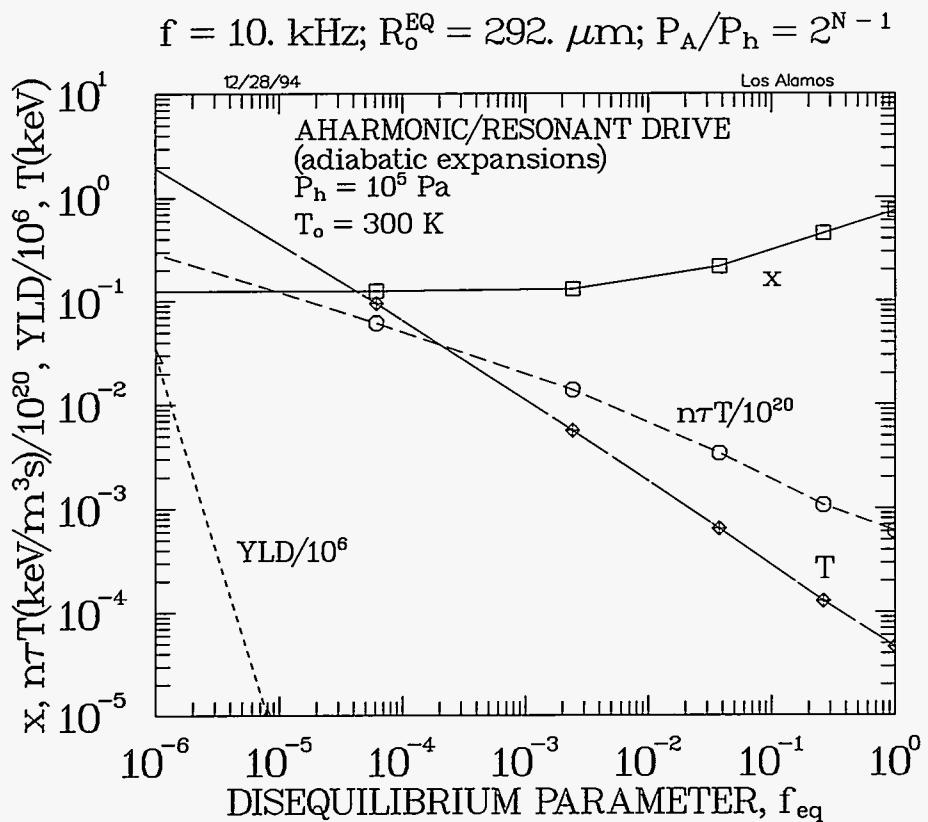
Figure 6. Dependence of integral and peak-compression parameters for the aharmonic/resonant drive given on Fig. 5.
