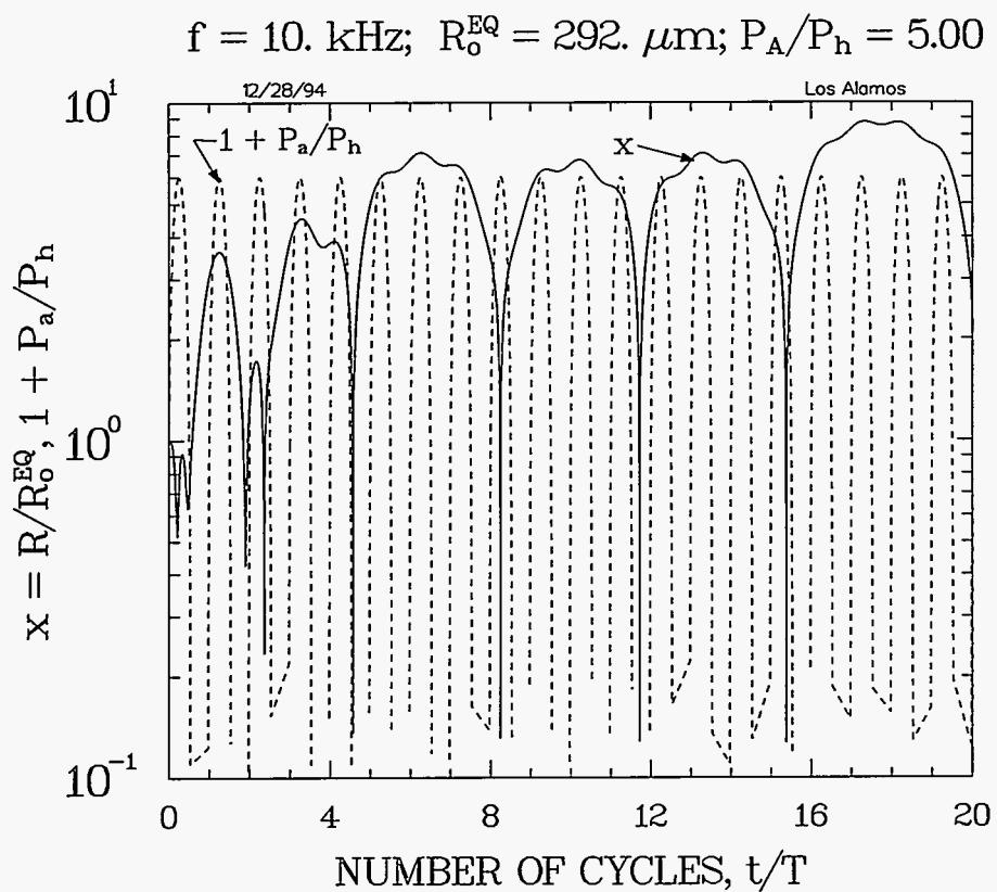
Figure 3. Response of normalized bubble radius to  $f = 10 \text{ kHz}$ ,  $P_A = 5 \times 10^5 \text{ Pa}$  sinusoidal pressure oscillations starting with a resonant ( $\omega_r = 2\pi f$ ), equilibrium ( $x, f_{\text{eq}} = 1$ ) bubble.
