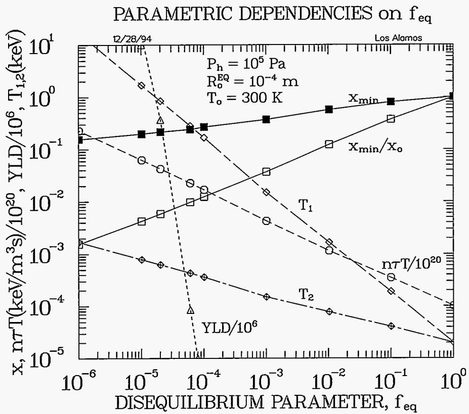
Figure 2. Parametric dependence of integral and peak-compression parameters on disequilibrium parameter,  $f_{eq} = P_{go}/P_{go}^{EQ}$ .
