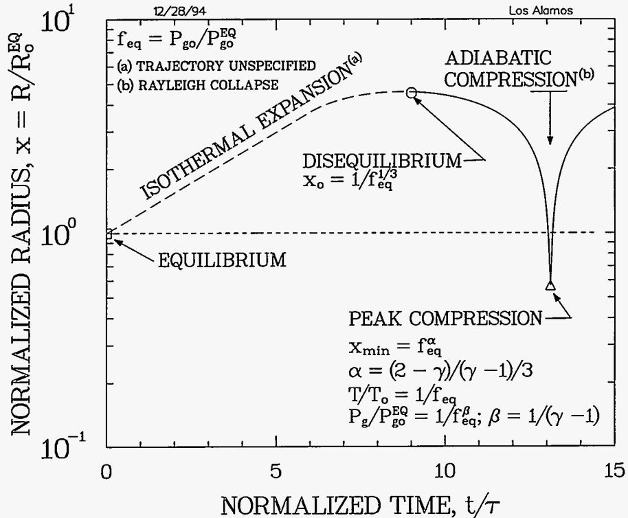
Figure 1. Schematic diagram of bubble radius trajectory illustrating approach to  $f_{eq} < 1$  disequilibrium from  $f_{eq}, x = 1$  equilibrium state, followed by collapse to  $x_{min}$ .
