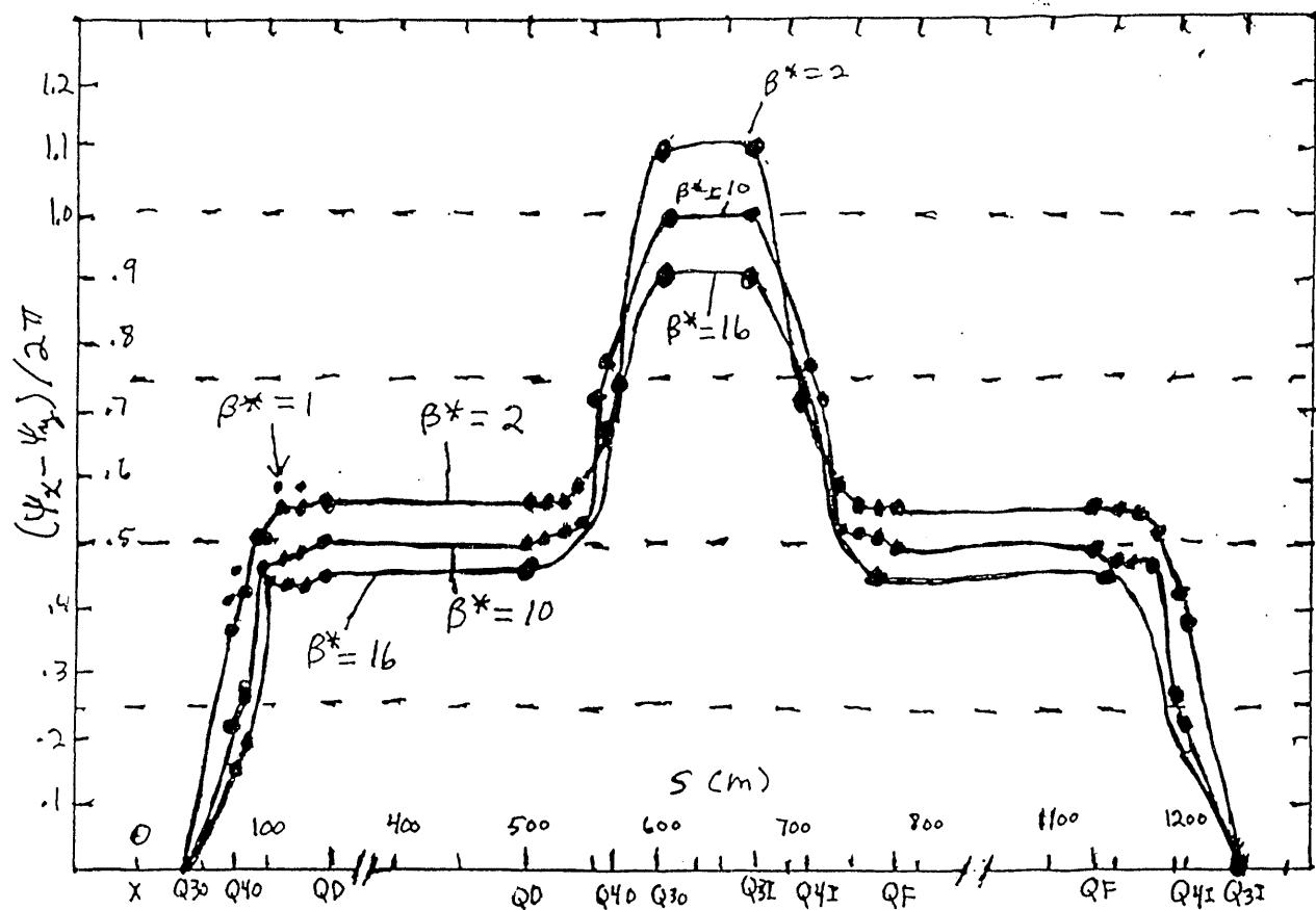
Figure 2: Plot of  $(\psi_x - \psi_y)/2\pi$  against  $s$  for RHIC92 lattices with  $\beta^* = 1, 2, 10, 16$ . The  $\beta^* = 1$  curve nearly overlaps the  $\beta^* = 2$  curve except for the indicated points for  $\beta^* = 1$ .
