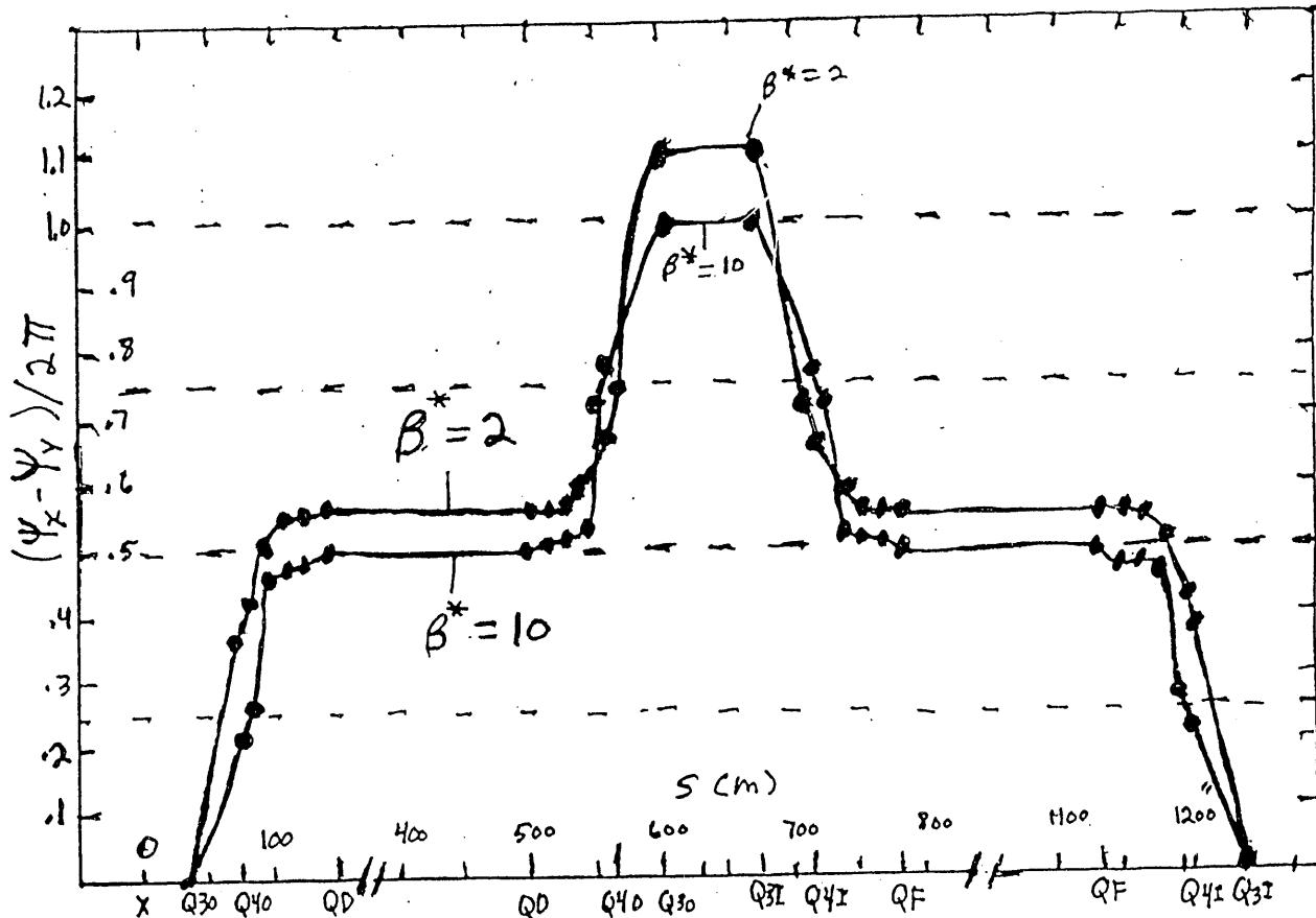
**Figure 1:** Plot of  $(\psi_x - \psi_y) / 2\pi$  against  $s$  for the RHIC92 lattice with 6  $\beta^* = 10$  and 6  $\beta^* = 2$  insertions. Each dot on the curves indicates the location of a quadrupole.
