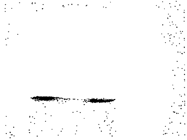
b. Liquid in motion (black areas) revealed by subtracting two adjacent incoming images and thresholding the result.
