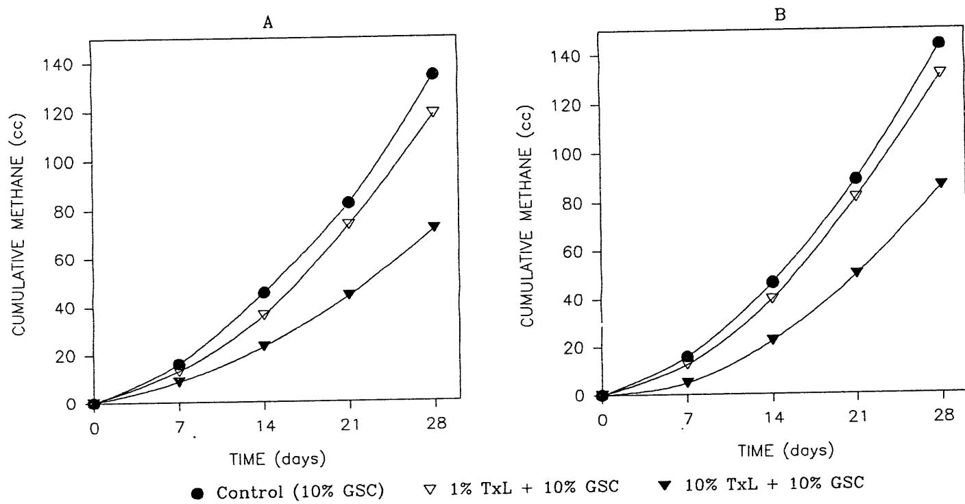
Figure 1. Influence of Different Anaerobic Conditions  $H_2:N_2$  (A) and  $N_2:CO_2$  (B) on Cumulative Methane Production by Granulated Sludge Consortium (GSC).
