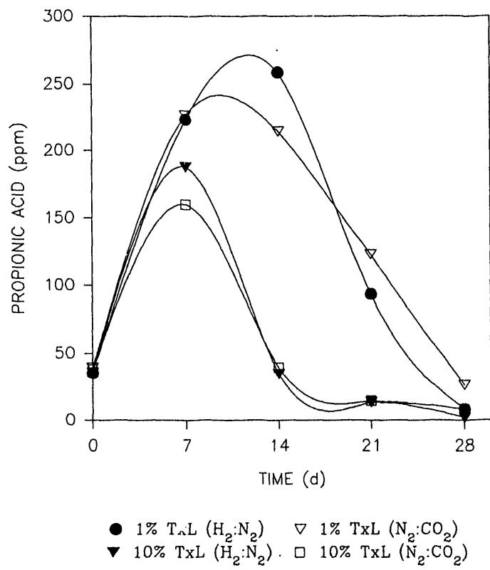
Figure 4. Time Course of Propionic Acid Concentrations During Biomethanation of 1% and 10% Texas Lignite by the 10% Granulated Sludge Consortium
