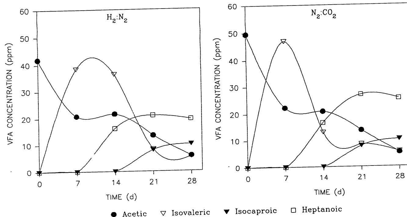
Figure 2. Time Course of VFA Concentrations During Biomethanation of 1% Texas Lignite by the 10% Granulated Sludge Consortium
