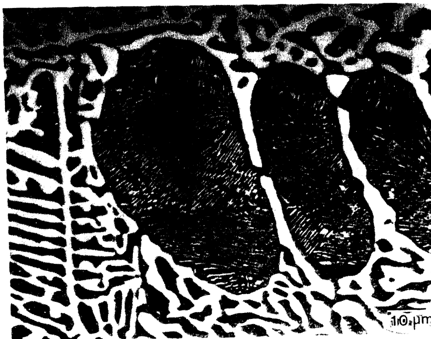
Figure 4.2 - Optical micrograph of Bi-Sn sample showing Bi precipitates within Sn dendrites. [XBB 939-5984 (Bottom)]
