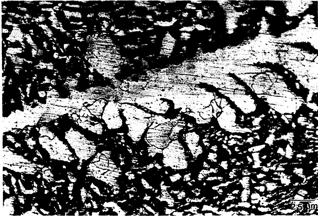
Figure 4.27 - Optical micrograph of \gamma phase dendrite within tested In-Sn on Cu sample. The dark lines in the dendrite are assumed to be grain boundaries. [XBB 934-2400]
