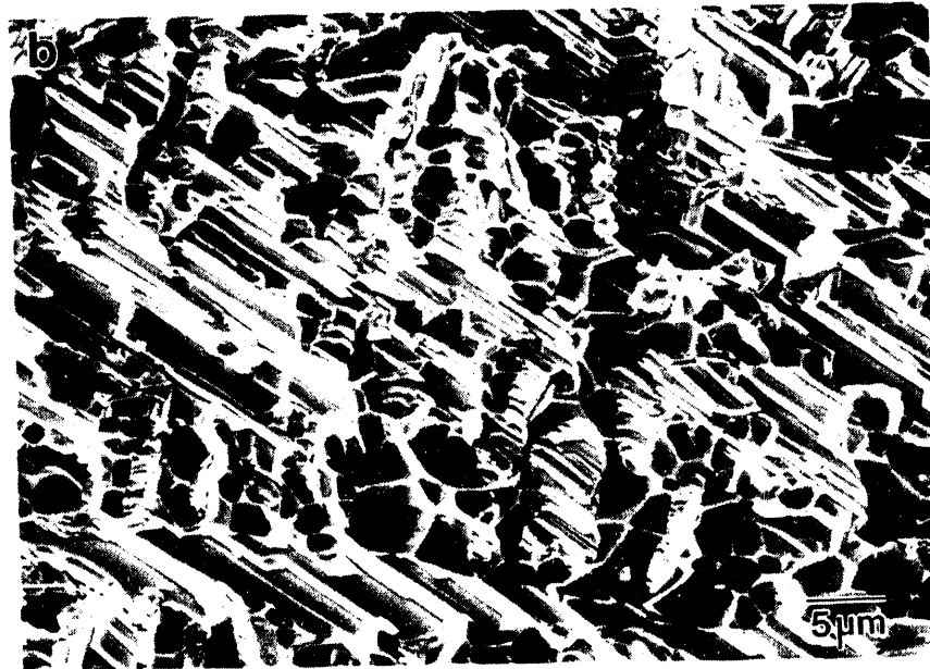
Figure 4.29 - SEM micrograph of fracture surfaces of Bi-Sn sample. (a) side 1, with Bi phase (faceted) and intermetallic particles, and (b) side 2, with Bi phase and dimples where intermetallic separated from surface. [XBB 9311-7265]
