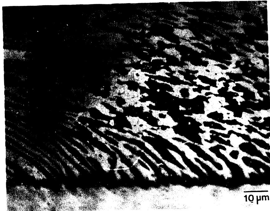
Figure 4.20 - Optical micrograph of Bi-Sn sample tested at constant strain rate and repolished. [XBB 920-9580A]
