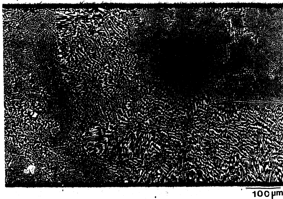
Figure 4.1 - Optical micrograph of untested Bi-Sn sample. In this and all optical micrographs of Bi-Sn, the Bi phase appears light and the Sn-rich phase appears dark. [XBB 939-5984 (Top)]
