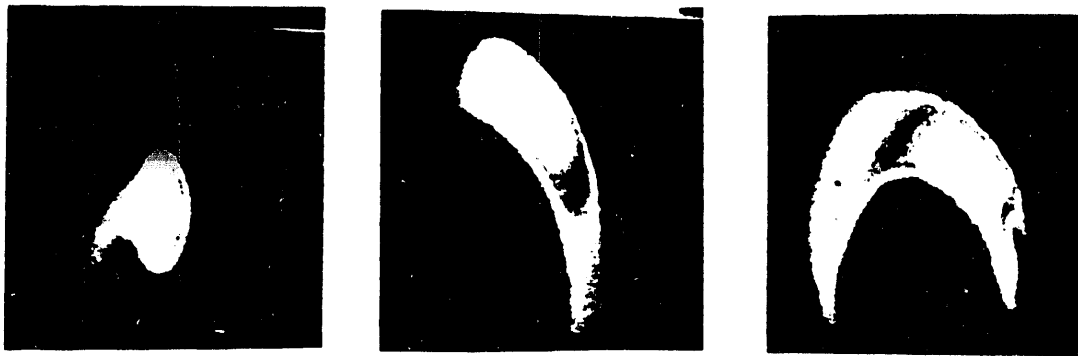
Fig. 9 Profiles (x-y) of a 2 \times 10^{10} e - bunch at 47 GeV with a 0.2 mm oscillation (left), with a 0.5 mm oscillation (center), and with a 1 mm oscillation (right) in both planes. The initial core sizes in both planes are about 120 \mu m.
