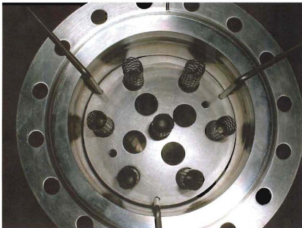
Picture showing fixture in place to center Pd/Ag tubes during catalyst loading.
