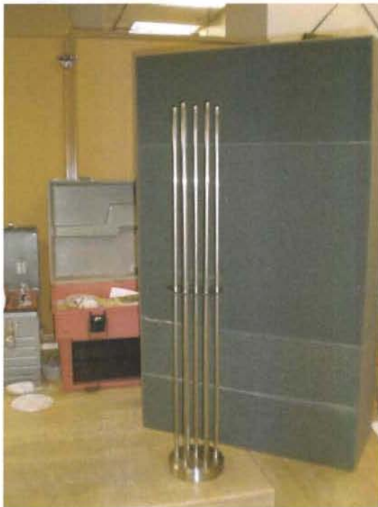
Picture showing Pd/Ag tubes brazed to collection plate during fabrication (at the factory).
