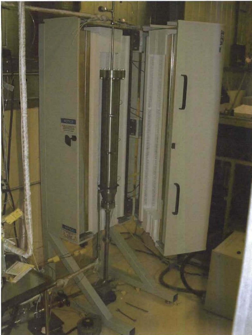
Picture showing the fully assembled PMR inside of the heating furnace.
