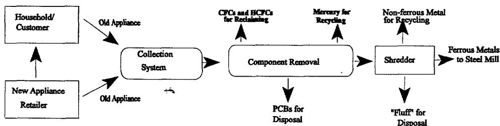
FIGURE 1 Appliance Flow Diagram
