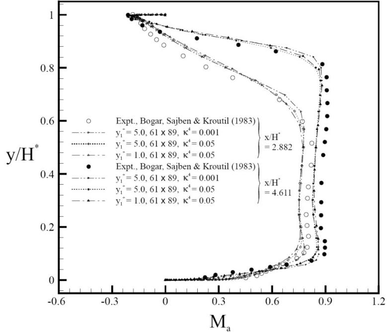
Figure 3-16: Predicted velocity profiles for separating transonic diffuser.
