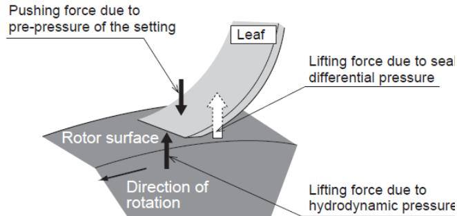
Fig. 7 Mechanism of leaf seal operation
