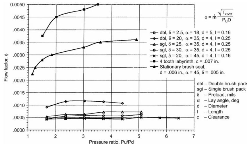
Figure 65.—HFBS performance compared to a stationary brush seal and a labyrinth seal. [ $\dot{m}$  is the mass flow rate of air (pps),  $T_{ave}$  is the average upstream air temperature (°R),  $P_u$  is the average upstream air pressure (psia),  $D$  is the shaft outer diameter (in.)].<sup>146</sup>
