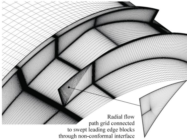
**Figure 3-37: Computational grid used for Rampressor rotor simulations.**
