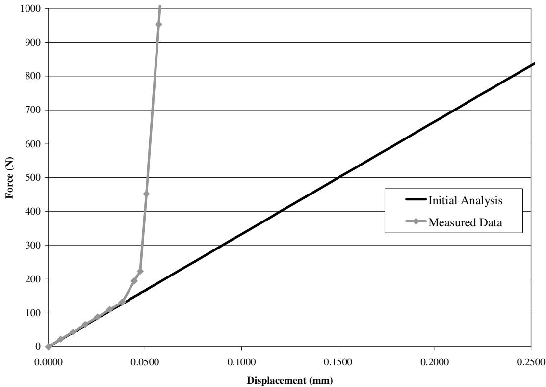
**Figure 2-5: Comparison of initial linear o-ring model and measured nonlinear stiffness.**
