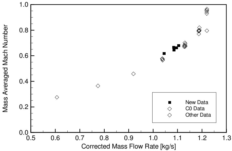
**Figure 4-26:** Calculated mass averaged Mach number at IGV exit probe location. The solid symbols represent new data discussed in this section while the open symbols are data from previous measurements reported by Williams (2007). The new data are in general agreement with previous measurements.
