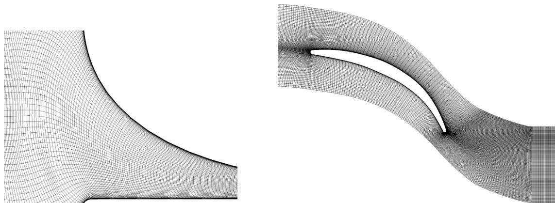
**Figure 3-42: Bellmouth and inlet guide vane grid resolution.**
