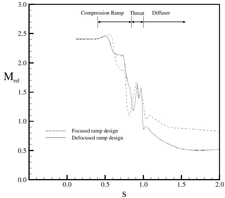
**Figure 3-39: Comparison of focused and defocused relative centerline Mach number vs. normalized streamwise distance.**
