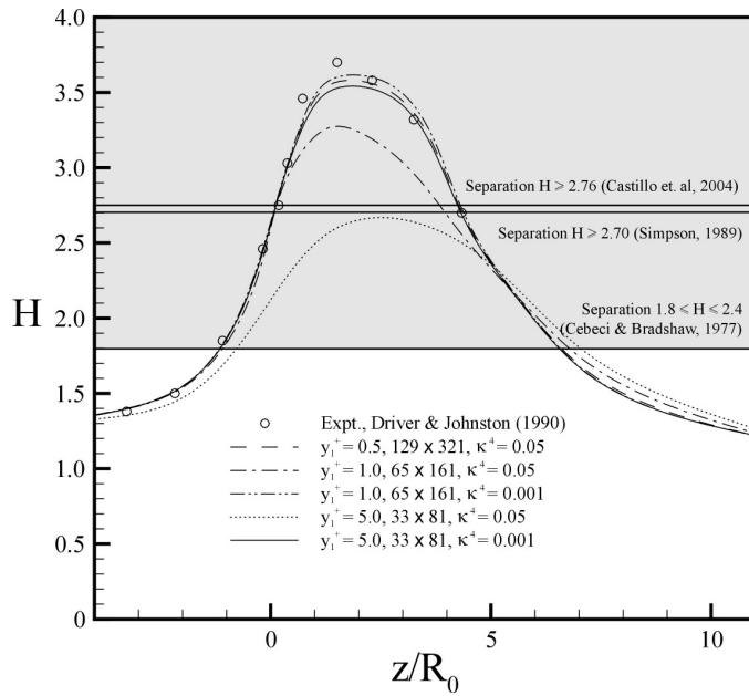
Figure 3-10: Annular separating diffuser shape factor prediction.
