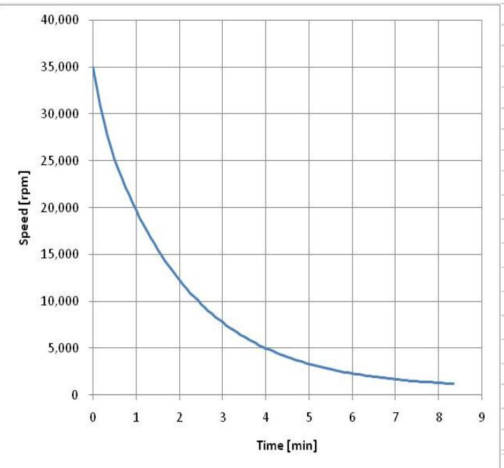
**Due to high rotational speeds, ~10 minute rundown predicted for motor/gearbox/compressor**
