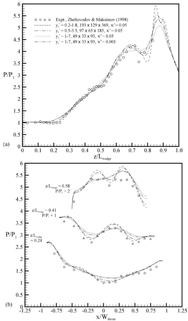
**Figure 3-21: Asymmetric crossing shockwave flow prediction of platform static pressure distribution at (a) centerline and (b) cross stream.**
