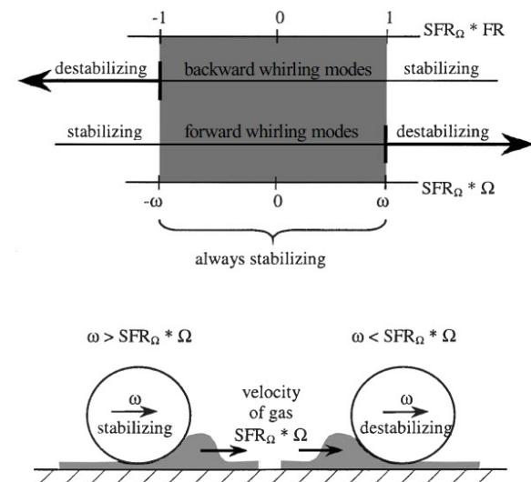
Figure 4. Stability Criterion of Labyrinth Seals.
