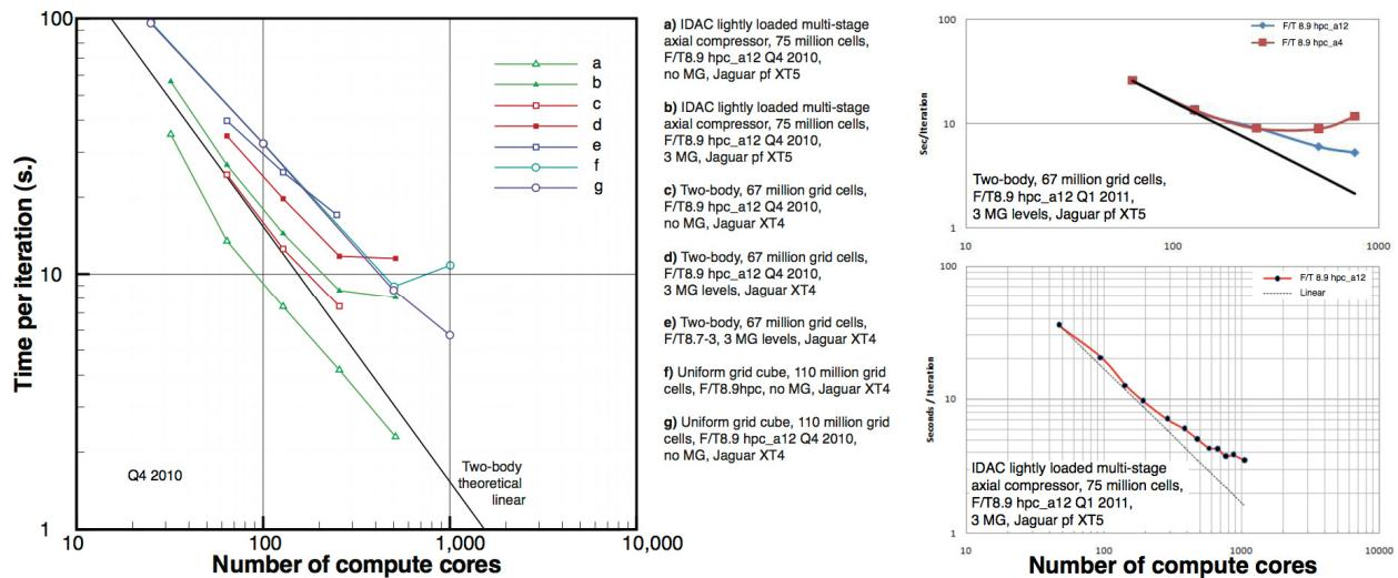
Figure 2: Demonstration of parallel scalability performance measured using a series of test cases. Substantial improvements in the parallel efficiency and practical number of cores that can be run per simulation has been demonstrated over the last year for a series of both linear / stationary, as well as rotating turbomachinery test cases in the 50-100 million grid cell range.
