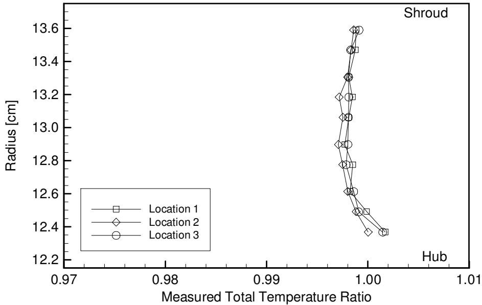
**Figure 4-13: Radial surveys of total temperature ratio, bellmouth to end of inlet, at three different circumferential locations with the rotor at 107% corrected speed.**
