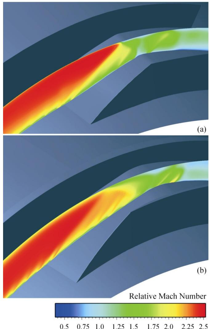
**Figure 3-38: Viscous rotor passage model comparison of relative Mach number at mid-pitch for (a) focused (max PR 6:1) and (b) defocused (max PR 8:1) ramp designs.**
