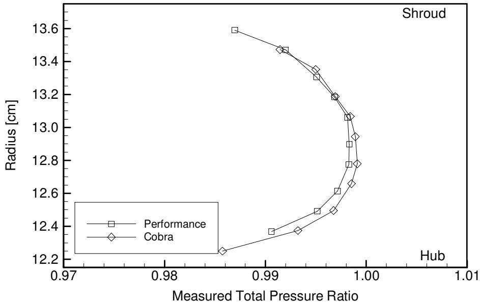
**Figure 4-8: Radial surveys of total pressure ratio, plenum to end of inlet, using two different total pressure probes at circumferential location 1 at 107% corrected speed.**
