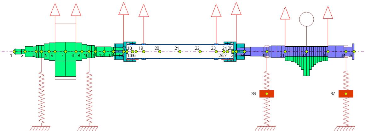
Figure 2-1: DyRoBeS model with the replacement quillshaft.
