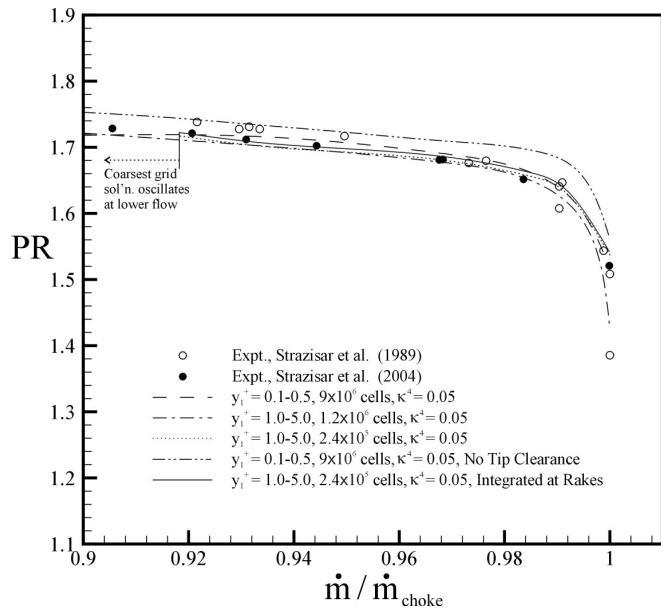
Figure 3-25: Transonic fan rotor flow simulation predicted pressure ratio.
