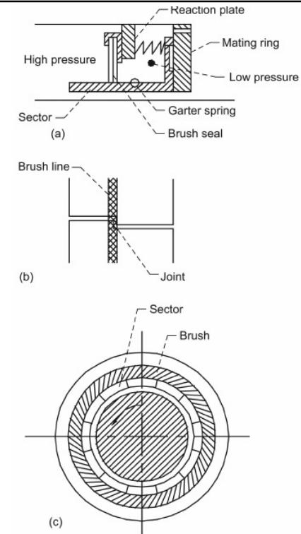
Figure 63.—Schematic of film riding brush seal. (a) Assembly. (b) Joint. (c) Installed.<sup>143</sup>
