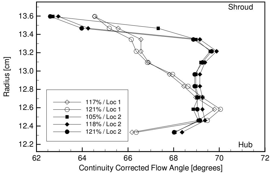
**Figure 4-22: Continuity corrected flow angle radial profiles at different probe locations and corrected speeds.**
