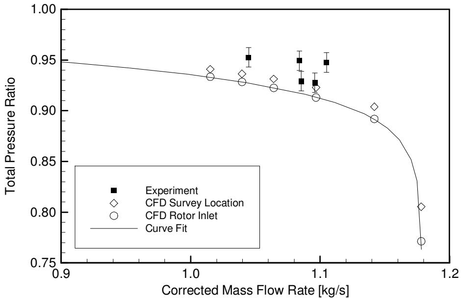
**Figure 4-25:** Calculated mass averaged total pressure ratio from IGV exit to plenum compared with CFD simulation presented in Figure 3-47. The measurements are in general agreement with the CFD simulations.
