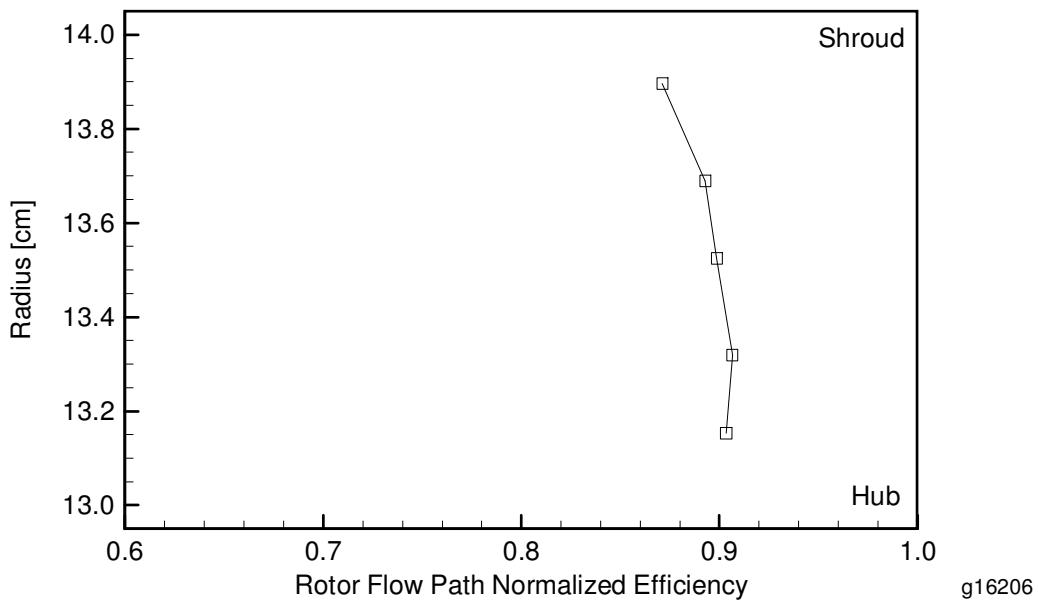
**Figure 4-34: Radial variation of normalized efficiency for a test at 120% corrected speed.** The survey shown is the same as in Figure 4-31.
