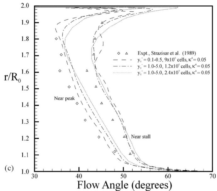
Figure 3-29: Transonic fan rotor flow predicted exit angle profile.
