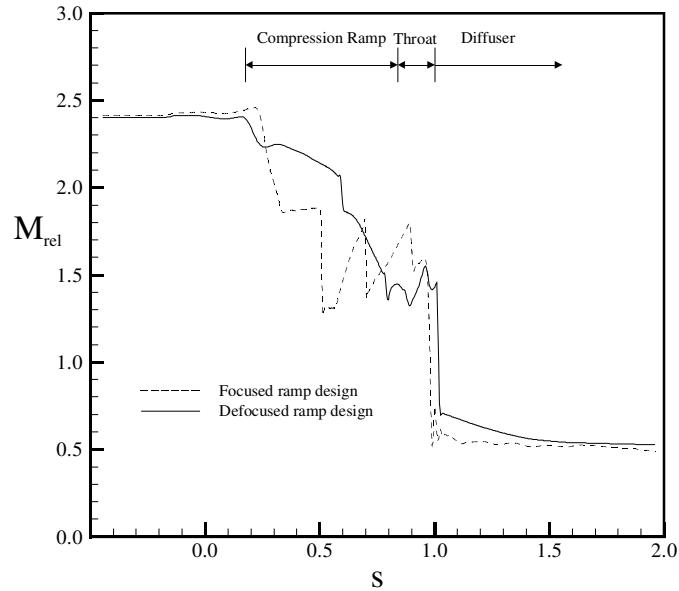
**Figure 3-34: Comparison of focused and defocused relative centerline Mach number vs. normalized streamwise distance.**
