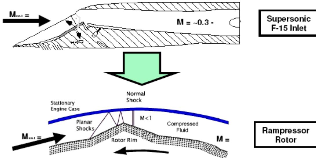
Figure 1-2: Ramgen rotor profile and its relationship to a supersonic flight inlet.
