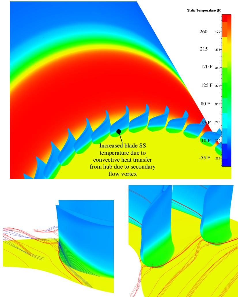
**Figure 3-44: Inlet guide vane secondary flow vorticity.**
