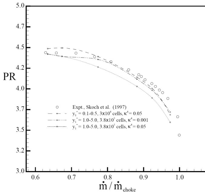
Figure 3-12: Predicted pressure ratio for 4:1 centrifugal impeller at 100% speed.
