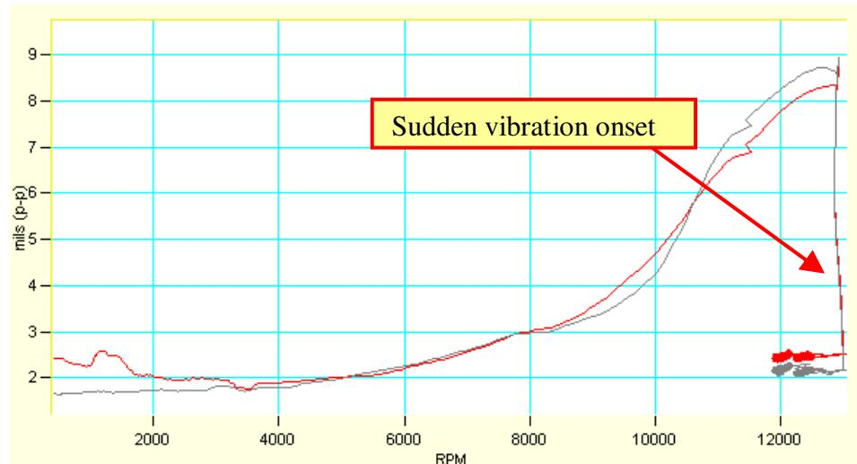
Figure 2-7: Run 65a – Sudden turbine shaft orbit increase and subsequent deceleration.
