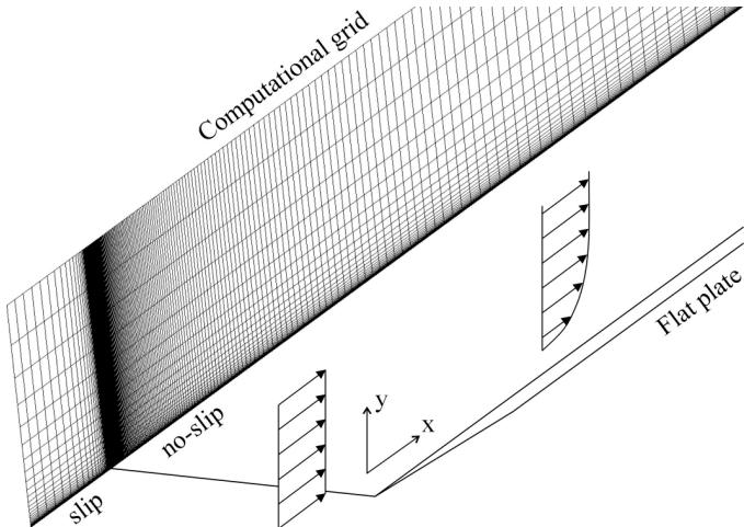
**Figure 3-1: Schematic view of flat plate flow and computational grid used in simulations.**
