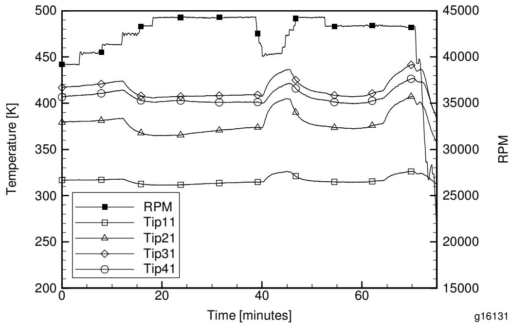
**Figure 4-4: Tip ring temperatures detect flow path starting and unstarting with rotor speed variation.**
