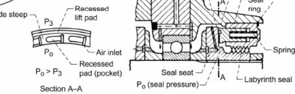
Figure 45.—Self-acting face seal with labyrinth seal presealing.<sup>110</sup>
