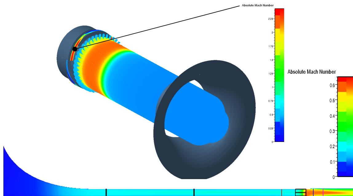
Figure 3-48: IGV and rotor coupled via mixing plane rotor/ stator interface.
