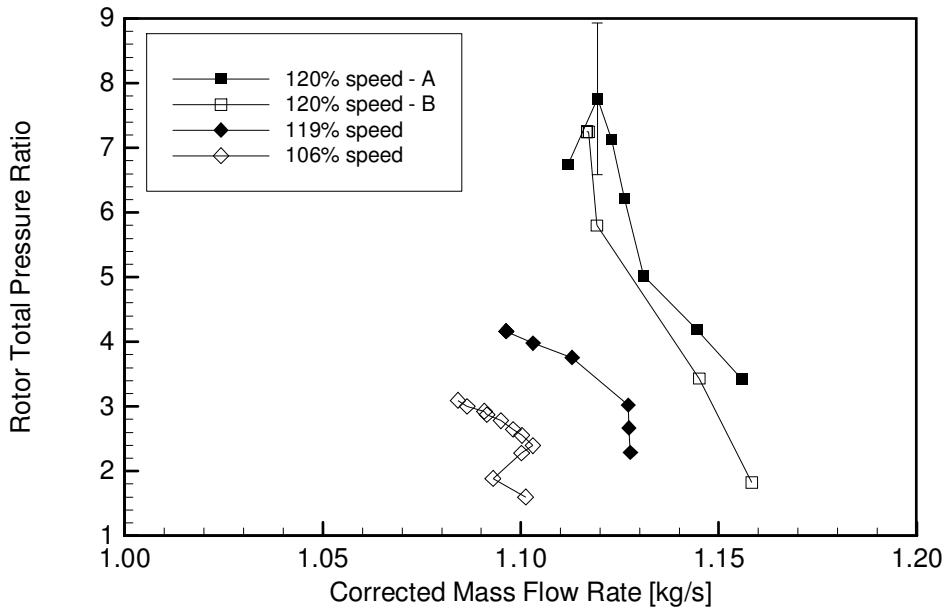
**Figure 4-30:** Variation of corrected mass flow rate with total pressure ratio and the effect of tip clearance. See text for details on tip clearance for each speed line.
