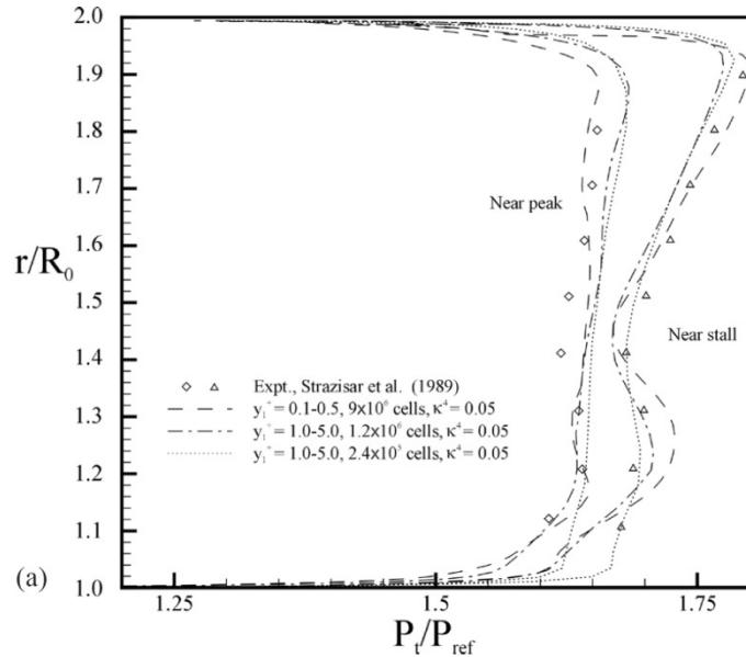
Figure 3-27: Transonic fan rotor flow predicted total pressure ratio profile.
