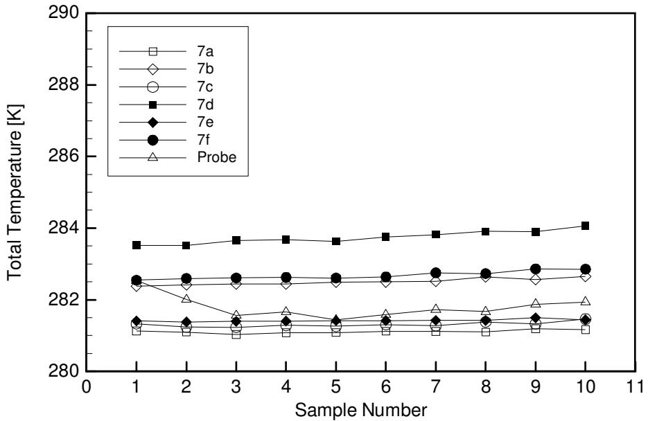
**Figure 4-12: Measured inlet total temperature during a typical high speed test with forward bleed. The data are from the same test as those in Figure 4-11.**
