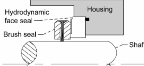
Figure 64.—The Hybrid Floating Brush Seal (HFBS).<sup>146</sup>
