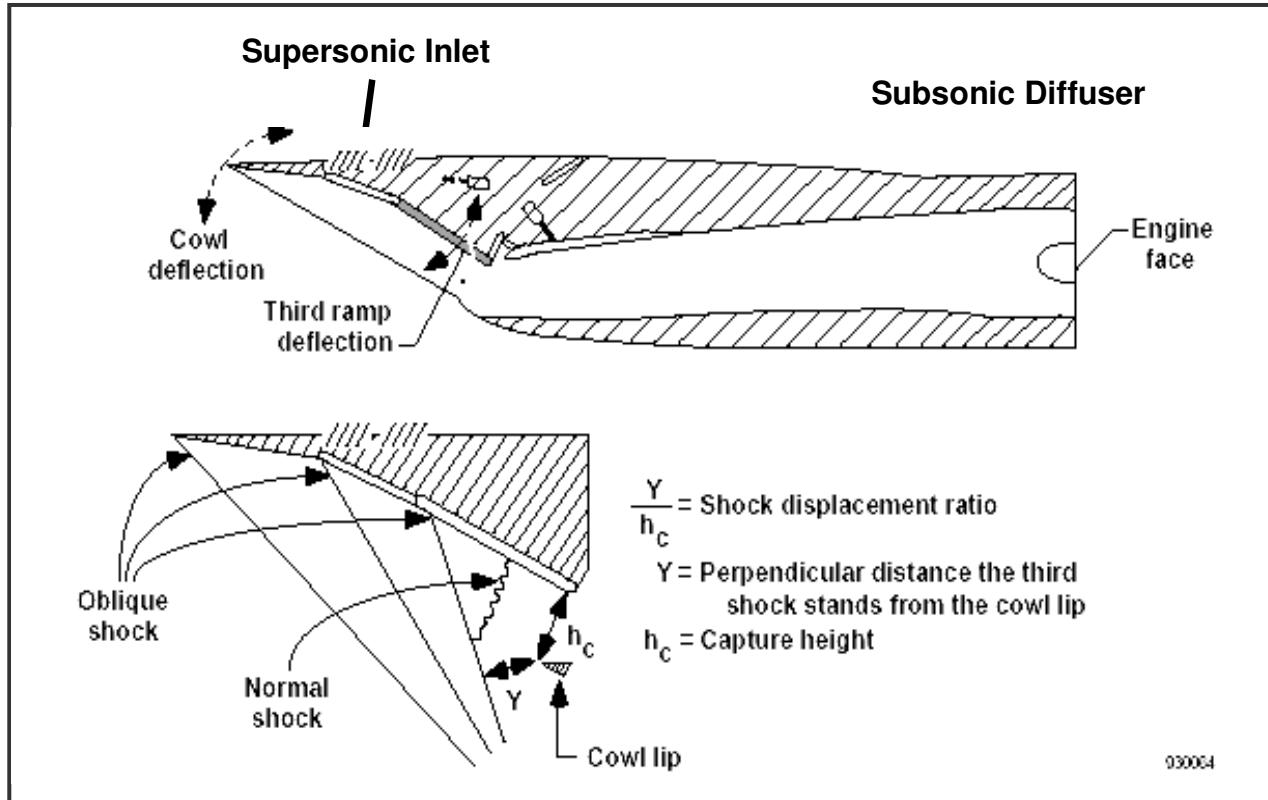
Figure 2.4.2 F-15 Supersonic Inlet Cross Section Detail
