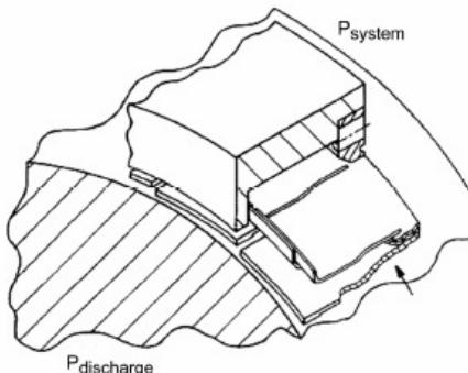
Figure 59.—Pressure balanced compliant film riding leaf-seal.<sup>140</sup>
