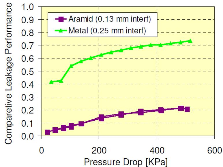
Fig. 8 Sample Aramid Seal Leakage Data
