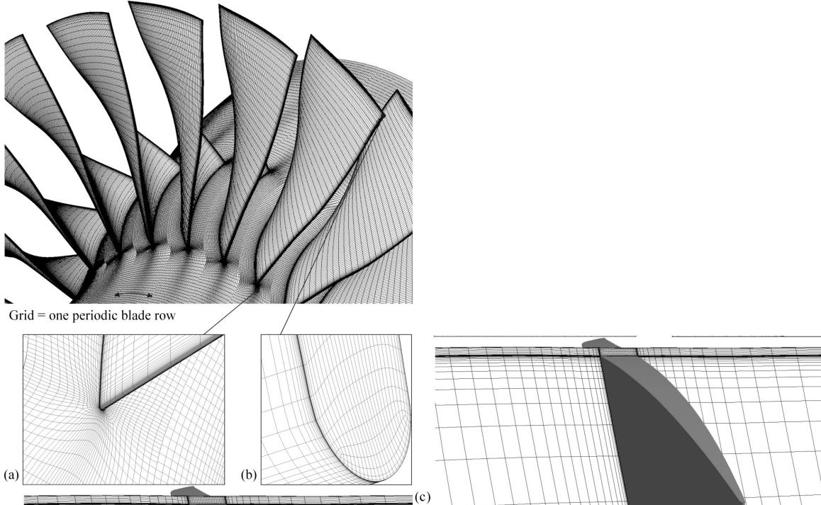
**Figure 3-22: Transonic fan rotor flow computational grid used in simulations. The intermediate resolution is shown here. Figure (a) shows the leading edge at the hub. Figure (b) shows the leading edge at the tip. Figure (c) shows the spanwise grid distribution in the tip clearance region.**
