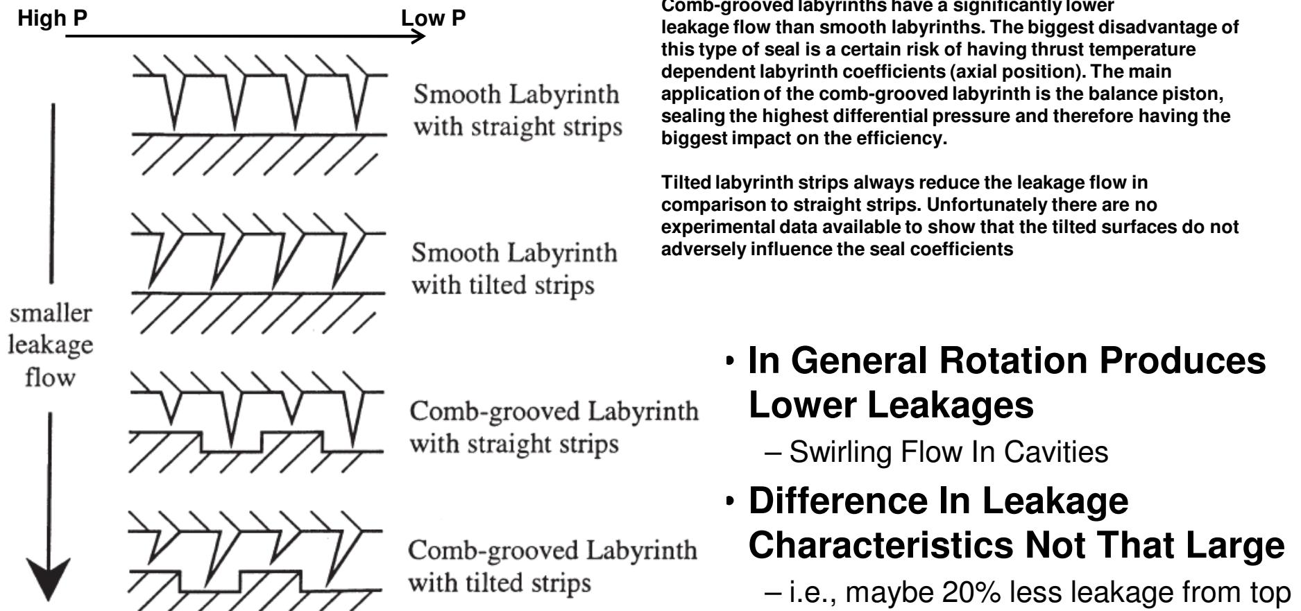
Figure 2. Labyrinth Seals Used in High Pressure Applications.
