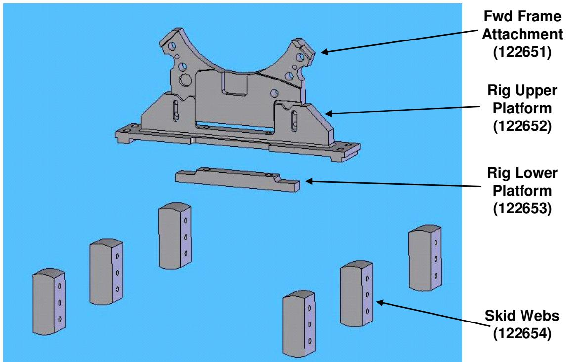
Figure 2-2: Forward end frame stiffness enhancement components.
