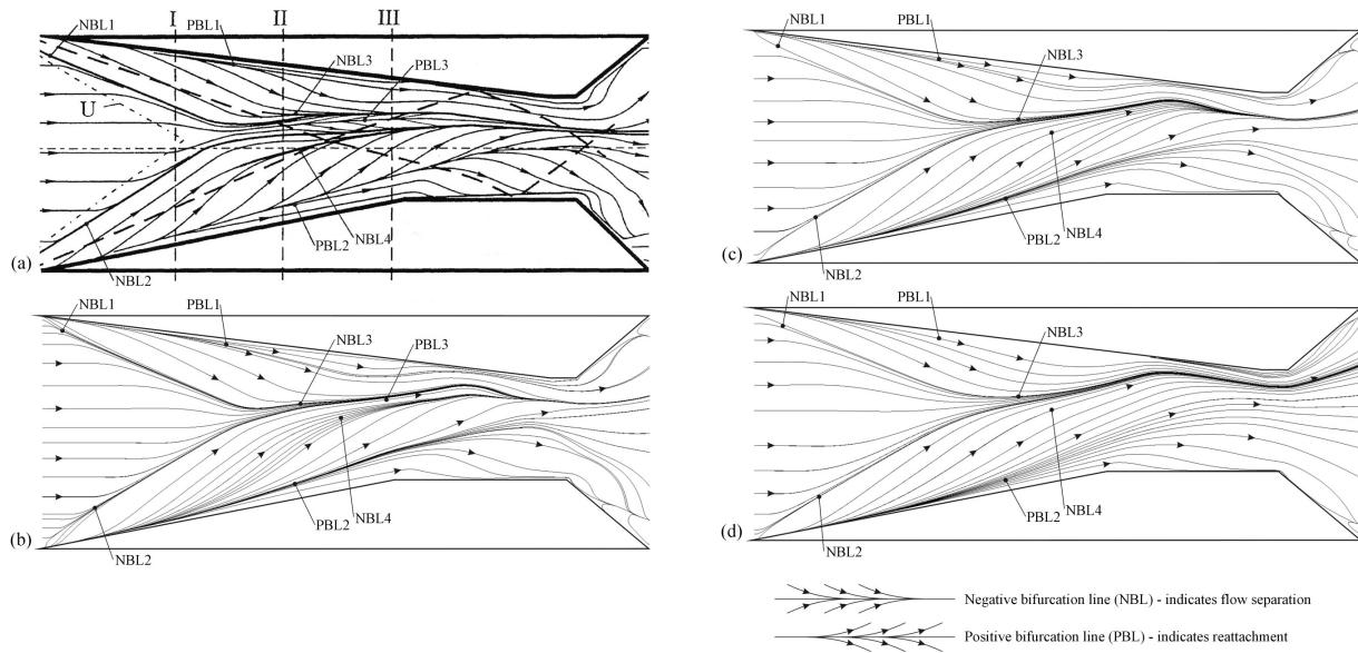
**Figure 3-20: Shock induced separation prediction using limiting surface streamlines. Figure (a) shows the experimental results while figures (b)-(d) show the finest to coarsest grids, respectively.**
