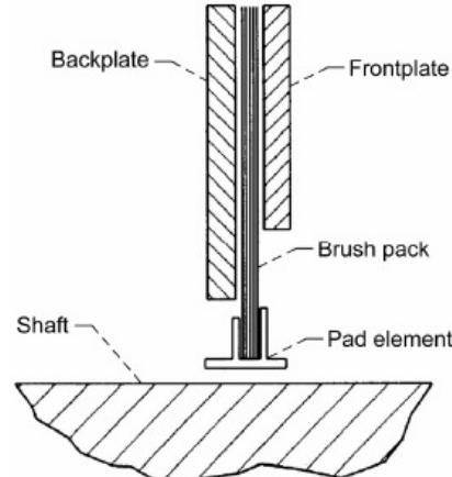
Figure 61.—Illustration of hydrodynamic brush seal (pad elements attached to bristles).<sup>141</sup>
