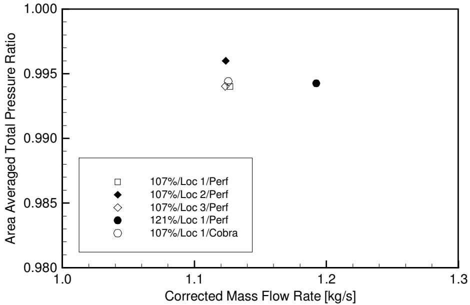
**Figure 4-9: Area averaged total pressure ratio, plenum to end of inlet, for each of the surveys presented in the previous three figures.**
