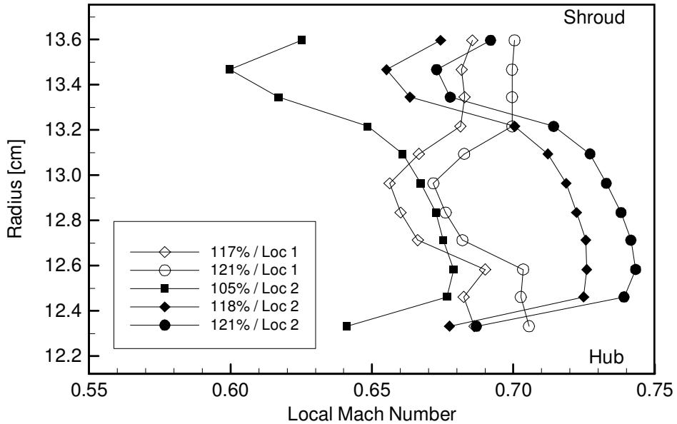
**Figure 4-20: Local Mach number radial profiles at different probe locations and different corrected speeds.**
