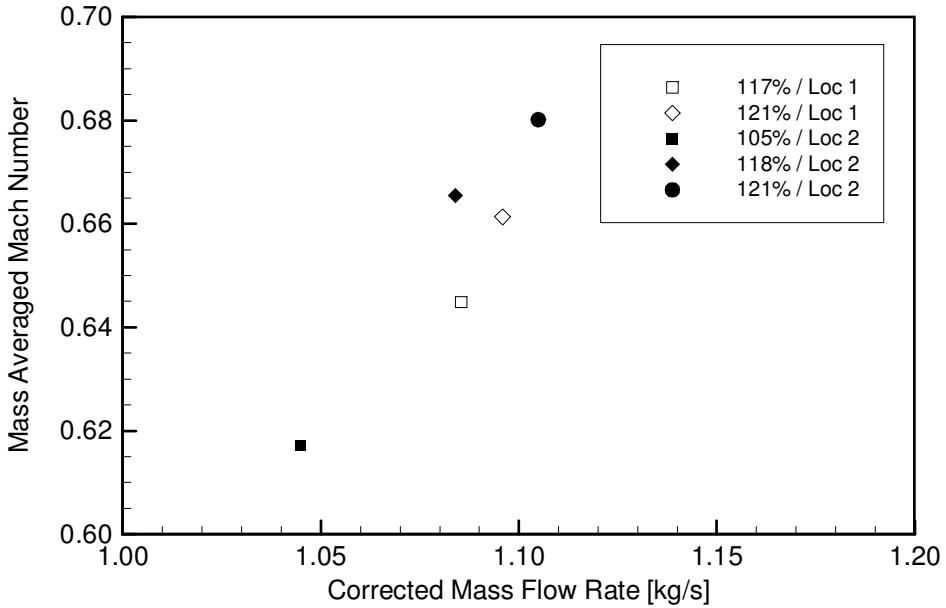
**Figure 4-21: Mass averaged Mach number at IGV exit probe location for each of the five surveys presented in the previous figure.**
