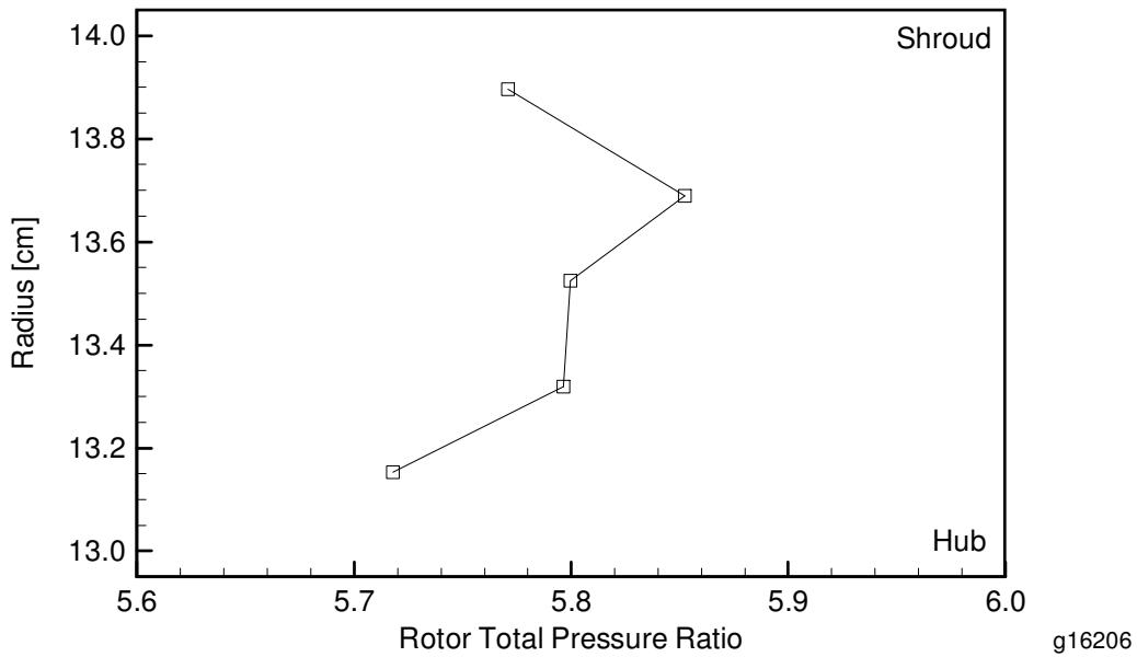
**Figure 4-31:** Radial variation of rotor total pressure ratio for a test at 120% corrected speed.
