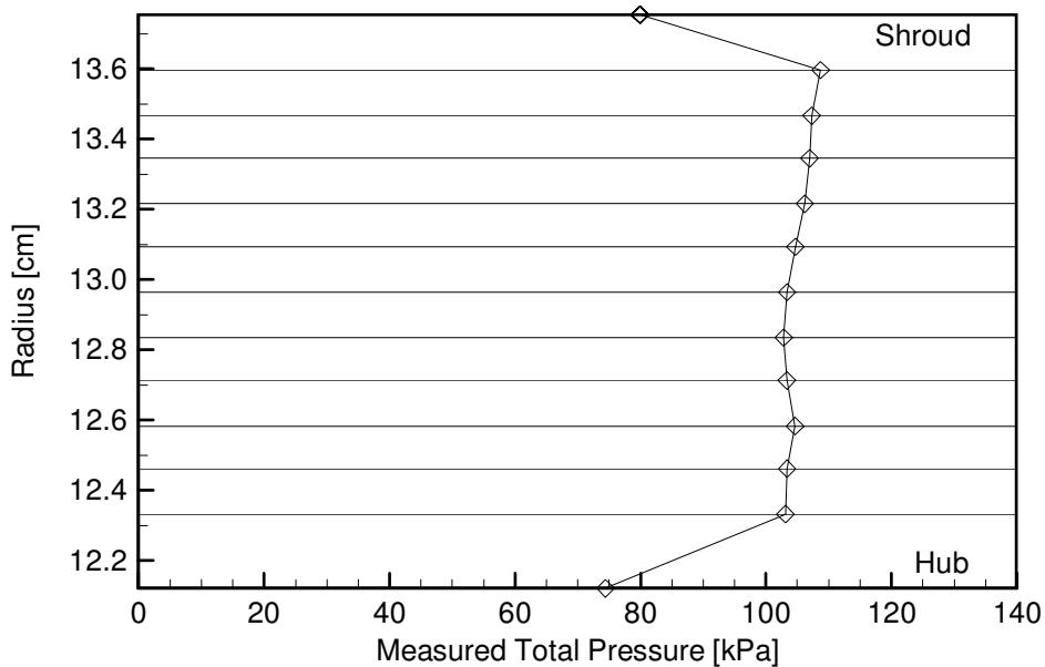
**Figure 4-19: Total pressure survey and stream tube boundaries.**
