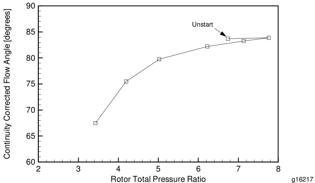
**Figure 4-35: Variation of centerline continuity corrected flow angle with total pressure ratio for run which achieved the highest total pressure ratio.**
