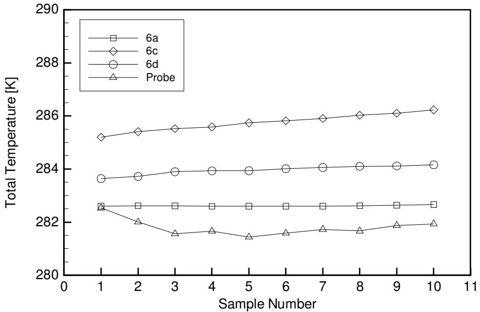
**Figure 4-11: Measured plenum total temperature during a typical high speed test with forward bleed. RTD 6c is directly downstream of a strut containing the forward bleed flow. The performance probe temperature is also shown.**
