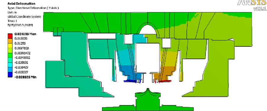
**DE diffuser attachment shows .020 in. of pressure generated variation.
