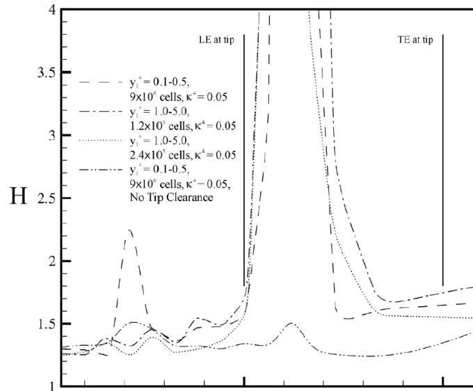
**Figure 3-30: Loss generation near stall, shroud boundary layer shape factor along passage centerline.**
