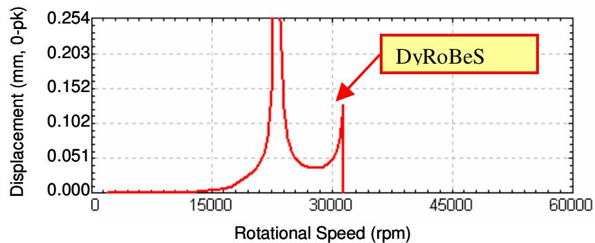
**Figure 2-6: Rotordynamic prediction with o-ring stiffness and damping corrected.**
