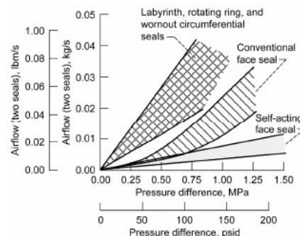
Figure 48.—Comparison of leakage characteristics for labyrinth, conventional (contact) face seal and self-acting face seals.<sup>109</sup>
