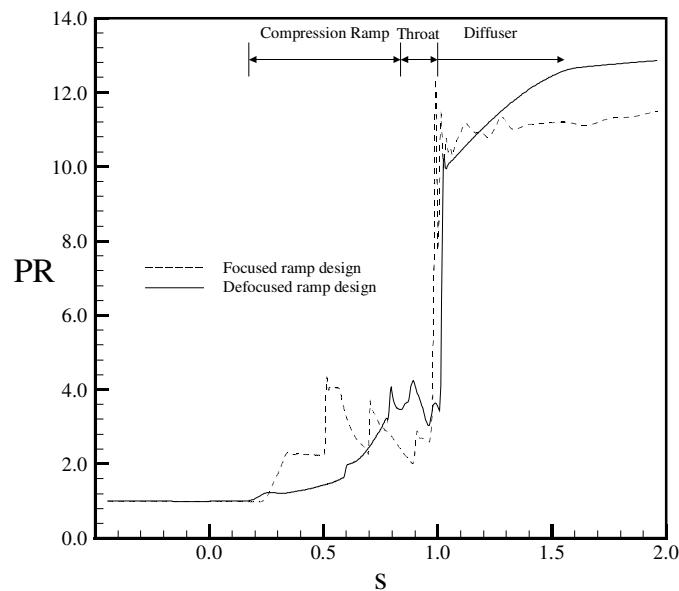
**Figure 3-35: Comparison of focused and defocused absolute centerline pressure ratio vs. normalized streamwise distance.**
