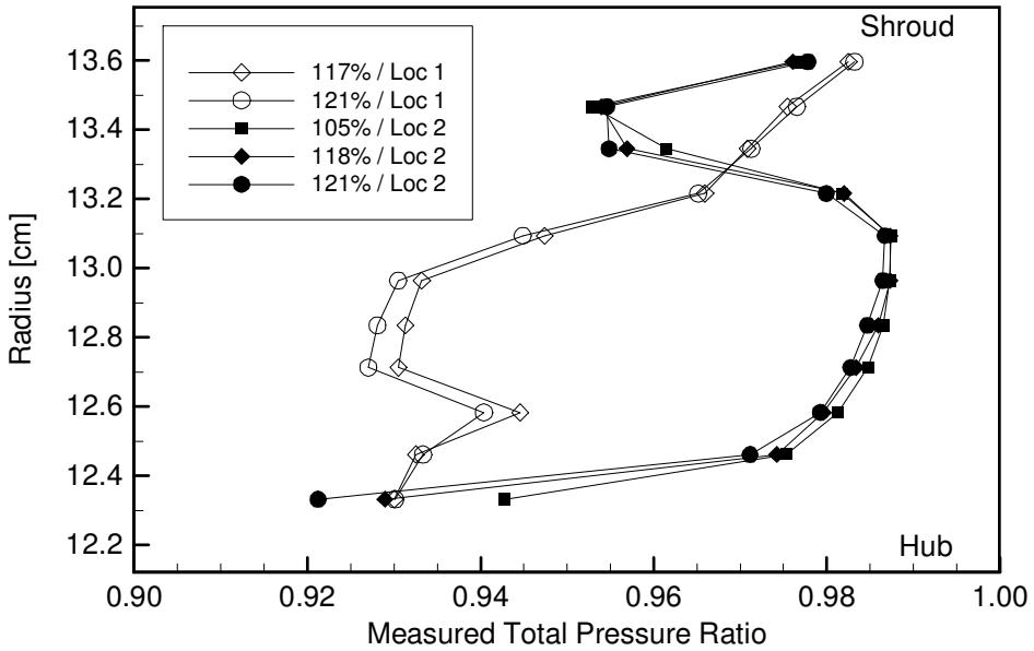
Figure 4-17: Radial surveys of total pressure ratio, IGV exit to plenum. Surveys were conducted at two circumferential locations and at three different corrected speeds.
