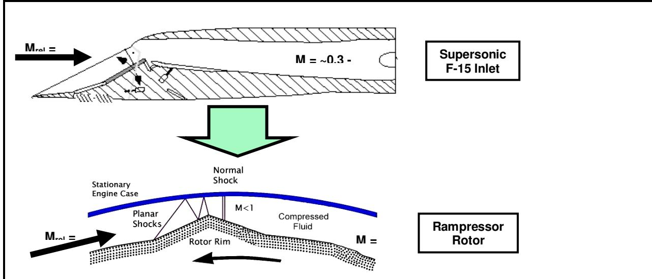
Figure 2.4.3 Rampressor Rotor Profile
