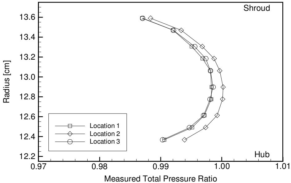
**Figure 4-6: Radial surveys of total pressure ratio, plenum to end of inlet, at three different circumferential locations at 107% corrected speed. The shroud and hub are at the top and bottom locations of the plot, respectively.**
