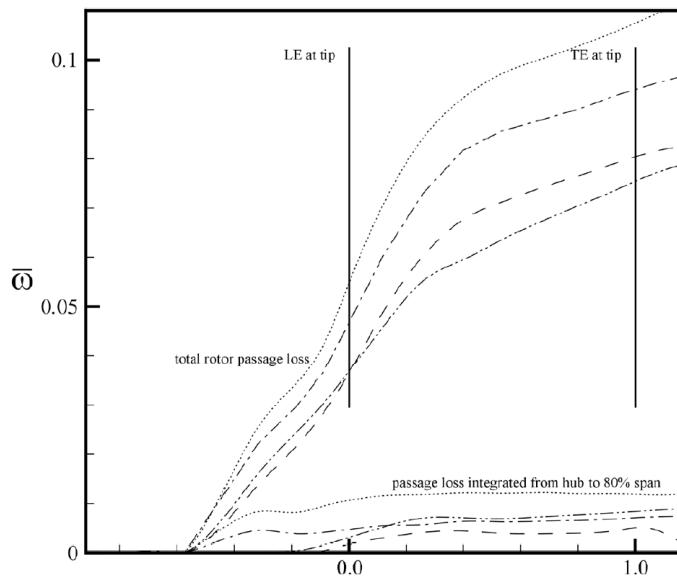
**Figure 3-31: Loss generation near stall, mass average relative total pressure loss along passage centerline.**
