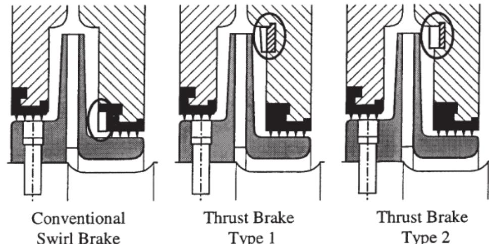
*Figure 5. Swirl and Thrust Brakes Used in High Pressure Compressors.*
