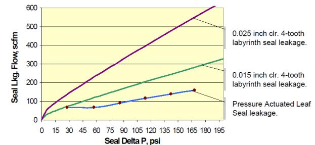
Figure 3. Pressure Actuated Leaf Seal Leakage Compared.
