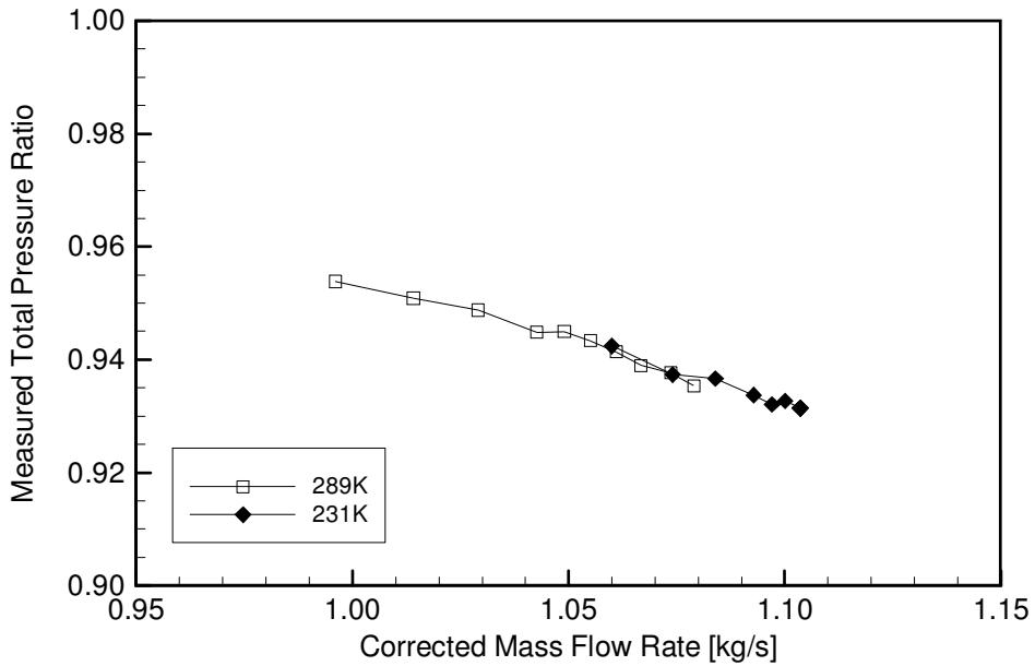
**Figure 4-15: Measured centerline total pressure ratio, IGV exit to plenum, at location 1.**
