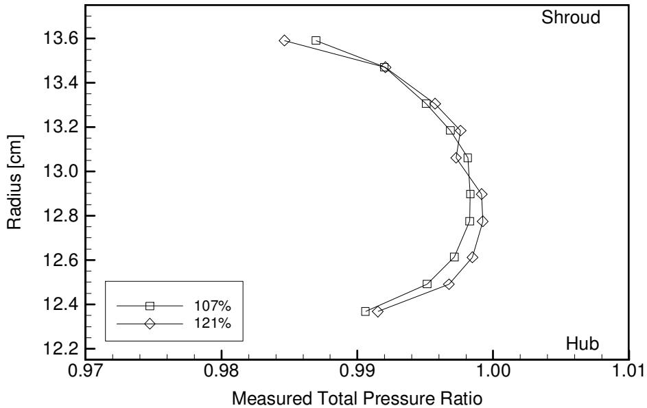
**Figure 4-7: Radial surveys of total pressure ratio, plenum to end of inlet, at circumferential location 1 for different rotor corrected speeds.**
