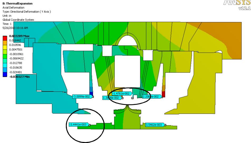
**Temperature only** effects tend to offset, over the discharge temperature range , with diffuser attachment point moving toward the midplane (-2.49e-002 and -1.48e-002) and case and shaft growth (-2.2e-002 + 0.73e-002 and -1.28e-002+0.34e-002).
