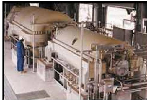
Figure 3.3 – Elliott Turbo Process Compressor Train
