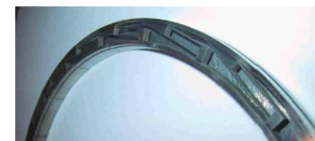
Figure 62.—Hydrodynamic brush seal (spring beam elements).<sup>142</sup>
