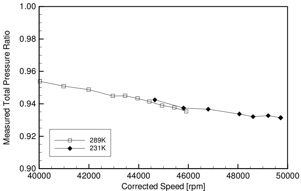
**Figure 4-16: Measured centerline total pressure ratio, IGV exit to plenum, at location 1.**
