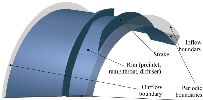
Figure 3-36: Computational domain used for viscous Rimpessor rotor simulations.
