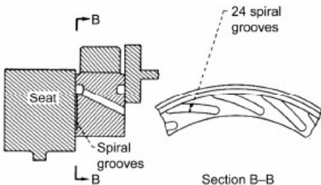
Figure 47.—Spiral groove sealing schematic.<sup>109</sup>
