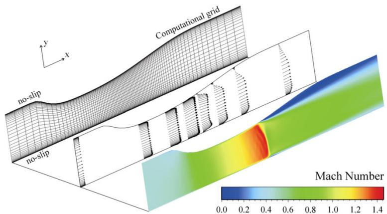
**Figure 3-14: Schematic of separating transonic diffuser flow and computational grid used in simulations.**
