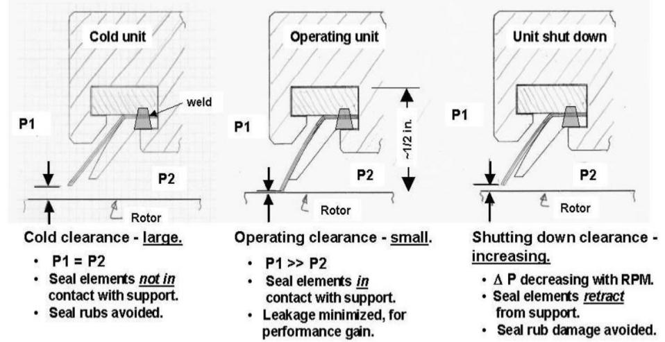
Figure 2. Pressure Actuated Leaf Seal Functional Characteristics.
