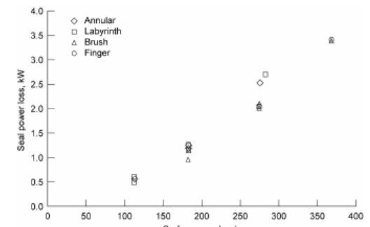
Figure 11.—Seal power loss for annular, 4-knife labyrinth, brush, and finger seals as a function of speed. Inlet air temperature = 700 K; Seal pressure differential = 276 kPa.
