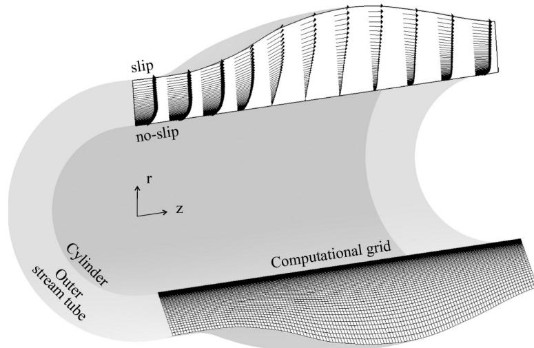
**Figure 3-5: Schematic of annular separating diffuser flow and computational grid used in simulations.**
