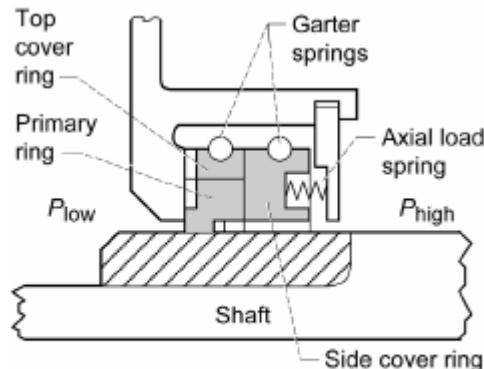
Figure 42.—Shaft riding or circumferential contact seal.<sup>104</sup>
