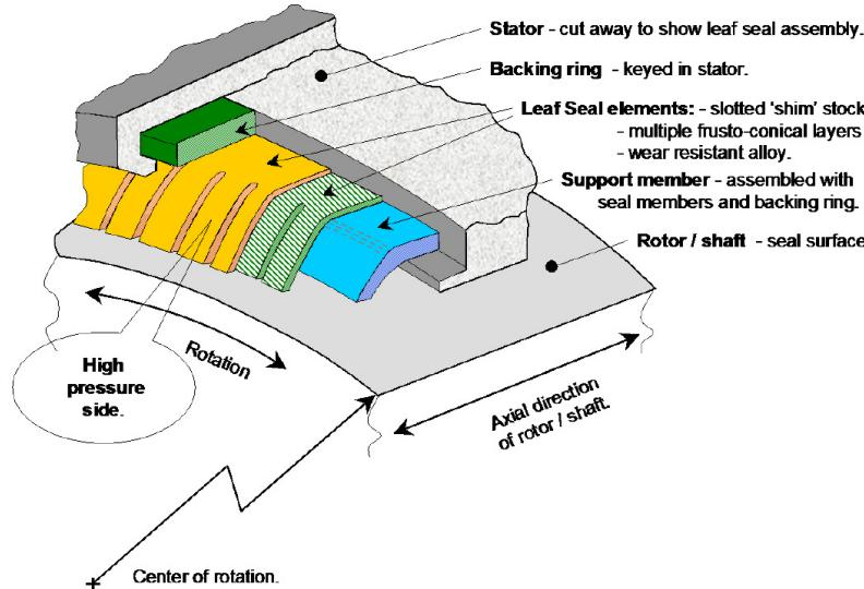
Figure 1. Pressure Actuated Leaf Seal Assembly.
