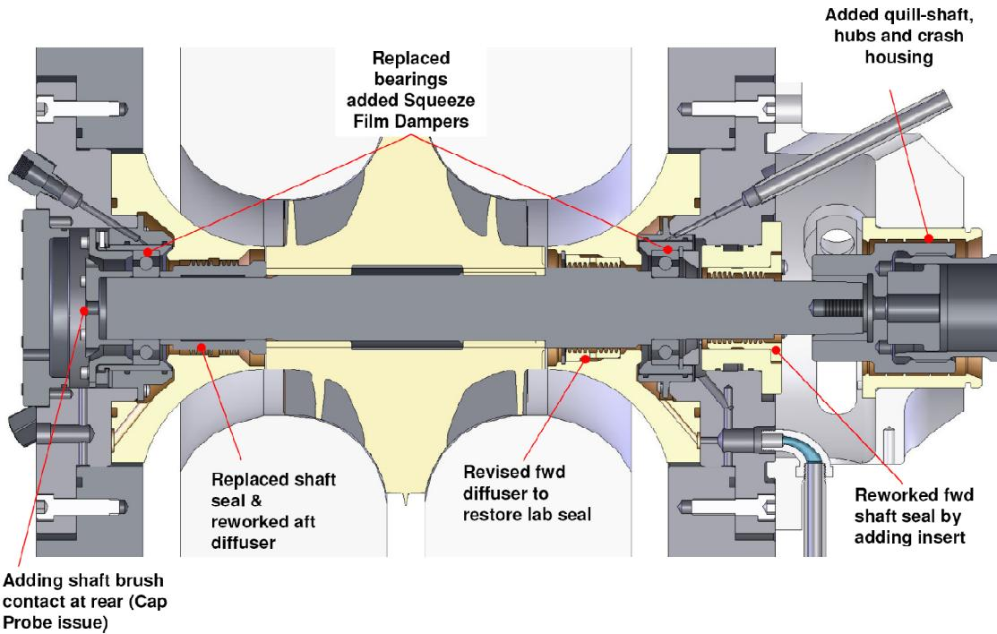
Figure 2-10: Section through the drive turbine final configuration.
