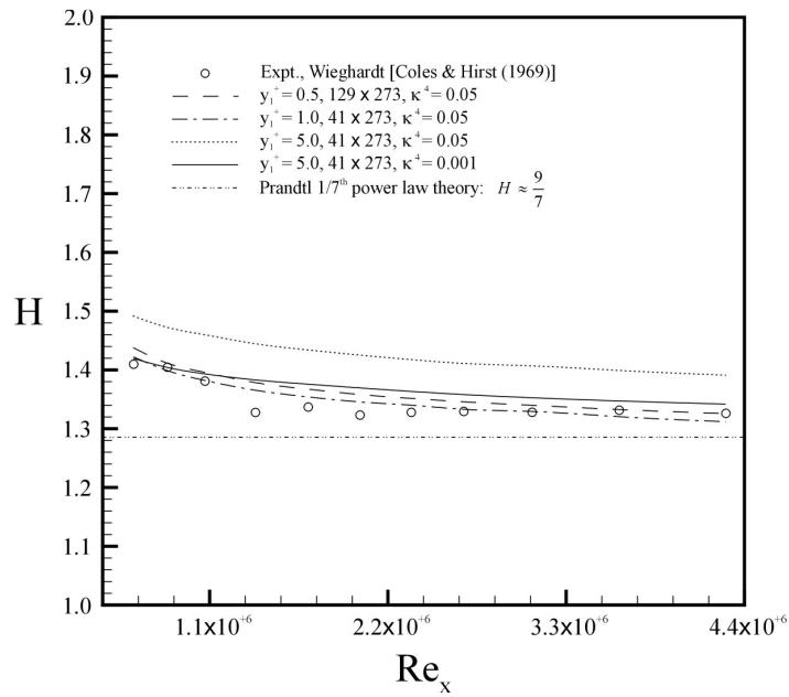
Figure 3-4: Flat plate shape factor prediction.
