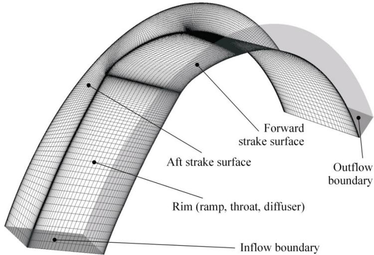
**Figure 3-32: Computational grid used for reduced flow path model. Note that all solid surfaces were set as slip surfaces.**
