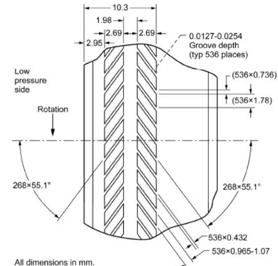
Figure 4.—Herringbone groove design.
