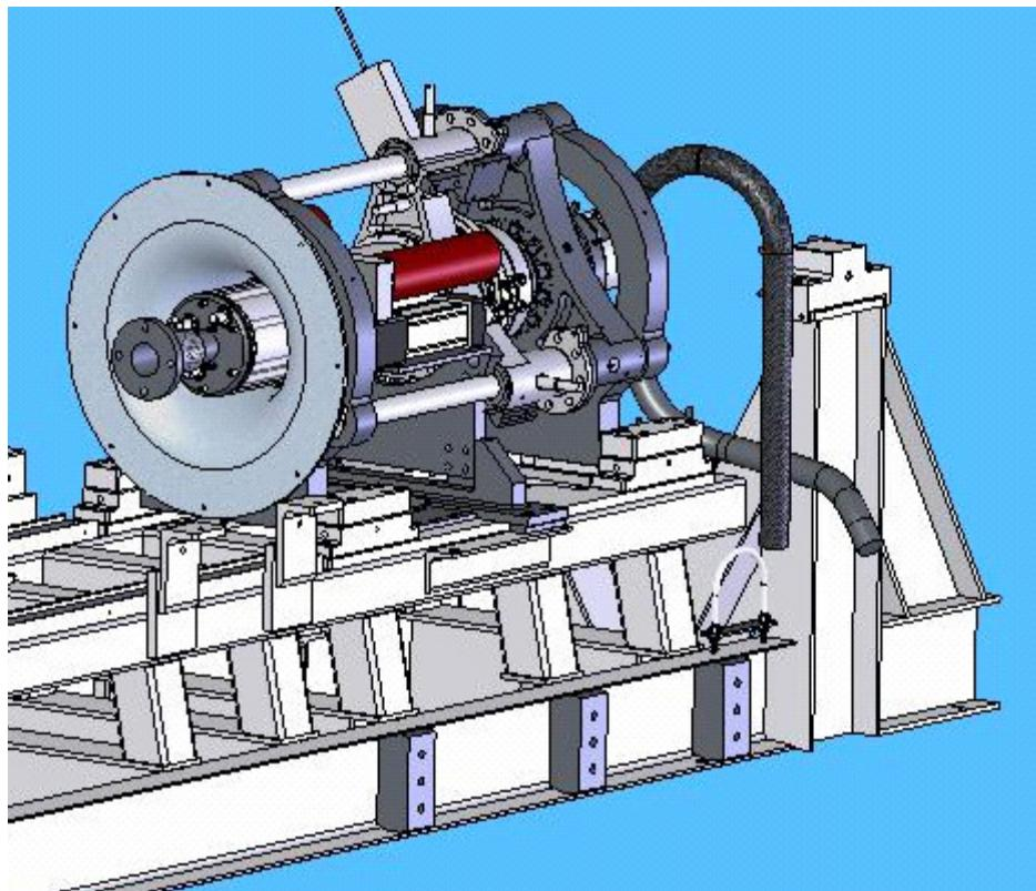
Figure 2-3: Forward end frame stiffness enhancement components as installed.
