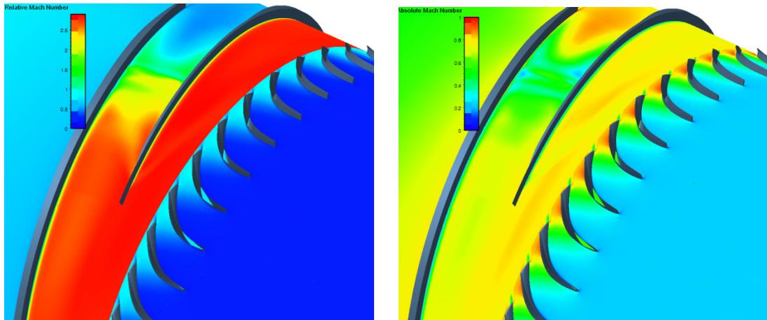
**Figure 3-51:** Results of IGV and rotor coupled modeling showing left) absolute and right) relative Mach number at rotor mid-span.
