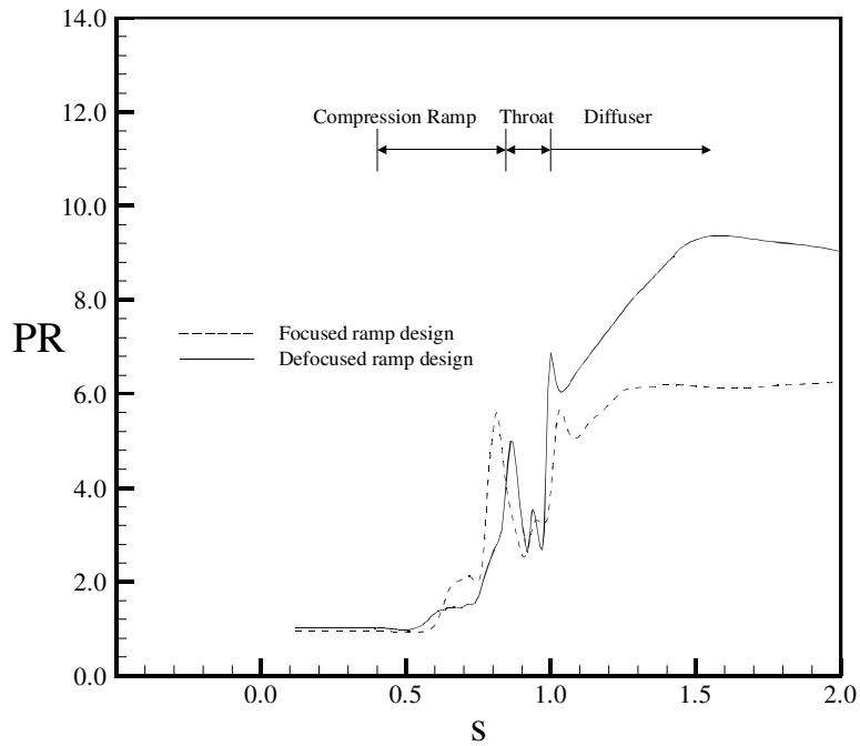
**Figure 3-40: Comparison of focused and defocused absolute centerline pressure ratio vs. normalized streamwise distance.**
