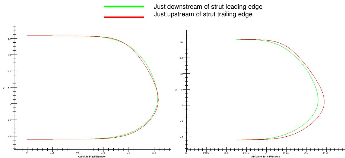
**Figure 3-46: Impact of strut on IGV performance. Left) Mach number and right ) total pressure pitchwise averaged profiles upstream and downstream of strut.**
