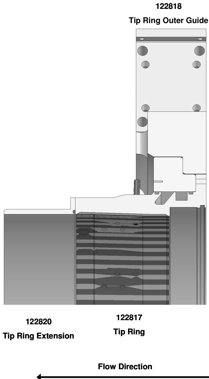
Figure 2-11: Section through tip ring assembly.
