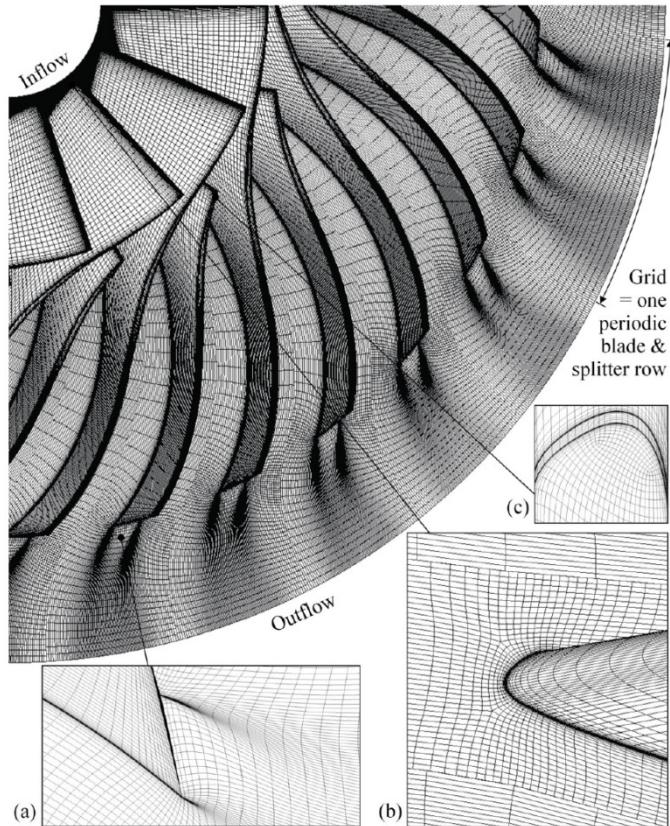
**Figure 3-11: Computational grid used for 4:1 centrifugal compressor simulations. The 3 million cell version is shown. Figure (a) shows the trailing edge at the hub. Figure (b) shows the leading edge at the hub. Figure (c) shows the tip clearance at the leading edge.**
