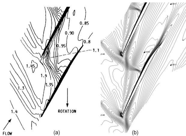
**Figure 3-24: Mach number contour prediction near stall for transonic fan rotor at 10% span from tip. Figure a shows the experimental results while figure b shows the cfd simulation results.**
