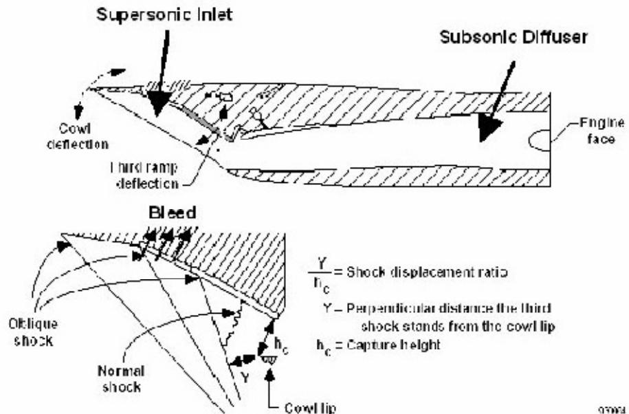
Figure 1-1: F-15 supersonic inlet cross section detail.
