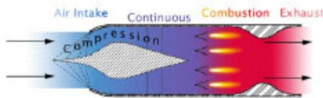
Figure 2.4.1. Ramjet Engine
