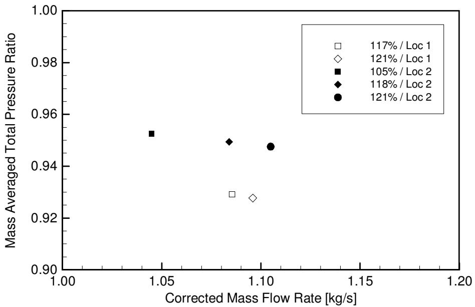
**Figure 4-18: Mass averaged total pressure ratio, IGV exit to plenum, for each of the five surveys presented in the previous figure.**
