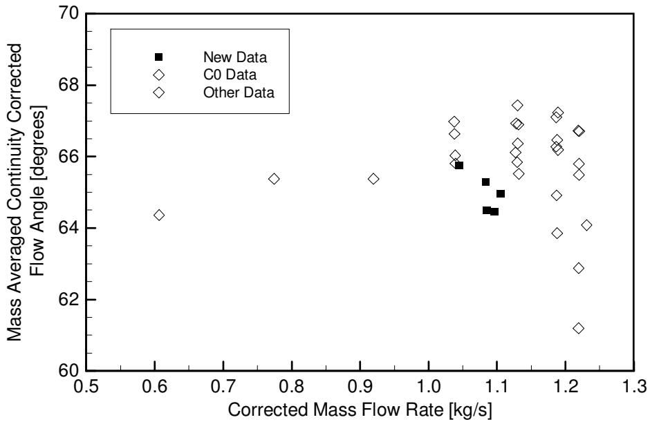
**Figure 4-27:** Calculated mass averaged continuity corrected flow angle at IGV exit probe location. The solid symbols represent new data discussed in this section while the open symbols are data from previous measurements reported by Williams (2007). The new data are in general agreement with previous measurements.
