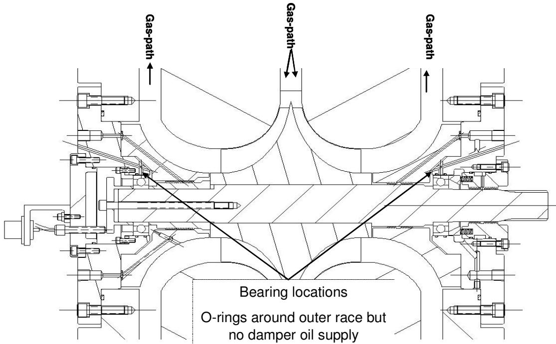
Figure 2-9: Section through the drive turbine original configuration.
