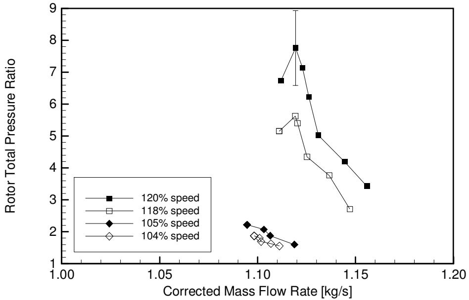
**Figure 4-29: Variation of corrected mass flow rate with total pressure ratio and the effect of corrected speed. The drop in total pressure ratio and corrected mass flow rate due to unstart can be seen in the two high speed cases.**
