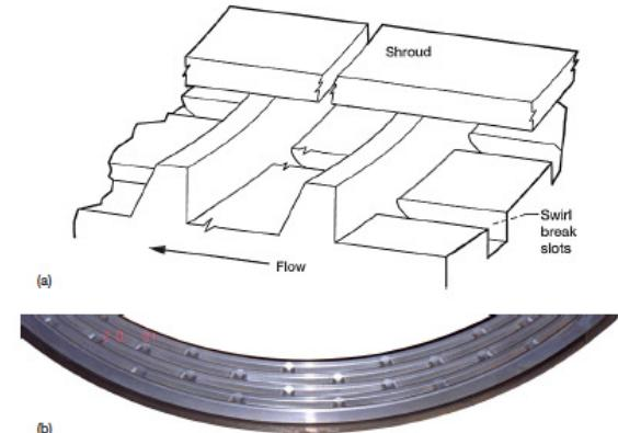
Figure 52.—Web seal. (a) Sketch of conceptual web seal. (b) Photograph of web seal or slotted labyrinth seal. (Camatti et al., 2003.) Courtesy ISORMA-2.
