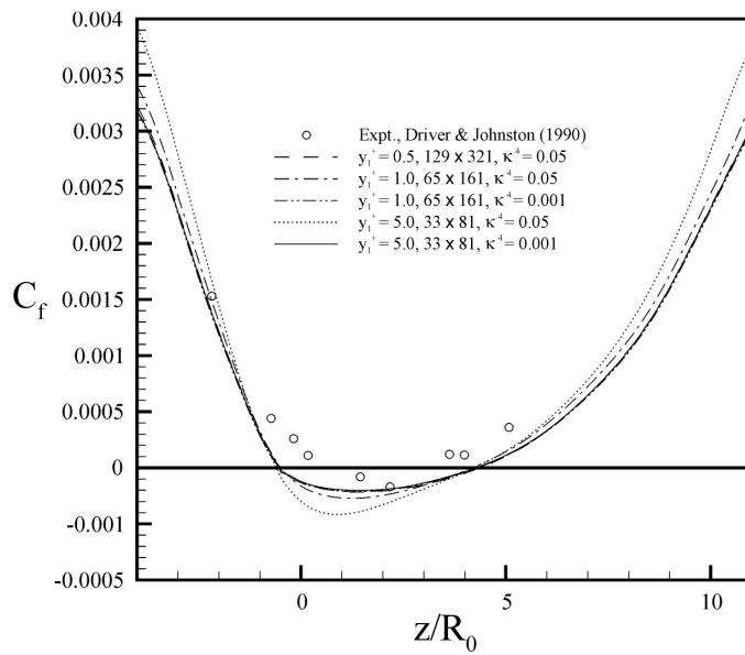
**Figure 3-8: Annular separating diffuser skin friction prediction.**
