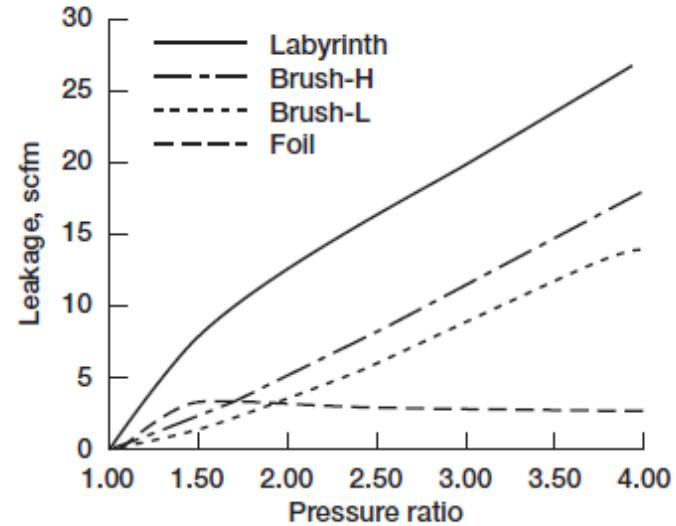
Figure 35.—Seal leakage comparison. (Munson et al., 2002.) Courtesy Rolls-Royce/Allison.
