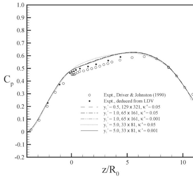
**Figure 3-7: Annular separating diffuser static pressure coefficient prediction.**
