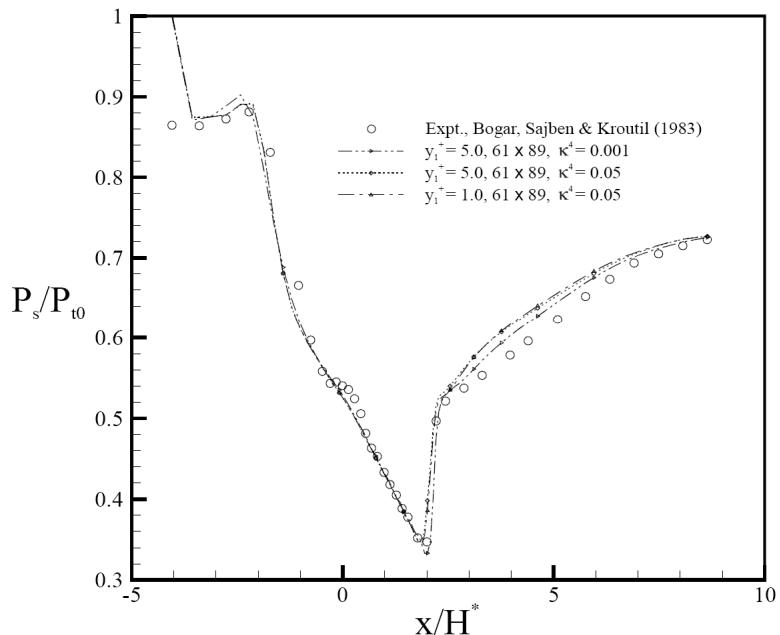
**Figure 3-15: Predicted static pressure for separating transonic diffuser.**
