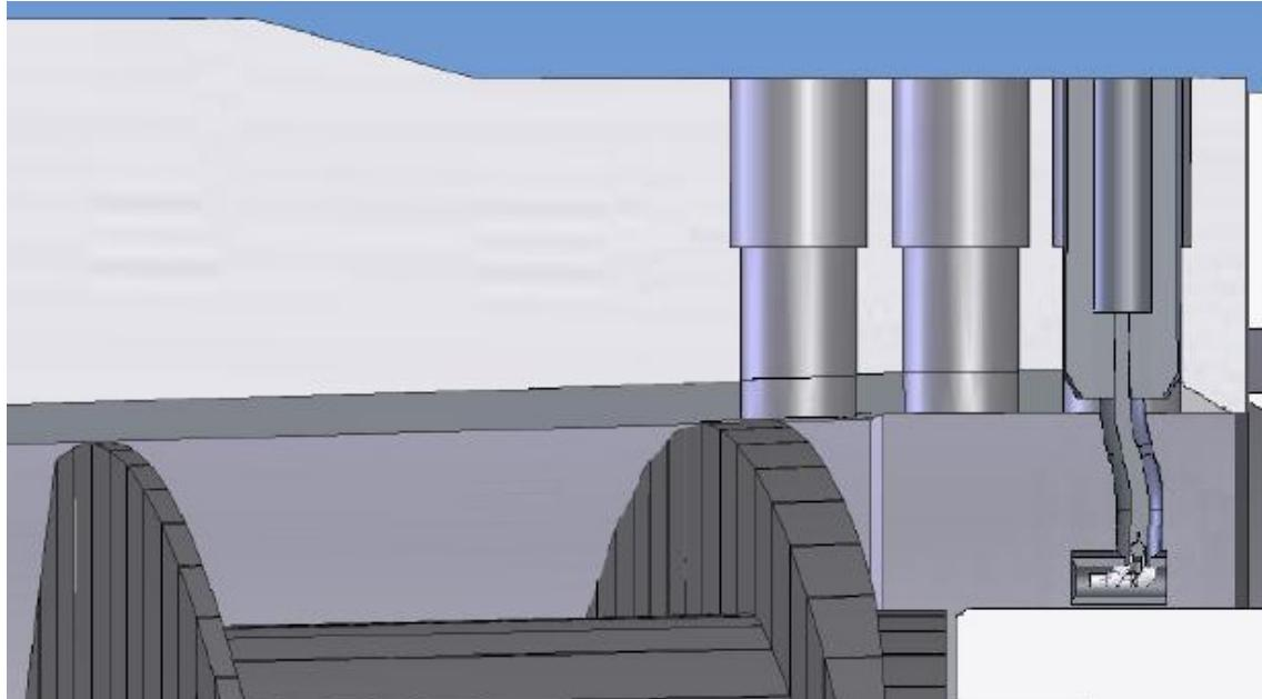
**Figure 4-28: Location of the performance probe relative to the rotor.** The performance probe could be positioned vertically in the flow path for radial surveys. Here it is shown positioned near the hub. The tip gap was adjusted by sliding the tip ring axially which also moved the performance probe relative to the rotor exit.
