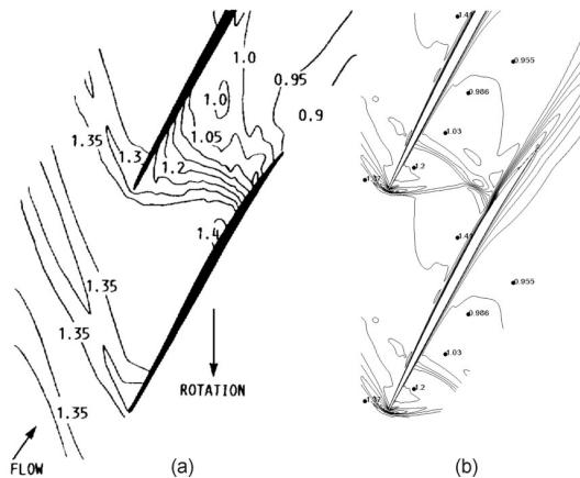
**Figure 3-23: Mach number contour prediction near peak efficiency for transonic fan rotor at 10% span from tip. Figure a shows the experimental results while figure b shows the cfd simulation results.**
