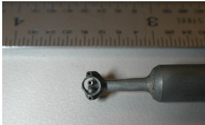
**Figure 4-1:** Performance probe used to measure inlet performance. The total pressure and total temperature probes are in the shroud and the nulling channels are outside the Kiel shroud. The outside diameter of the Kiel shroud was 3.18 mm (0.125 inches), and the outside diameter of the total pressure probe was 0.82 mm (0.032 inches).
