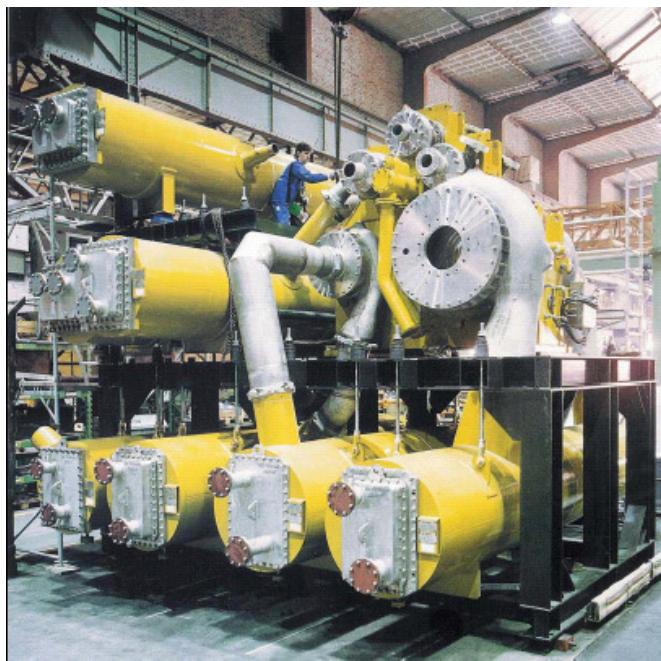
Figure 3.2 – MAN Turbo 10-stage 200:1 CO<sub>2</sub> Compressor
