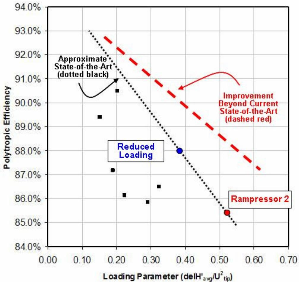
Figure 1: Compressor efficiency vs. stage loading
