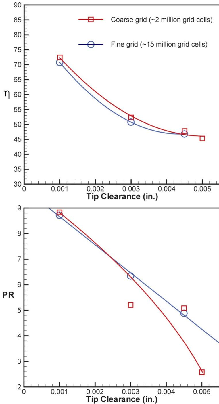
Figure 3-52: Rotor performance prediction sensitivity to grid resolution.
