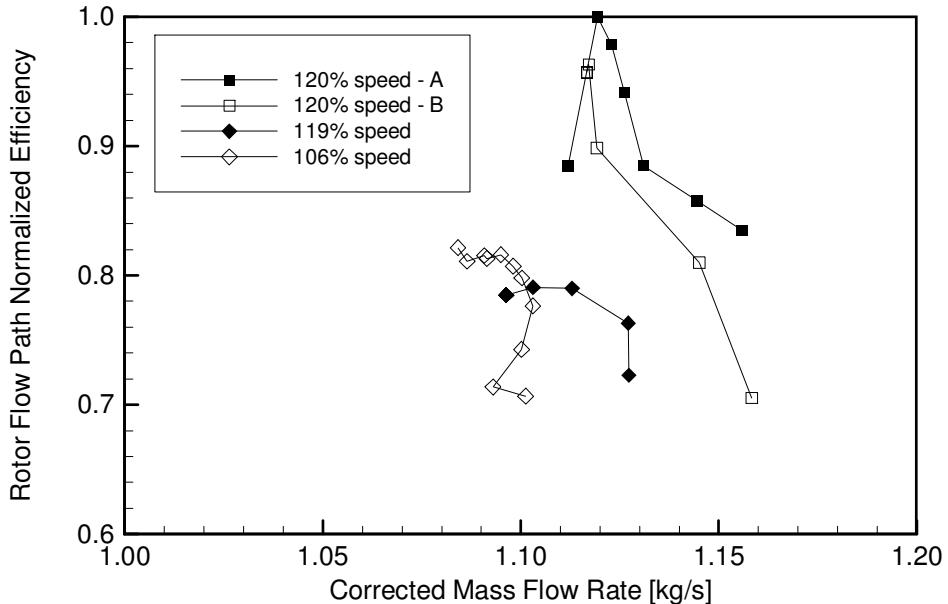
**Figure 4-33: Effect of tip gap on normalized efficiency.** The speed lines shown are the same as in Figure 4-30. See text for details on tip clearance for each speed line.
