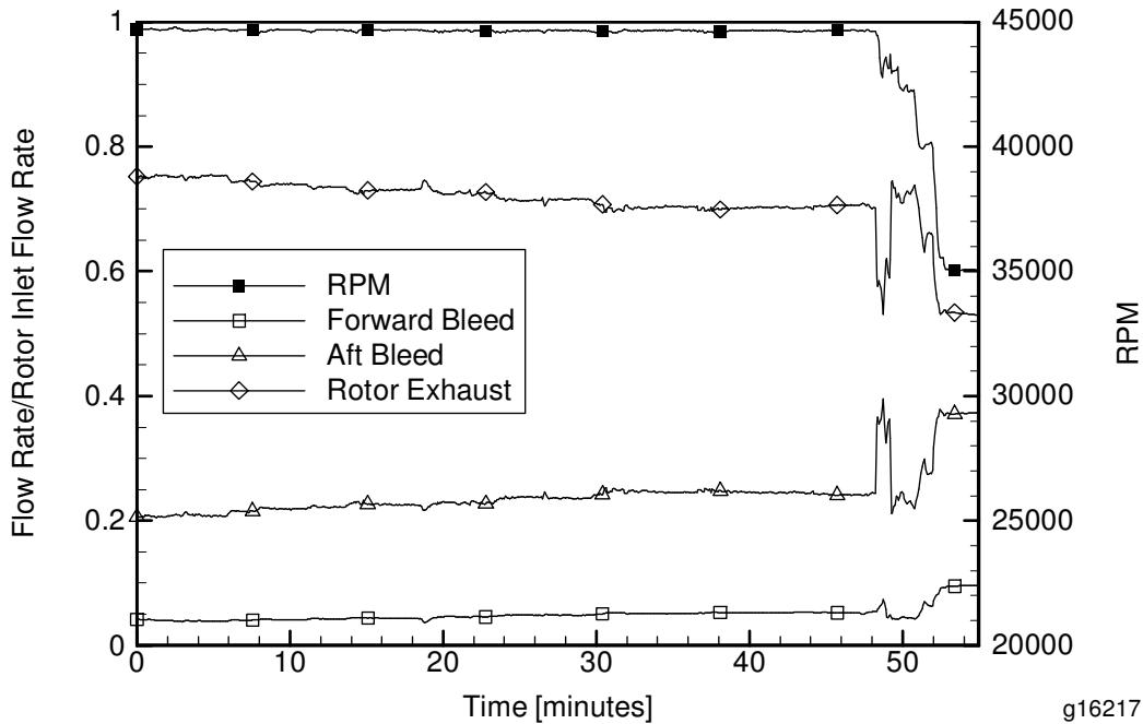
**Figure 4-5: Adjusted bleed and exhaust mass flow rates as a fraction of the rotor entrance flow.**
