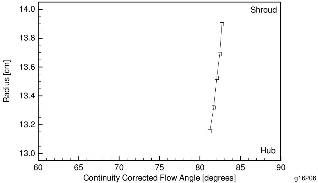
**Figure 4-36: Variation of continuity corrected flow angle with radius for the survey shown in Figure 4-31.**
