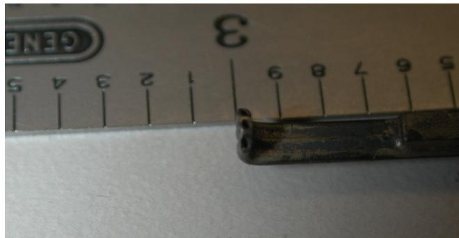
**Figure 4-2:** Cobra probe used to characterize inlet performance. Total pressure was measured at the center tube while the two side tubes provide nulling channels. The outside diameter of the total pressure probe was 0.82 mm (0.032 inches).
