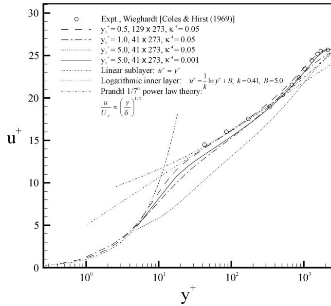
**Figure 3-2: Flat plate boundary layer profile prediction at approximately mid-plate location.**
