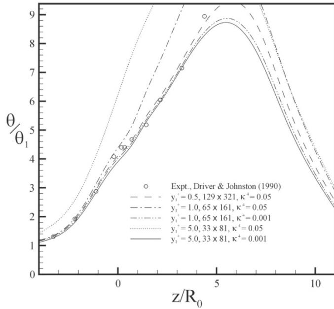
Figure 3-9: Annular separating diffuser momentum thickness prediction.
