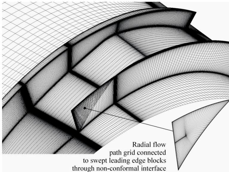
**Figure 3-49: Rotor grid generated using IGG.**
