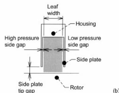
Figure 58.—Leaf seal configuration parameters. (a) Front view. (b) Side view.<sup>138</sup>
