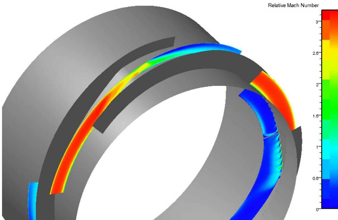
**Figure 3-53: Midpitch Mach number from Run 217 CFD simulation with 0.001 inch tip clearance.**
