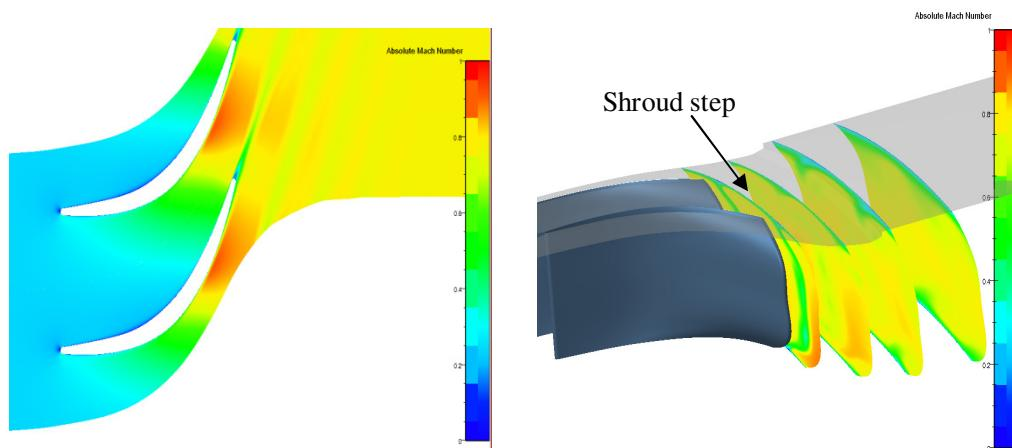
**Figure 3-43: Inlet guide vane blade to blade and exit plane Mach number distributions.**
