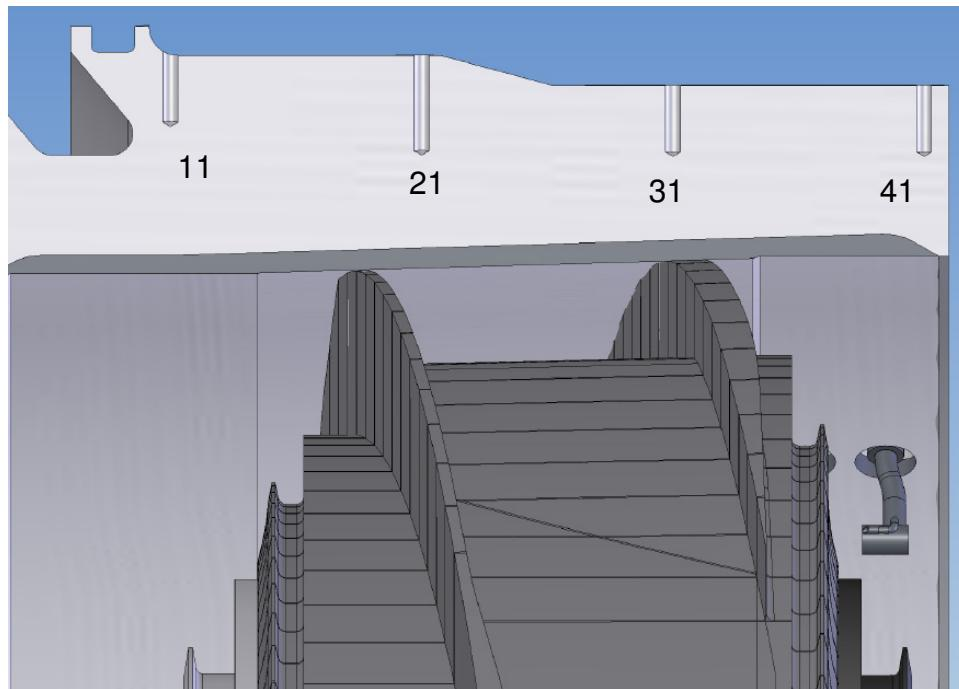
**Figure 4-3: Location and numbering convention of tip ring thermocouples.** Air flows from left to right. There is a large cooling passage on the upper left end of the tip ring. The dark gray area on the inside diameter of the tip ring is abradable. Tip ring and rotor relative positions match the test configuration for the data shown in Figure 4-4.
