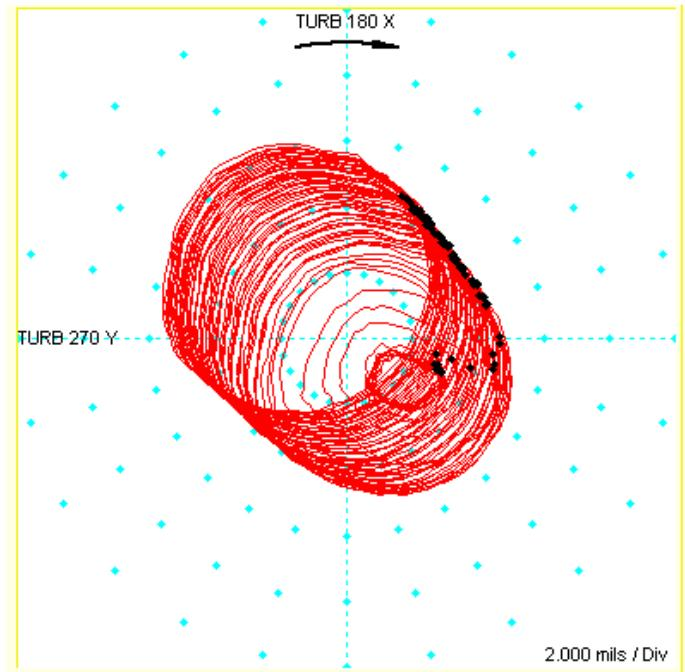
Figure 2-8: Run 65a - Sudden turbine shaft orbit increase.
