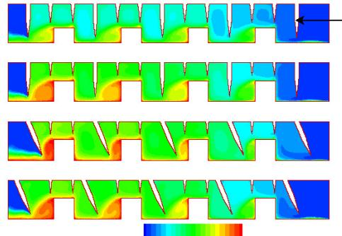
Figure 11. Axisymmetric swirl velocity in different designs ( $P_1/P_{14} = 10$  – CFD)
