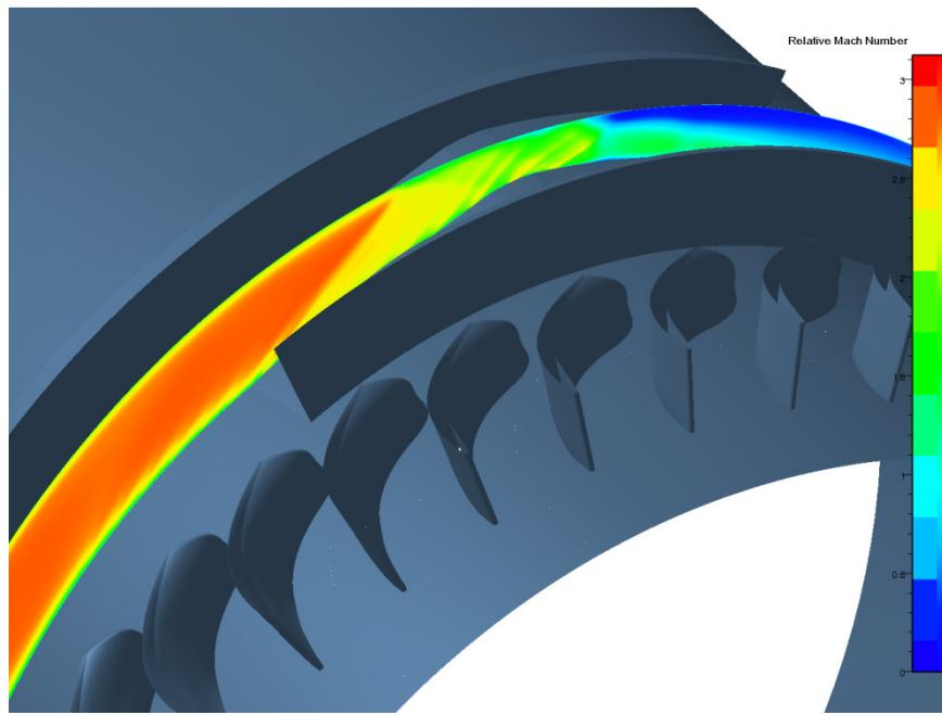
**Figure 3-50:** Results of IGV and rotor coupled modeling showing relative Mach number at rotor mid-pitch.
