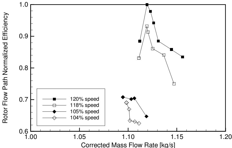
**Figure 4-32: Relationship between corrected mass flow rate and normalized efficiency and the effect of corrected speed. The drop in efficiency and corrected mass flow rate due to unstart can be seen in the two high speed cases. The speed lines shown are the same as in Figure 4-29.**
