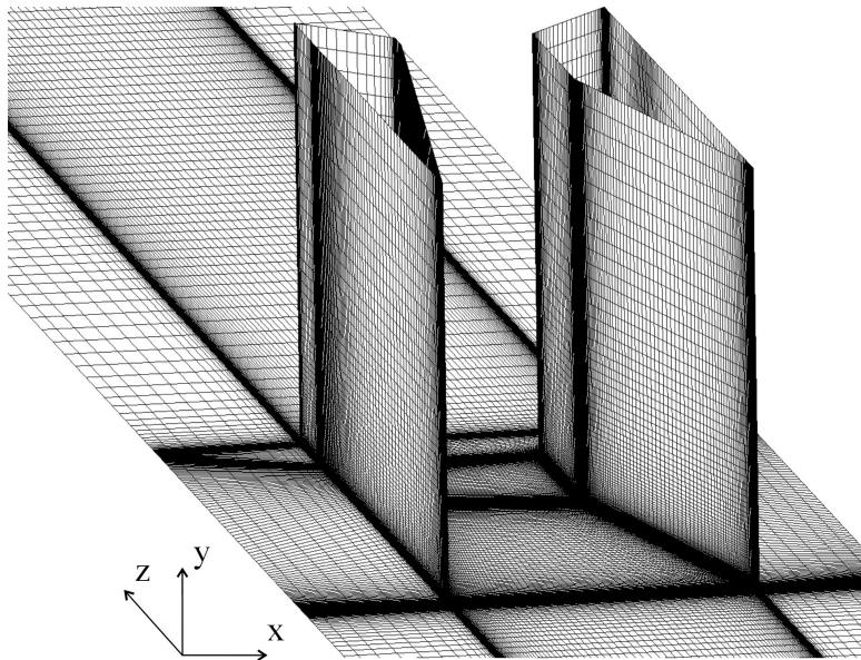
**Figure 3-17: Asymmetric crossing shock wave flow computational grid used in simulations. The finest resolution is shown in this image.**
