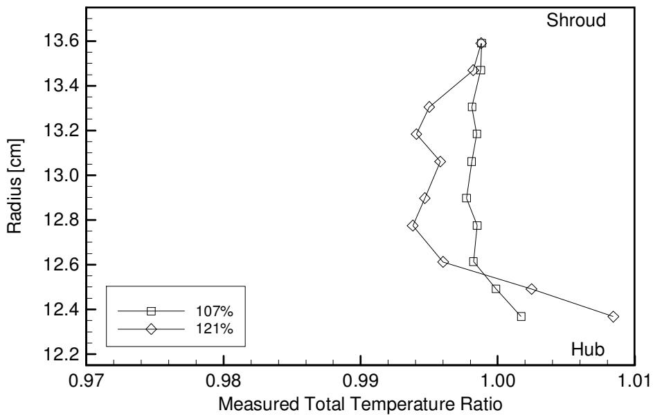
**Figure 4-14: Radial surveys of total temperature ratio, bellmouth to end of inlet, at circumferential location 1 for different rotor corrected speeds. In order to obtain 121% speed, liquid nitrogen was introduced into the main air to reduce the plenum temperature to approximately 230°K (-45°F).**
