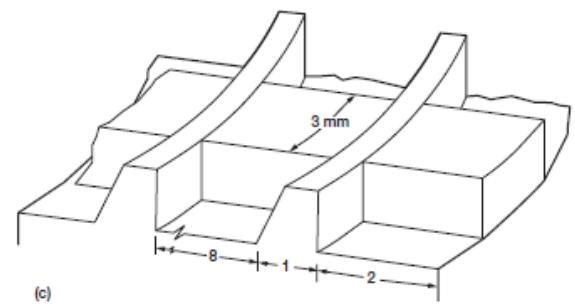
Figure 43.—Configuration of test seal. (a) Annular seal. (b) Labyrinth seal. (c) Flow blockers. Dimensions in millimeters. (Kanki et al., 2003.) Courtesy ISORMA-2.
