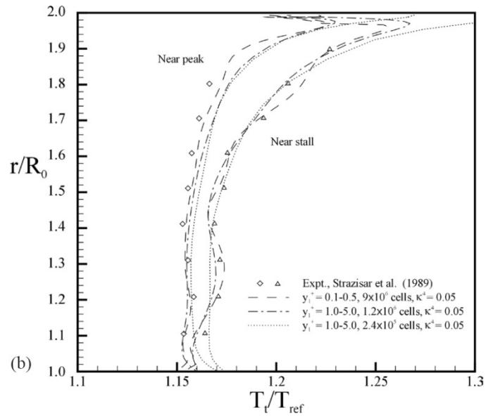
Figure 3-28: Transonic fan rotor flow predicted total temperature ratio profile.
