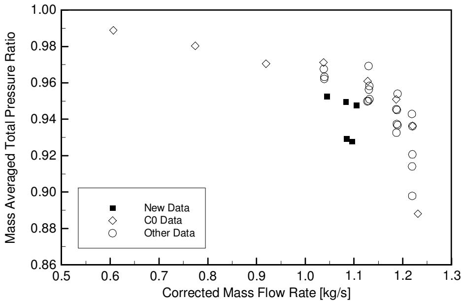
**Figure 4-24: Calculated mass averaged total pressure ratio from plenum to post-IGV probe location. The solid symbols represent the new data discussed in this section while the open symbols are the data from previous measurements reported by Williams (2007). The new data are in general agreement with previous measurements.**
