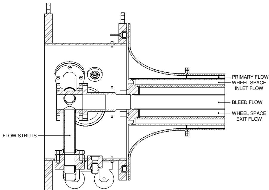
**Figure 4-10: Schematic of Rampressor inlet side flow passages.**
