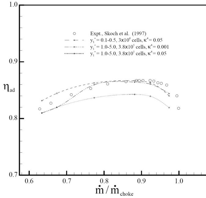
**Figure 3-13: Predicted adiabatic efficiency for 4:1 centrifugal impeller at 100% speed.**
