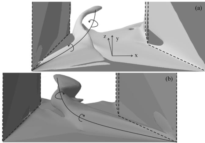
**Figure 3-19: Shock induced separation prediction using iso-surfaces of (a) negative vorticity and (b) positive vorticity.**
