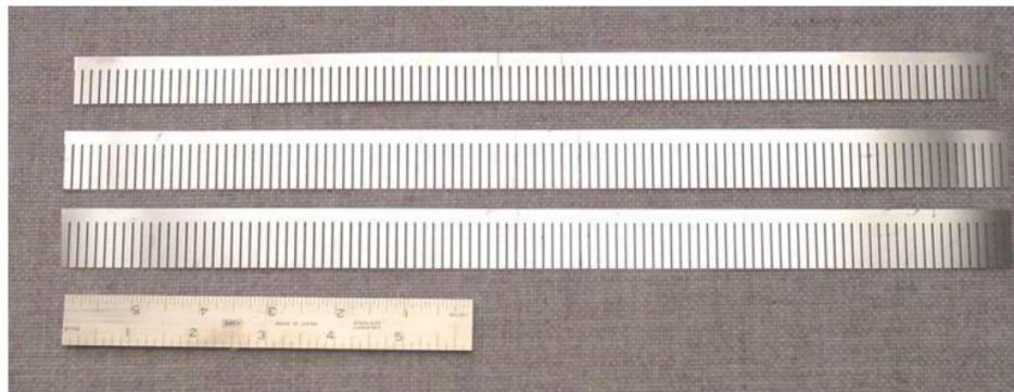
Figure 11. 3-D Strip Cut Seal Leaves.
