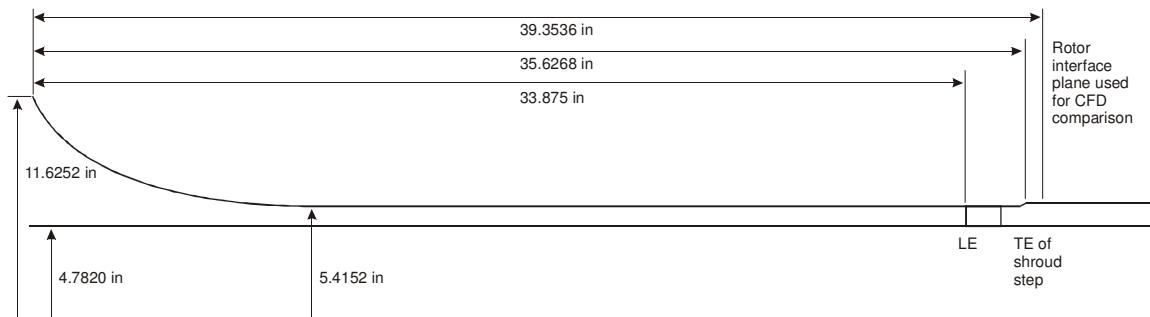
**Figure 3-41: Bellmouth and annulus leading to inlet guide vanes.**
