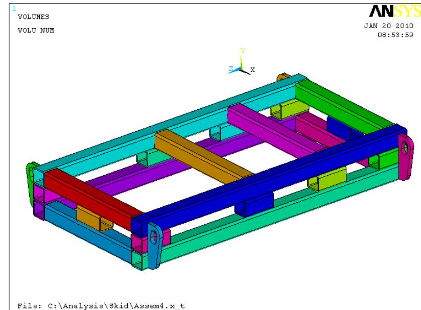
Assumption – spreader bar is being used so that loads are mostly vertical on the lifting lugs
