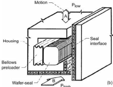
Figure 57.—Basic elements of leaf and wafer seals. (a) Leaf-seal.<sup>137</sup> (b) Wafer-seal.<sup>139</sup>
