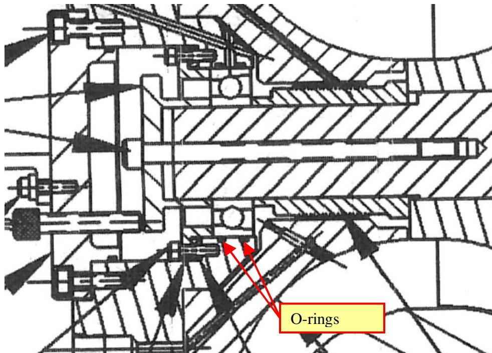
Figure 2-4: Original drive turbine bearing damper configuration.
