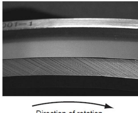
Fig. 6 Structure of leaf seal
