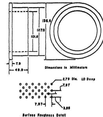
Figure 6(c). Round-hole pattern stator insert.
