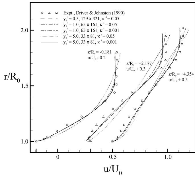
Figure 3-6: Annular separating diffuser boundary layer profile prediction.
