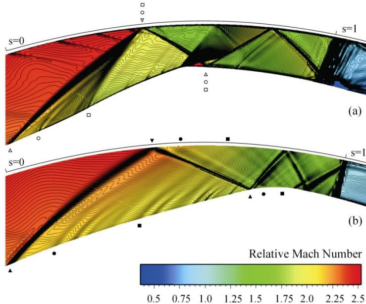
**Figure 3-33: Reduced model comparison of the relative Mach number of (a) focused and (b) defocused ramp designs. Symbols indicate three representative oblique shock initiation and reflection points.**
