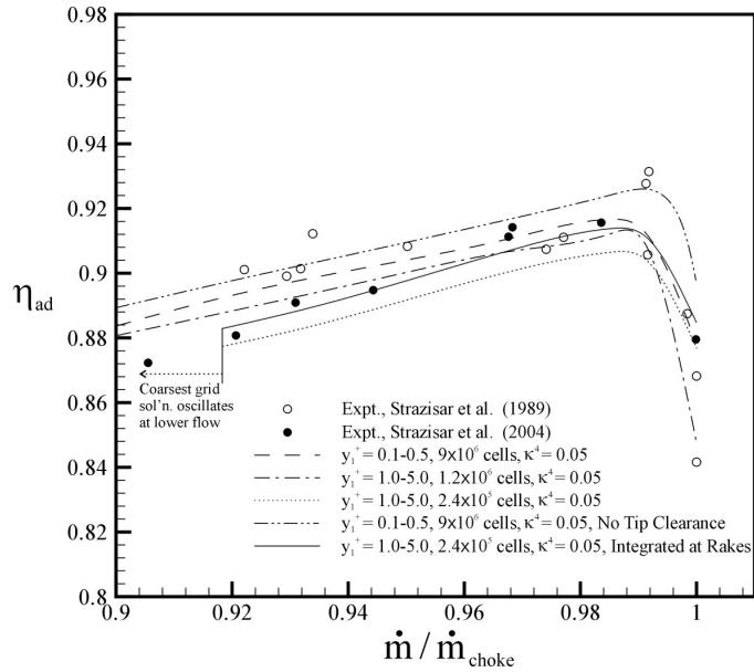
Figure 3-26: Transonic fan rotor flow simulation predicted efficiency.
