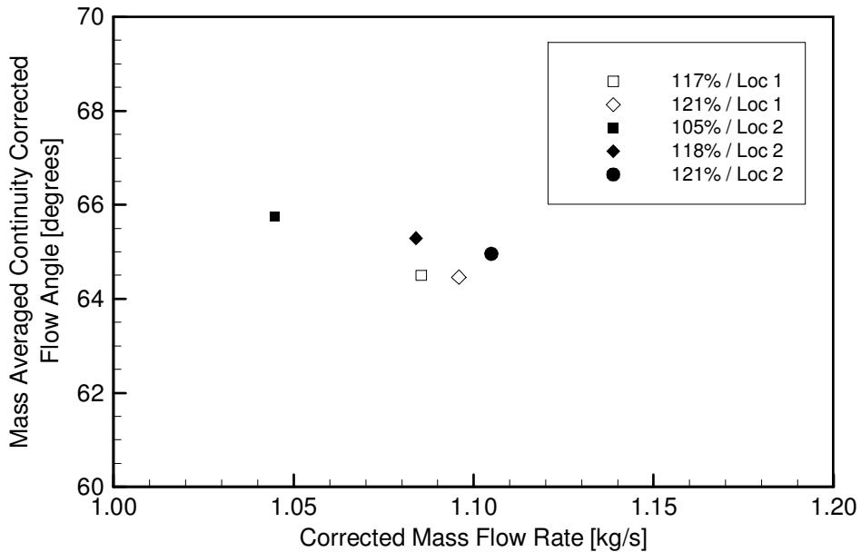
**Figure 4-23: Mass averaged continuity corrected flow angle at IGV exit probe location for each of the five surveys presented in the previous figure.**
