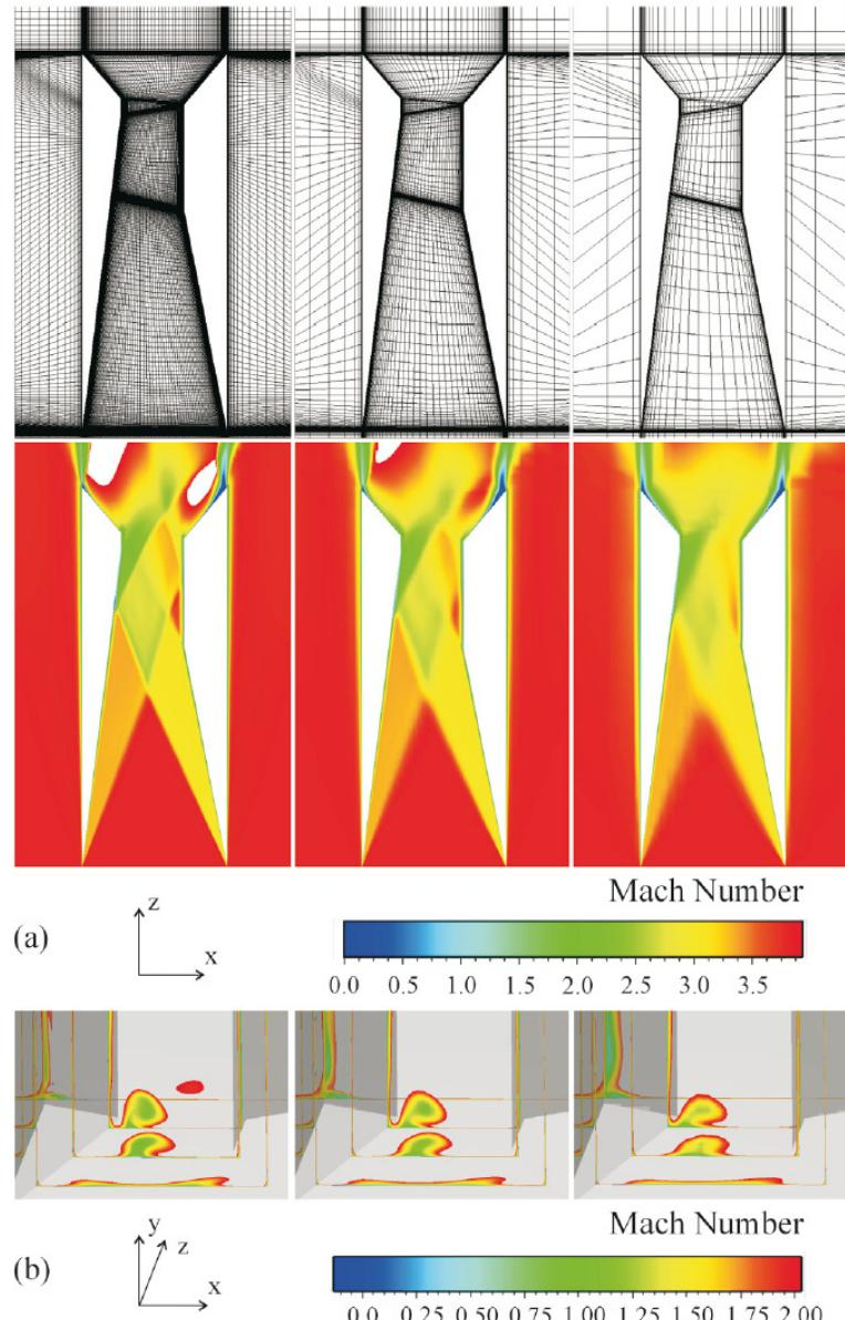
**Figure 3-18: Asymmetric crossing shockwave flow sensitivity of shock structure prediction to grid resolution. Figure a shows the Mach number at midspan while figure b indicates streamwise vortex production. The finest to coarsest grids are from left to right.**
