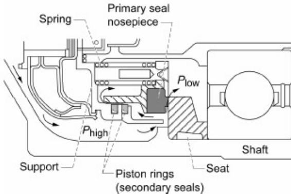
Figure 43.—Positive contact face seal.<sup>105</sup>
