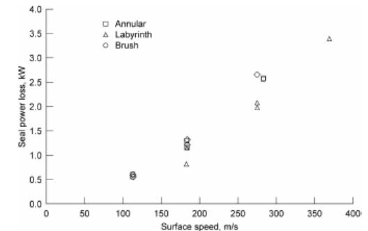
Figure 10.—Seal power loss for annular, 4-knife labyrinth and brush seals as a function of speed. Inlet air temperature = 297 K; Seal pressure differential = 276 kPa.
