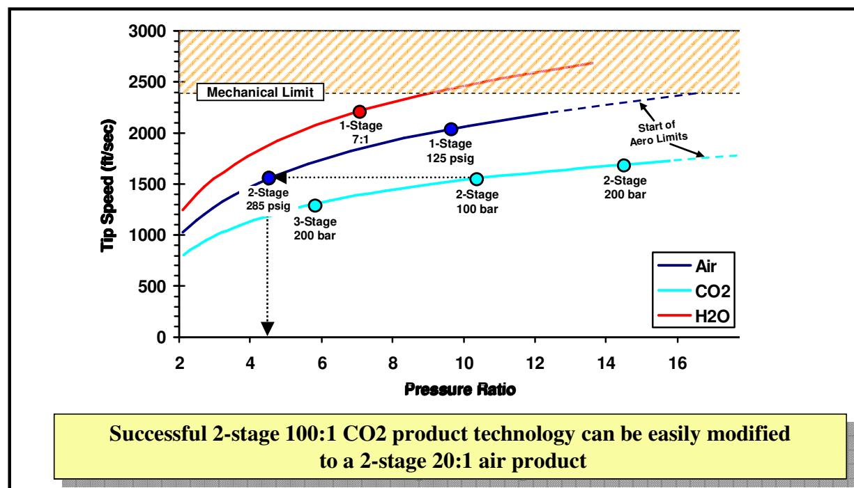
Figure 4.1 – Tip Speed vs. Pressure Ratio for Three Gases
