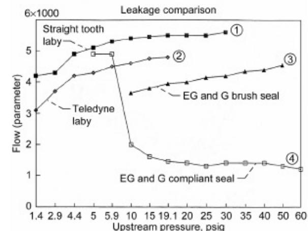
Figure 60.—Leaf-seal leakage comparison with labyrinth and brush seals.<sup>140</sup>
