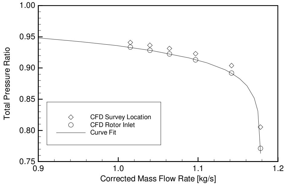
**Figure 3-47: CFD prediction of the total pressure loss between the bellmouth inlet and a location downstream of the IGV. The capture plane is at the rotor inlet while the survey plane is upstream at the location where measurements were taken.**
