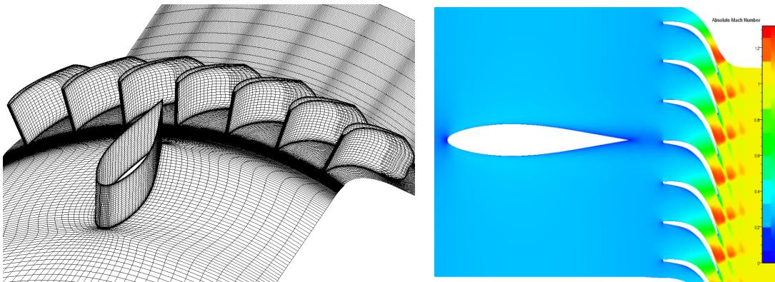
**Figure 3-45: Impact of strut on IGV performance. Left) grid used in CFD analysis and right) Mach number of mid-span blade to blade flow.**
