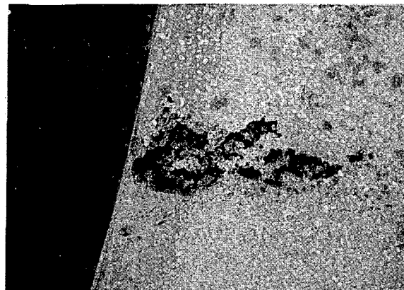
Figure 8 Corrosion from contact with wet foam
