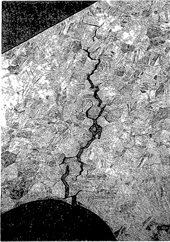
Figure 2. Cross section of intergranular fillet crack.
