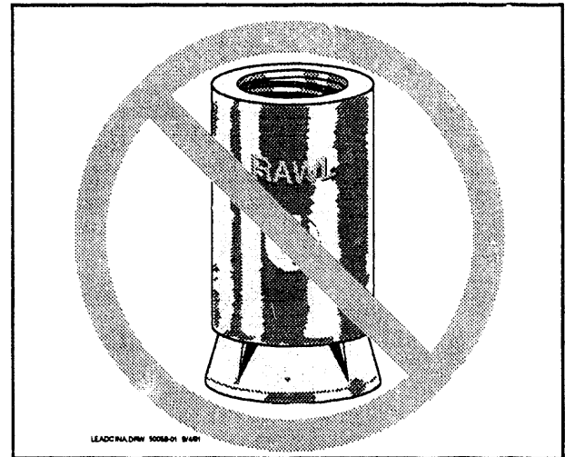
Figure 9-3: Lead cinch anchors have lower capacity
