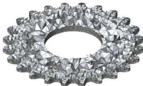
Figure 8: A cut through the volume mesh of a gear. The mesh has 6870 vertices, 7084 boundary faces, and 22456 tetrahedra.
