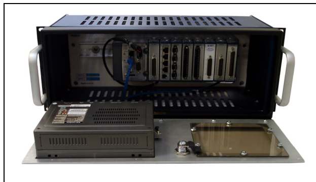
Figure 2: Wire Scanner System BiRIO Chassis
