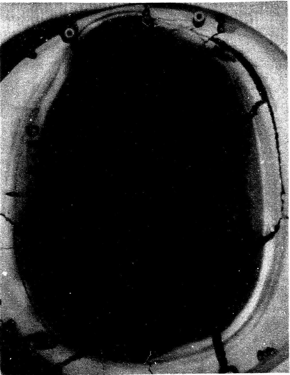
Figure 4.2.11. PIE photo showing final state of the DF-4 test bundle at the 95 mm axial level [5].
